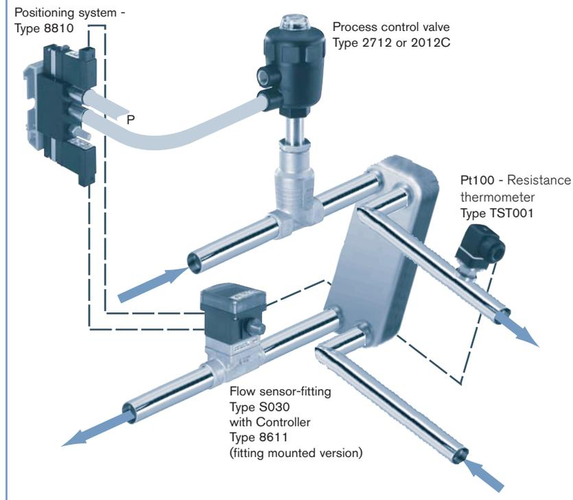
Flow control with process control valve
