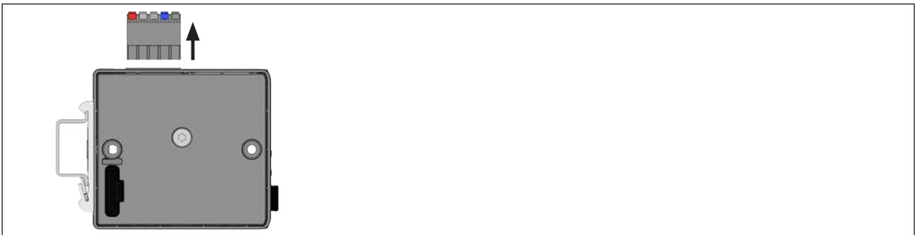
Figure 25: Remove 5-pin spring-type terminal
