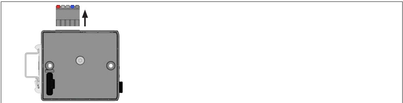
Figure 29: Remove 5-pin spring-type terminal
