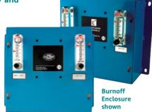
Reference air of approximately 20% oxygen must be supplied for the carbon probe to perform properly. The reference air enclosure is equipped with a single flowmeter and output. The burnoff enclosure is equipped with reference air and burnoff air flowmeters and outputs. An atmosphere controller with an event output can trigger the probe burnoff.
