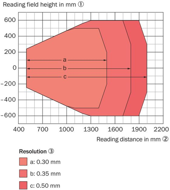
Figure 107: CLV690-1xxx (Standard Density): reading field height depending on the reading distance and resolution
