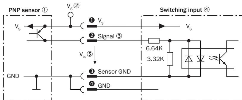
Figure 61: Wiring of a switching input with external PNP sensor
