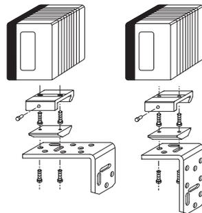
Figure 12: Example of mounting a CLV69x with a quick clamping device and a mounting bracket
