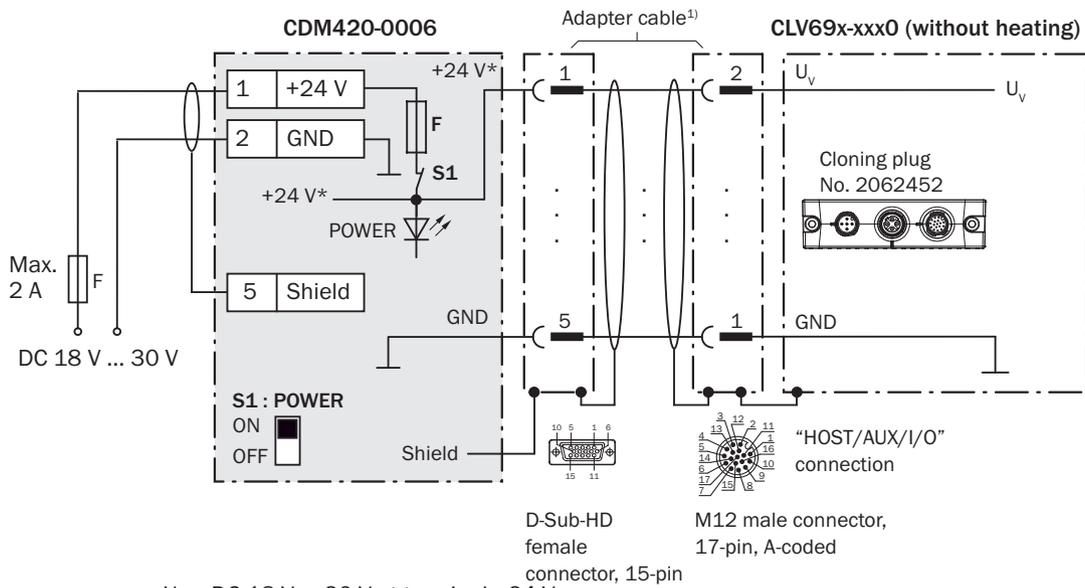
$U_v = \text{DC } 18 \text{ V} \dots 30 \text{ V}$  at terminal +24 V =
