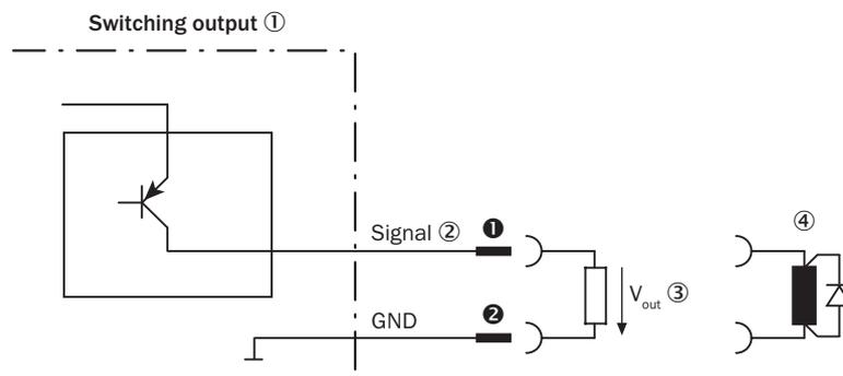
Figure 62: Wiring of a switching output
