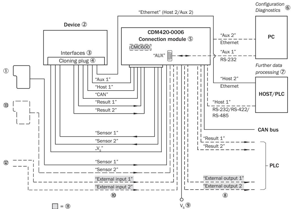
Figure 58: Connection of the device to the CDM420-0006 connection module
