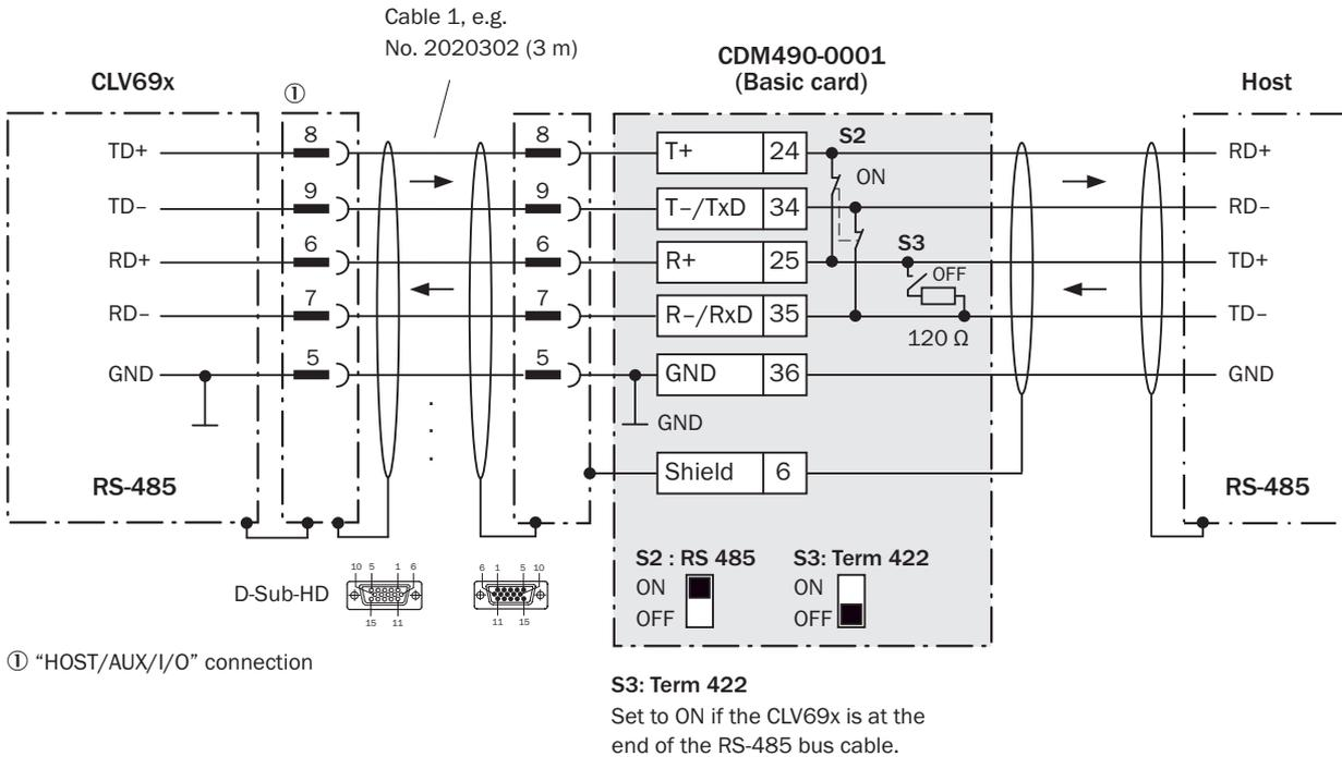
Figure 93: Wire serial host interface RS-485
