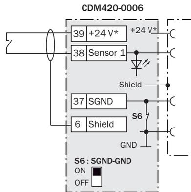
d) Switch connected volt-free and externally supplied
