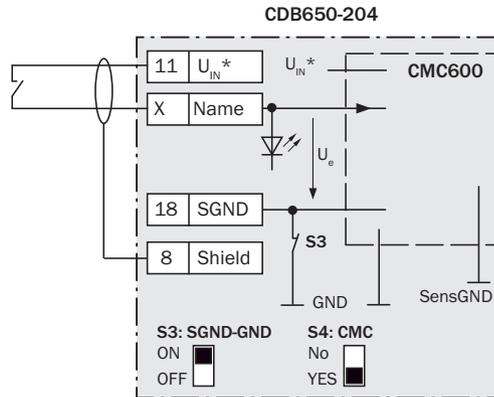
d) Switch connected volt-free and supplied externally
