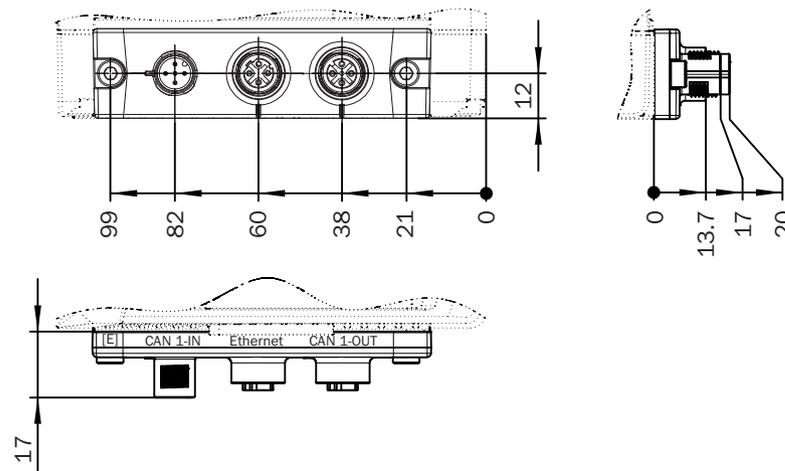
Figure 51: Dimensions of cloning plug E (M12), all dimensions in mm
