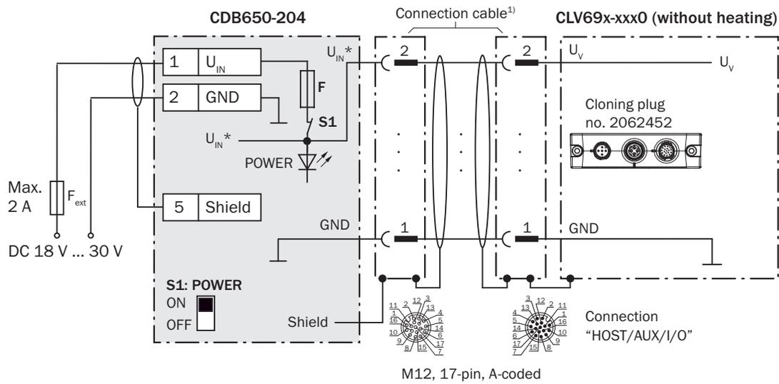
$U_V = \text{DC } 18 \text{ V} \dots 30 \text{ V}$  at terminal  $U_{IN}$  =
