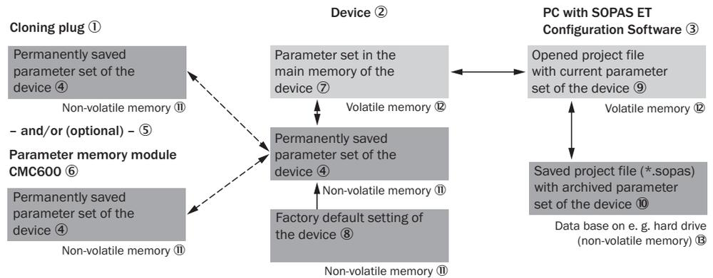
Figure 97: Configuration with SOPAS ET and saving the parameter set
