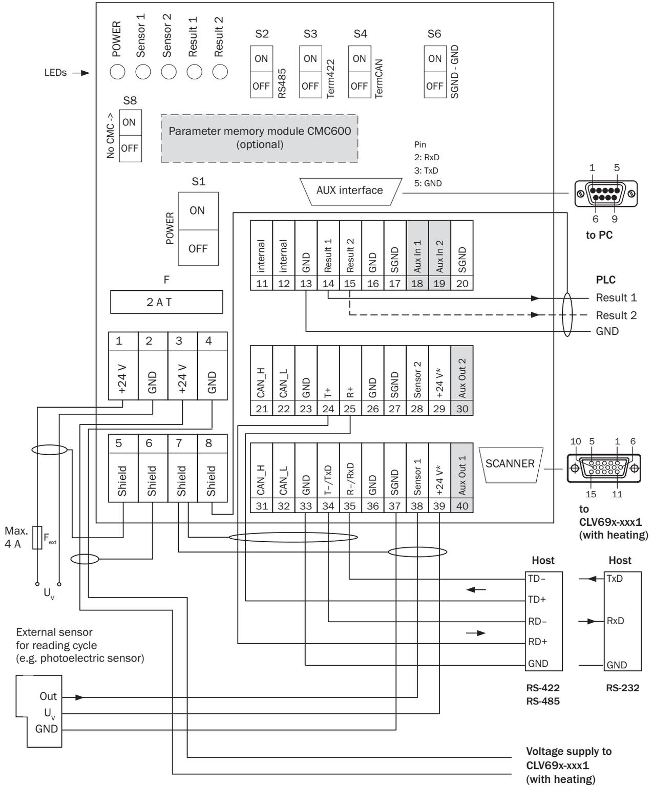
$U_v$  = DC 21.6 V ... 28.8 V for CLV69x-xxx1 (with heating), protected by external fuse provided by user
