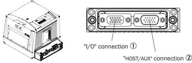
Figure 27: View of cloning plug A (D-Sub), part no. 2062450
