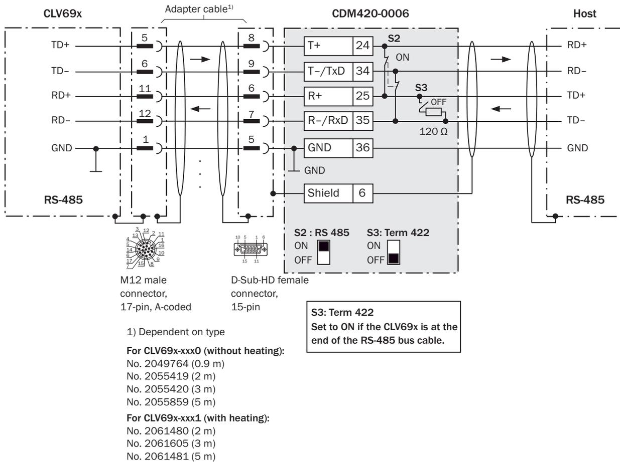
Figure 81: Wire serial host interface RS-485
