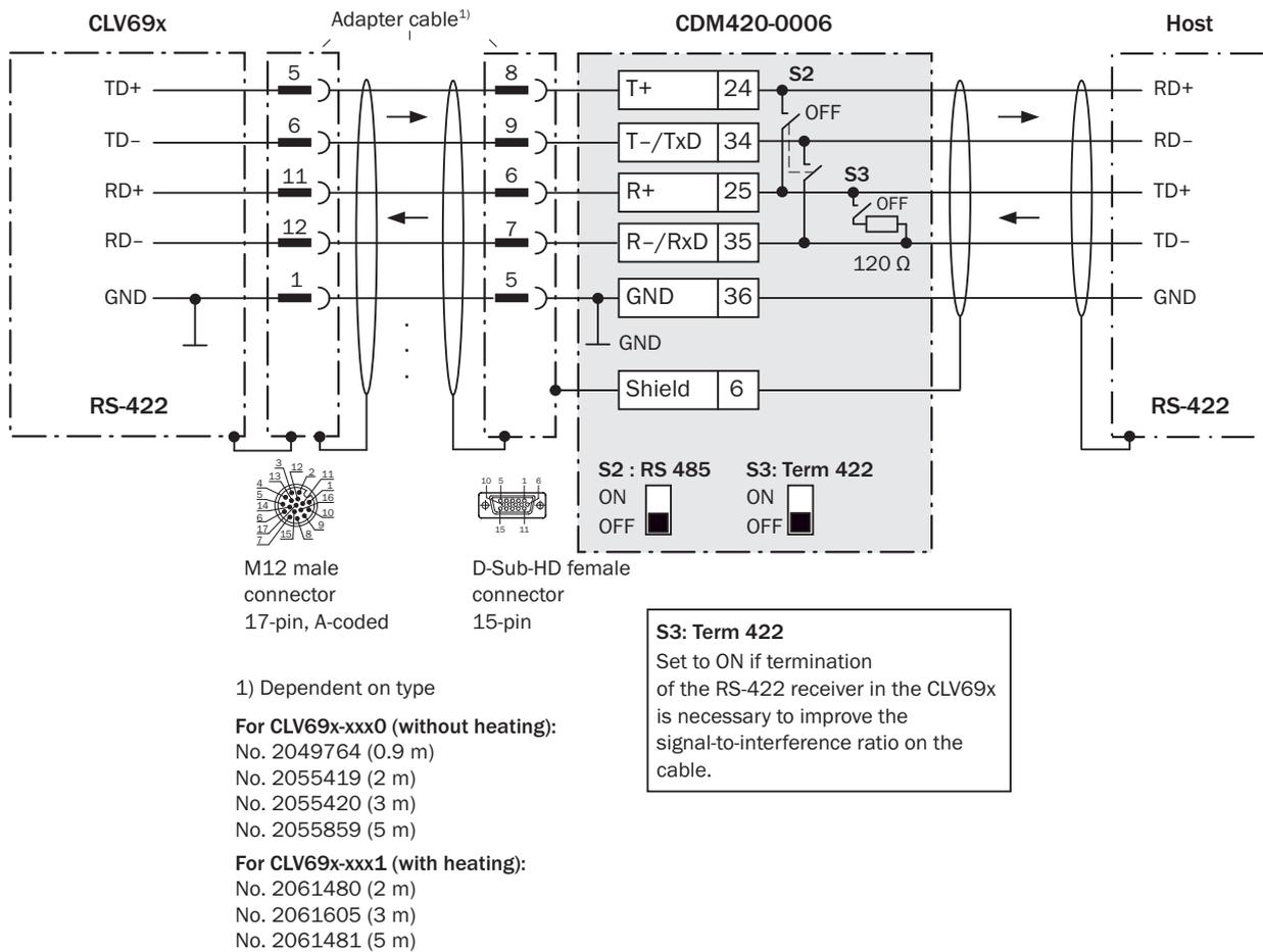
Figure 80: Wire serial host interface RS-422
