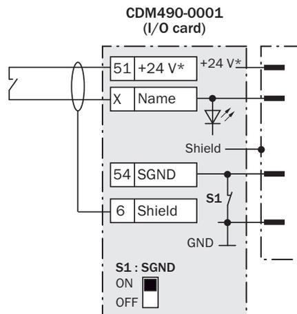
d) Schema: switch connected volt-free and externally supplied
