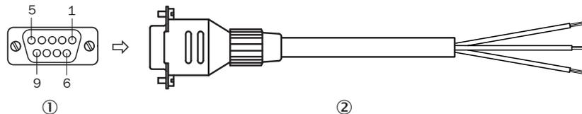
Figure 135: Adapter cable, part no. 2020319 (3 m)
