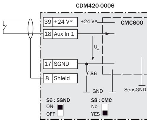
d) Switch connected volt-free and externally supplied
