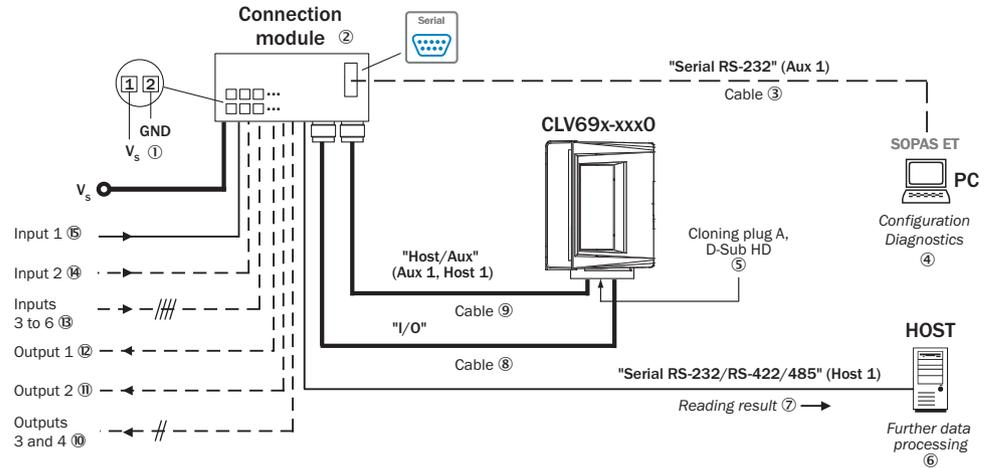
Figure 6: Facilities for connecting for devices without/with integrated heating to connection module CDM490-0001 when replacing a predecessor CLV49x
