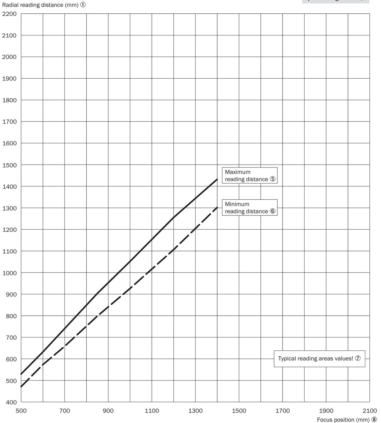
Figure 127: CLV692-1xxx (High Density): min. and max. radial reading distance depending on the focus position at a resolution of 0.25 mm and aperture angle of  $\alpha = 40^\circ$
