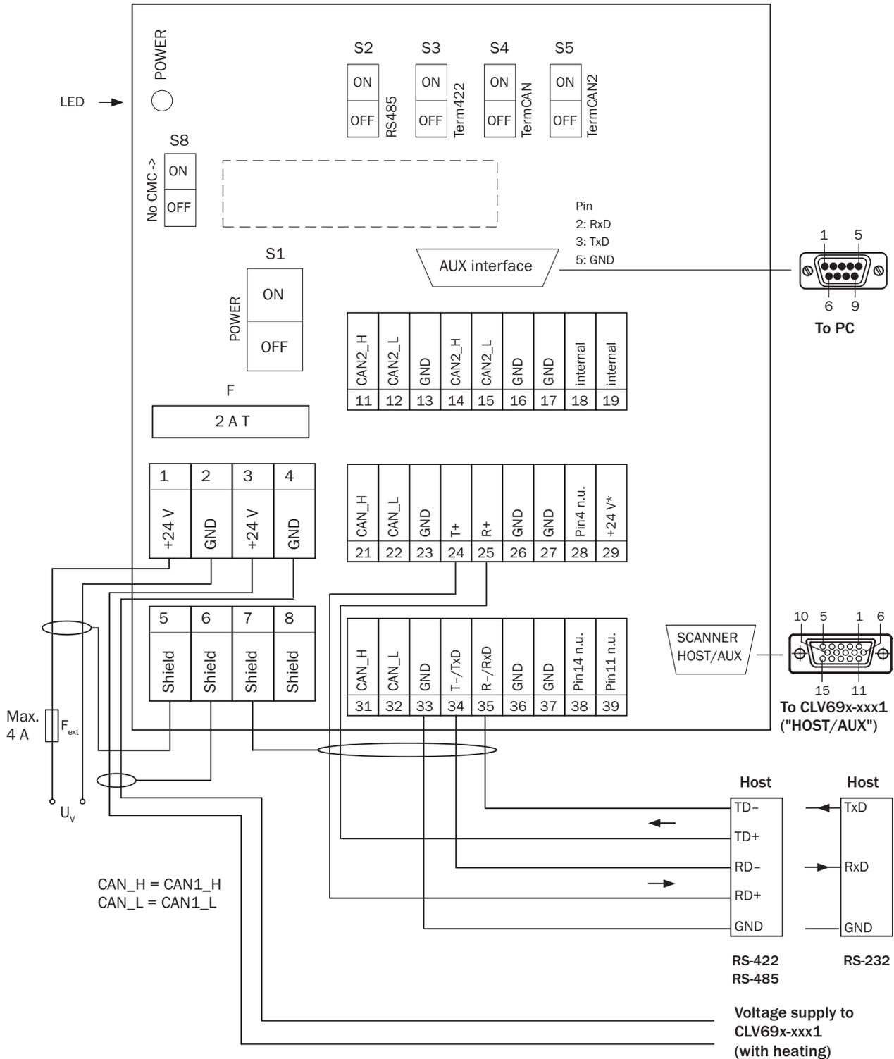
U<sub>v</sub> = DC 21.6 V ... 28.8 V for CLV69x-xxx1 (with heating), protected by external fuse provided by user
