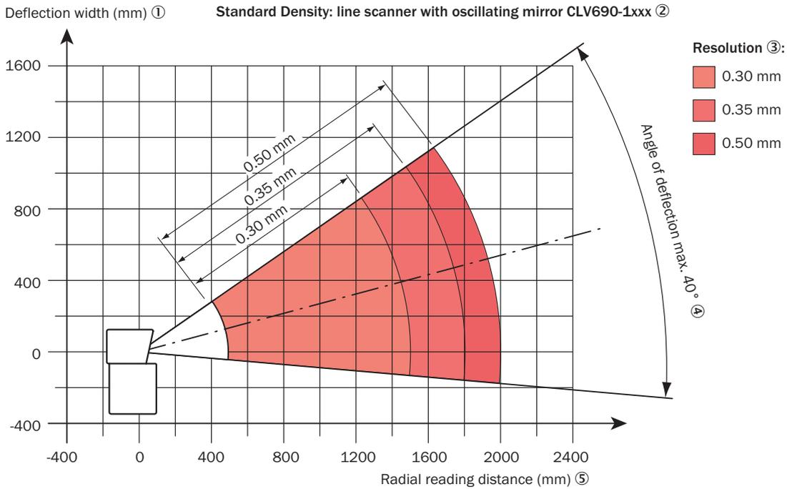
Figure 113: CLV690-1xxx (Standard Density): deflection width depending on the radial reading distance, angle of deflection and resolution
