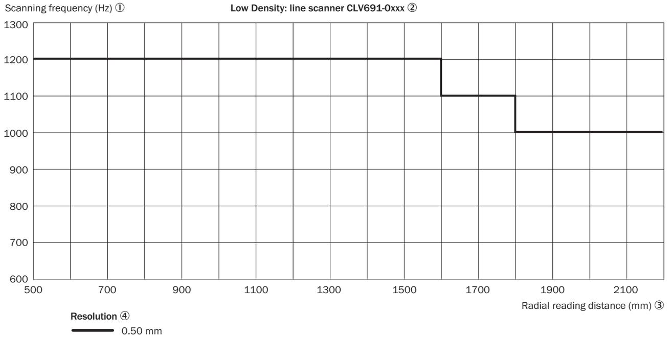
Figure 117: CLV691-0xxx (Low Density): characteristic curve field scanning frequency depending on the radial reading distance and resolution
