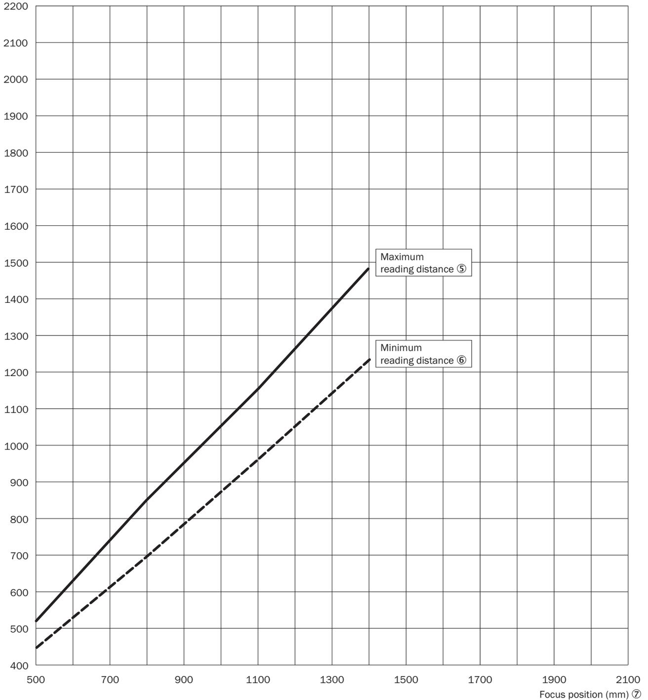
Figure 111: CLV690-1xxx (Standard Density): min. and max. radial reading distance depending on the focus position at a resolution of 0.50 mm and aperture angle of  $\alpha = 50^\circ$
