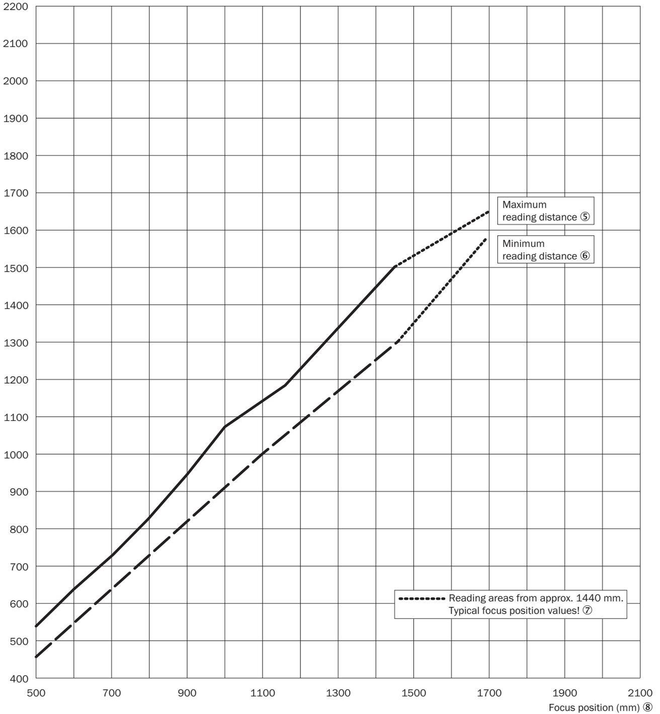
Figure 128: CLV692-1xxx (High Density): min. and max. radial reading distance depending on the focus position at a resolution of 0.35 mm and aperture angle of  $\alpha = 40^\circ$
