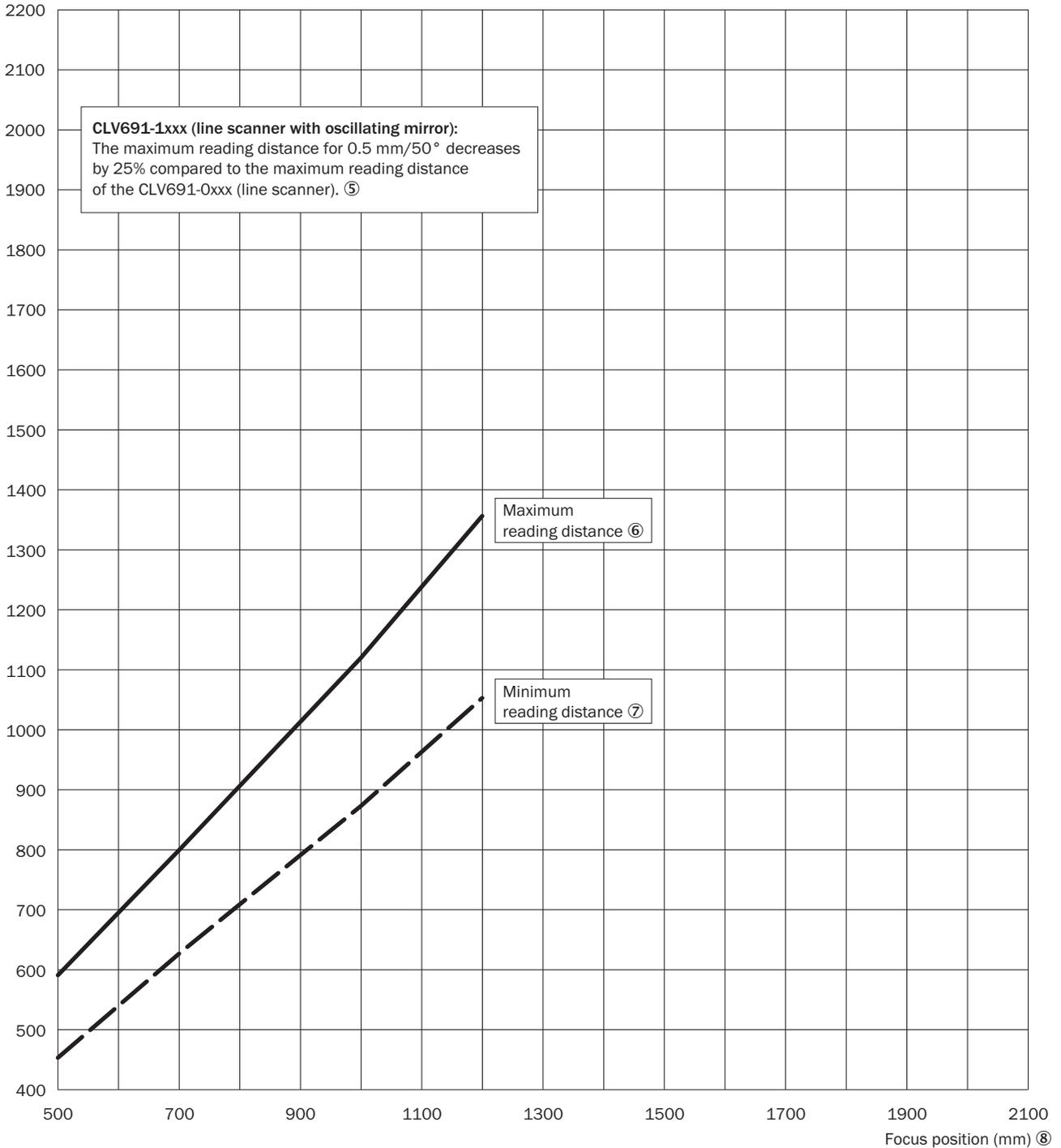
Figure 116: CLV691-0xxx (Low Density): min. and max. radial reading distance depending on the focus position at a resolution of 0.5 mm and aperture angle of  $\alpha = 60^\circ$
