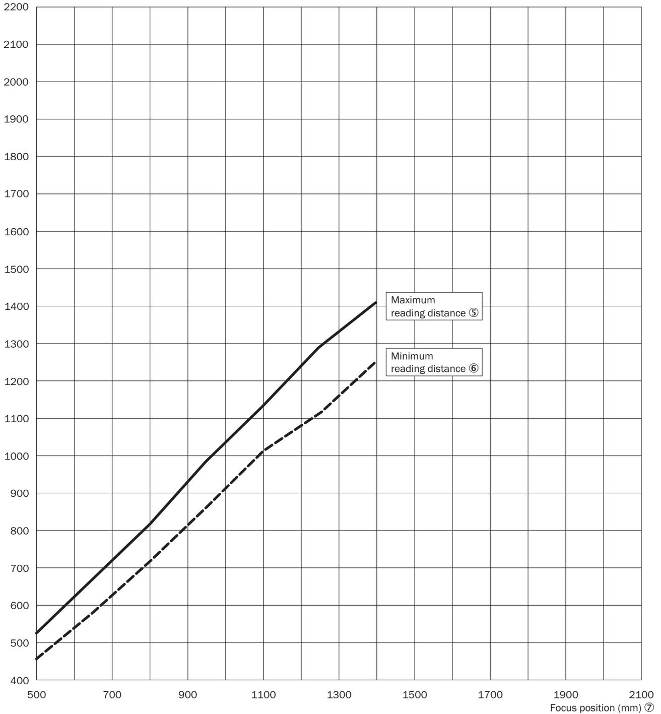
Figure 129: CLV692-1xxx (High Density): min. and max. radial reading distance depending on the focus position at a resolution of 0.35 mm and aperture angle of  $\alpha = 50^\circ$
