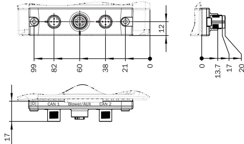
Figure 46: Dimensions of cloning plug D (M12), all dimensions in mm
