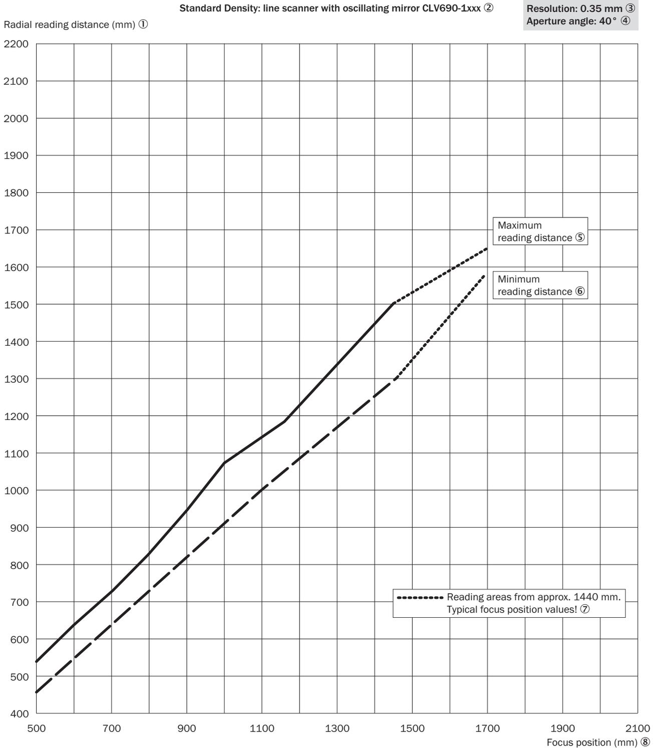
Figure 108: CLV690-1xxx (Standard Density): min. and max. radial reading distance depending on the focus position at a resolution of 0.35 mm and aperture angle of  $\alpha = 40^\circ$
