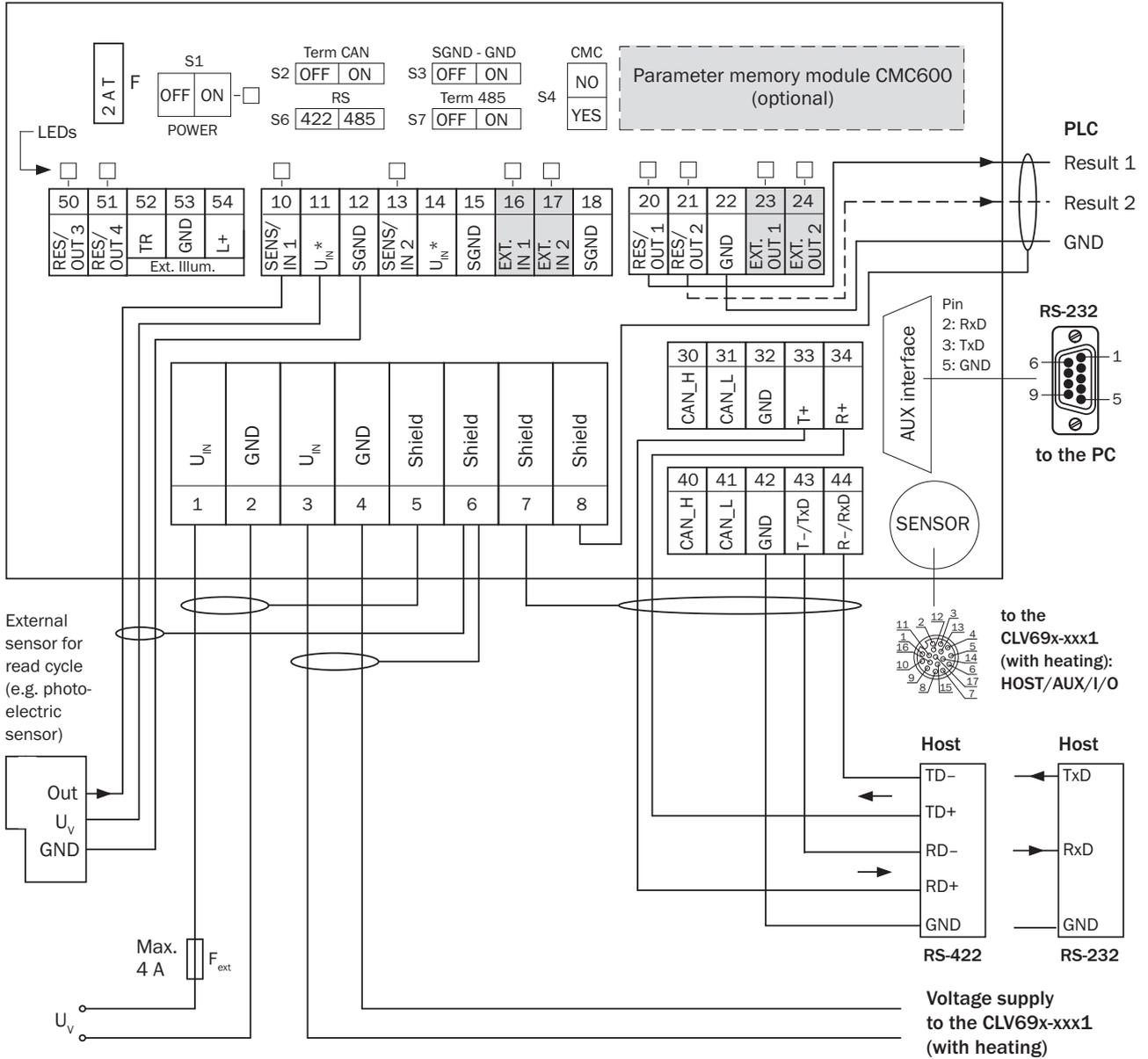
U<sub>v</sub> = DC 21.6 V ... 28.8 V for CLV69x-xxx1 (with heating), protected by external fuse provided by user
