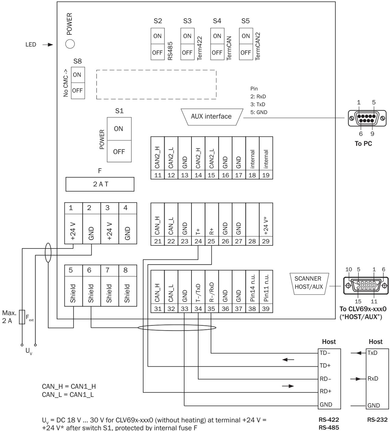
Figure 87: Wiring overview, part 1 (basic map below left), for CLV69x-xxx0 (without heating)
