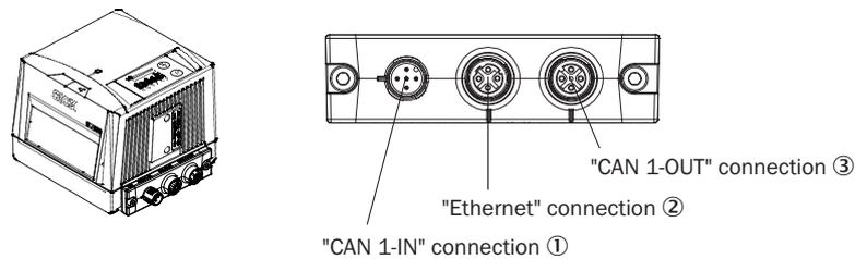
Figure 47: View of cloning plug E (M12), part no. 2074708
