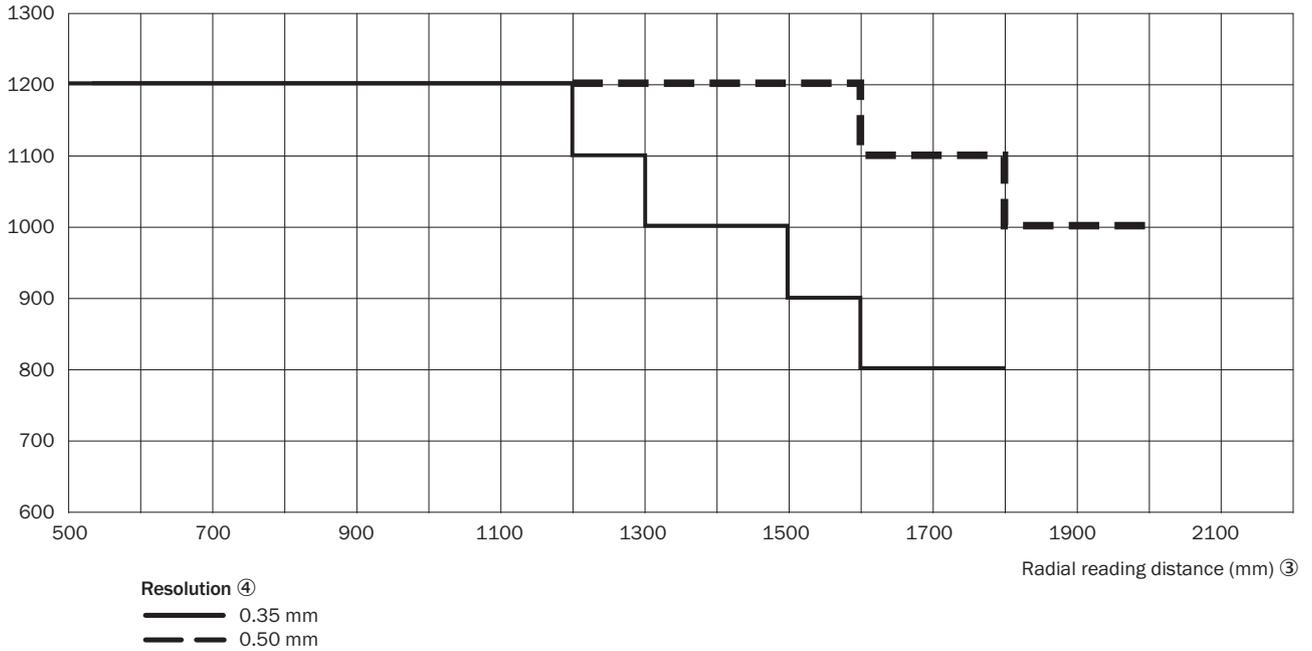
Figure 1.12: CLV690-1xxx (Standard Density): characteristic curve field scanning frequency depending on the radial reading distance and resolution
