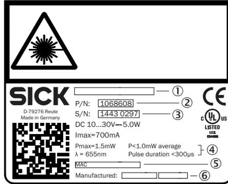
Figure 3: Type label design for the device, illustration may differ from actual type label
