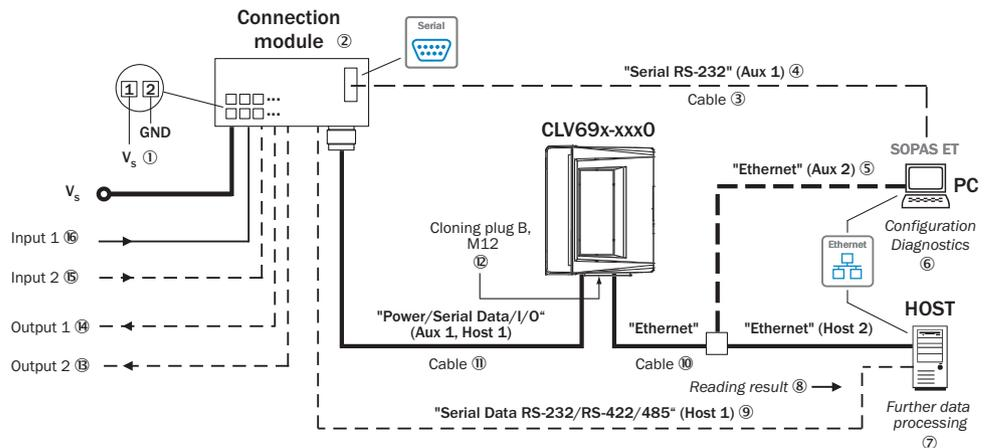
Figure 5: Facilities for connecting for devices without/with heating to connection module CDB650-204 or CDM420-0006
