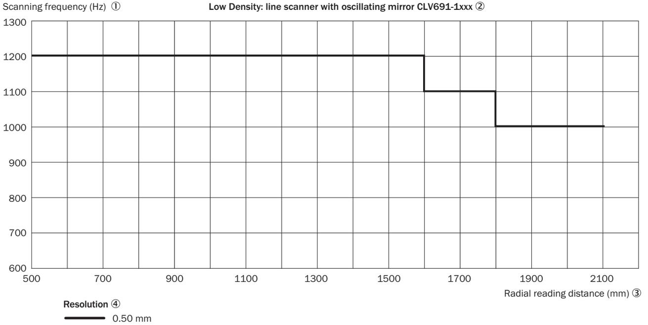
Figure 119: CLV691-1xxx (Low Density): characteristic curve field scanning frequency depending on the radial reading distance and resolution
