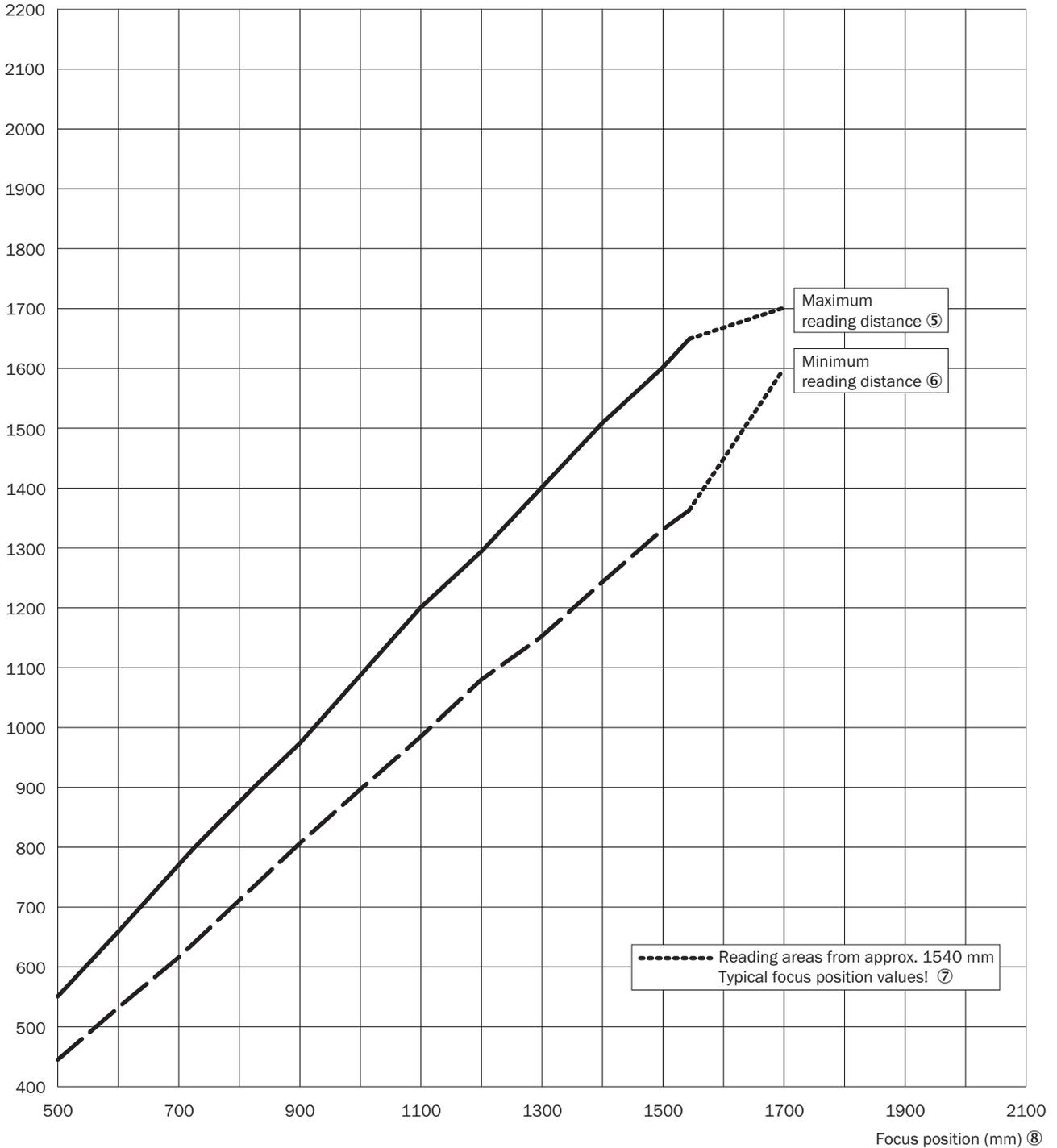
Figure 123: CLV692-0xxx (High Density): min. and max. radial reading distance depending on the focus position at a resolution of 0.35 mm and aperture angle of  $\alpha = 40^\circ$
