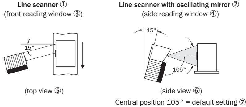
Figure 15: Avoiding surface reflections: Angle between light emitted and bar code (tilting away from vertical)
