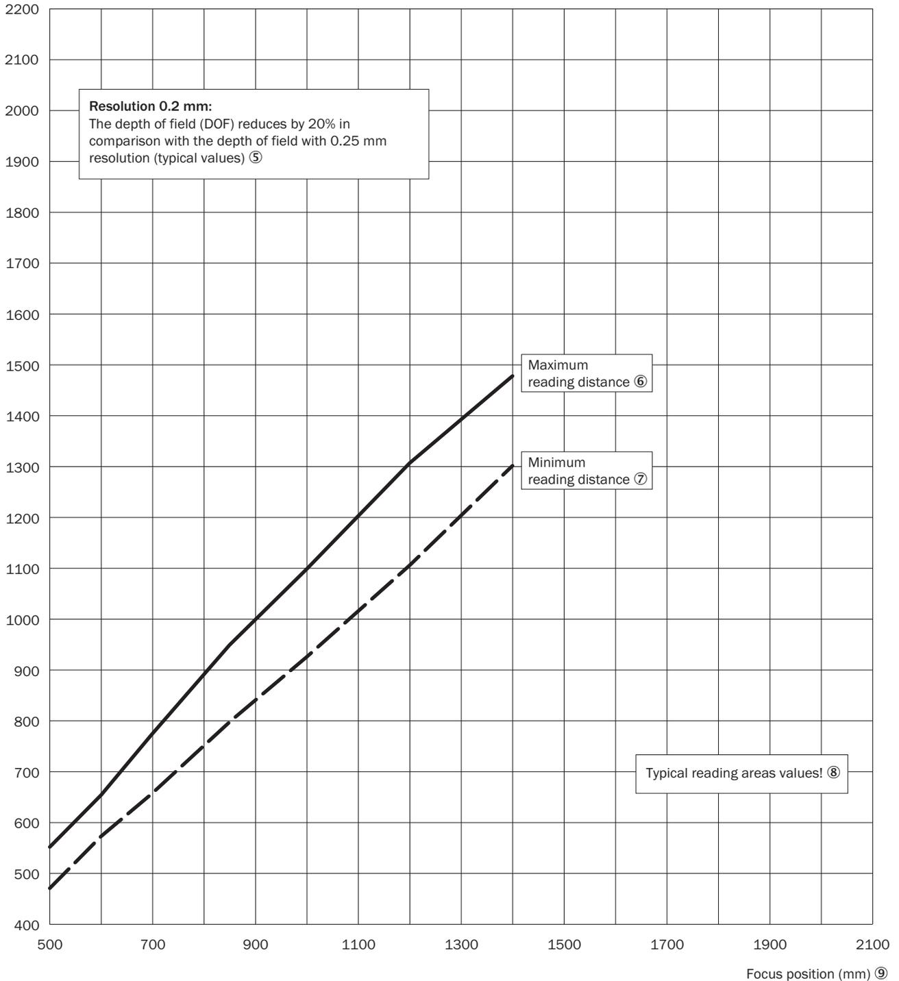
Figure 122: CLV692-0xxx (High Density): min. and max. radial reading distance depending on the focus position at a resolution of 0.25 mm and aperture angle of  $\alpha = 40^\circ$
