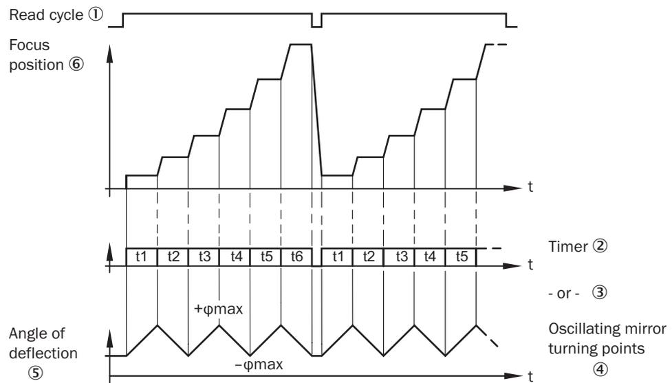
Figure 9: Oscillating mirror - example for focus position control during the search run, here with 6 focus positions
