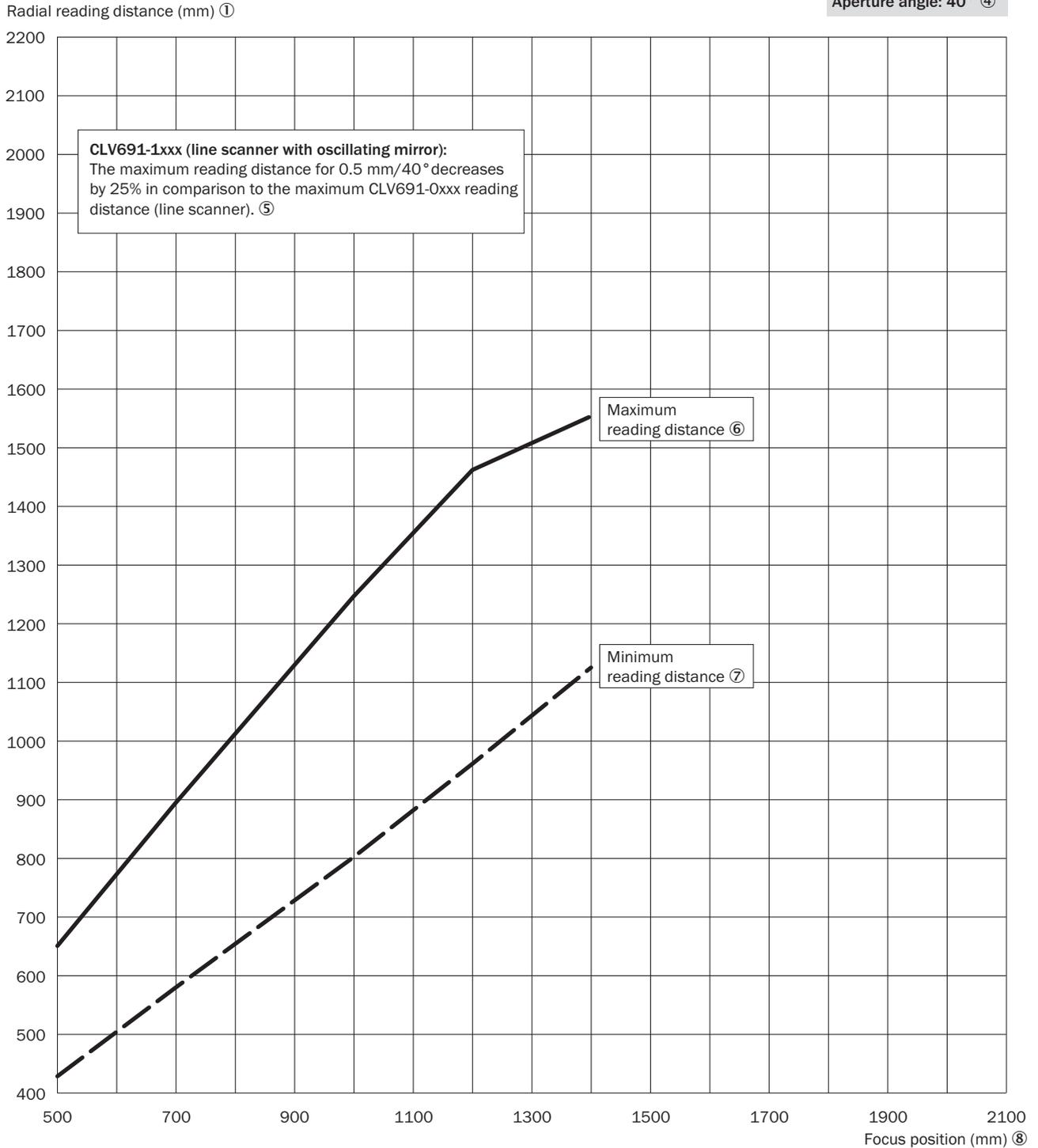
Figure 115: CLV691-0xxx (Low Density): min. and max. radial reading distance depending on the focus position at a resolution of 0.5 mm and aperture angle of  $\alpha = 40^\circ$
