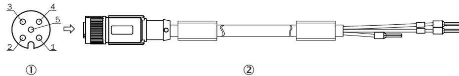
Figure 136: Adapter cable, e.g., part no. 6053224 (5 m)
