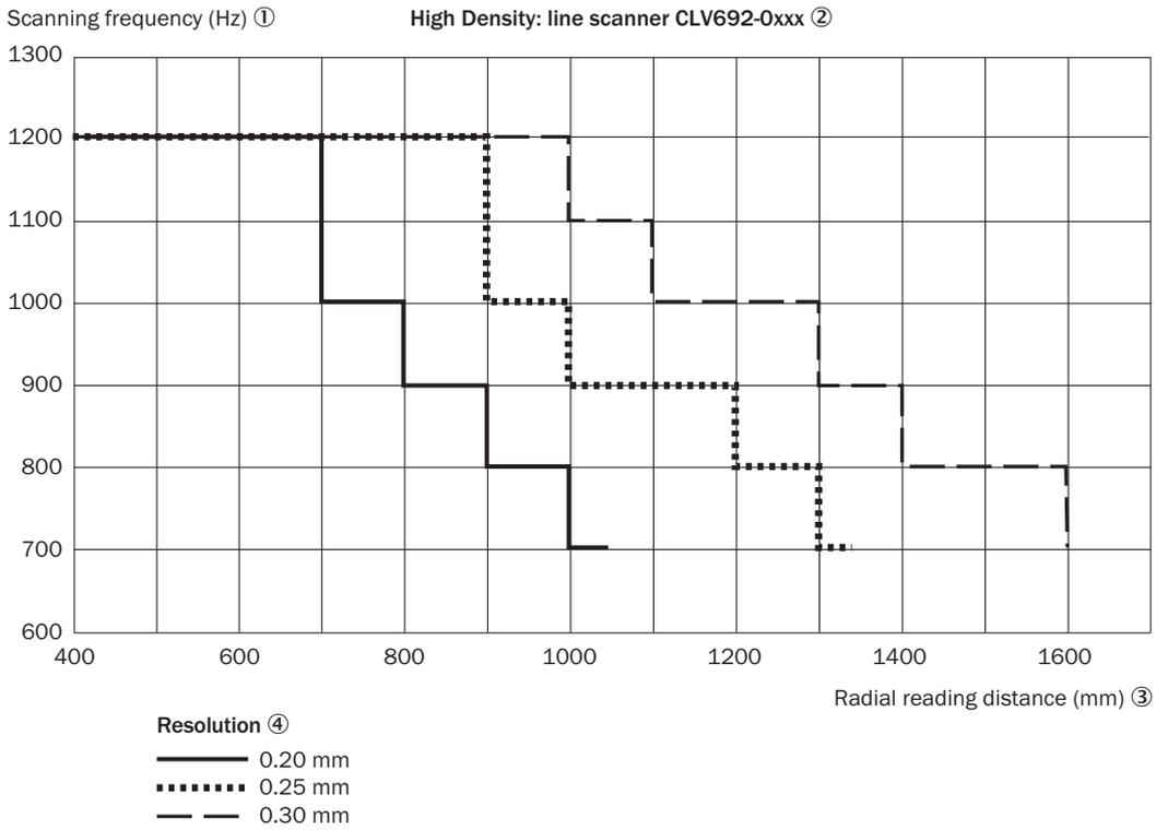
Figure 125: CLV692-0xxx (High Density): characteristic curve field scanning frequency depending on the radial reading distance and resolution
