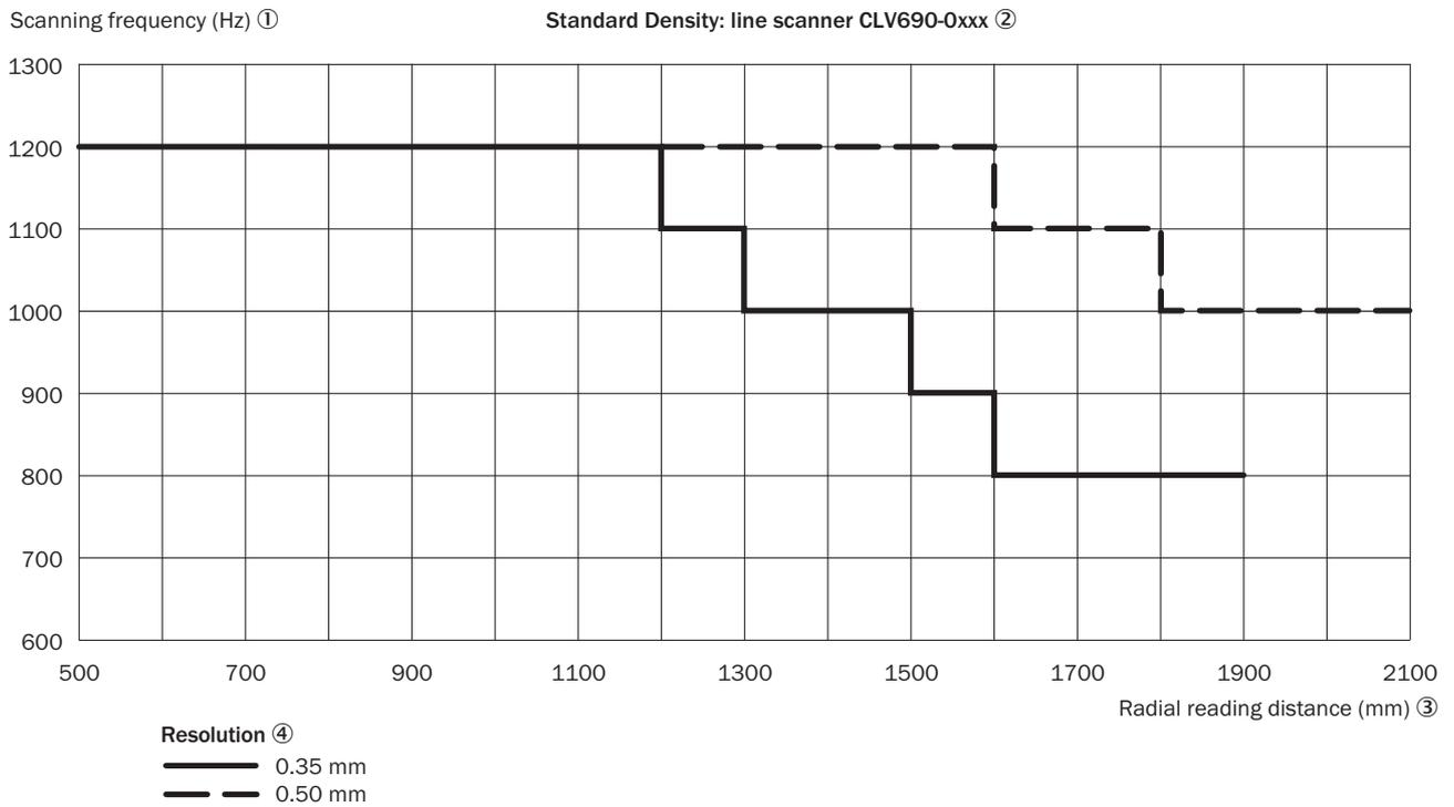
Figure 106: CLV690-0xxx (Standard Density): characteristic curve field scanning frequency depending on the radial reading distance and resolution
