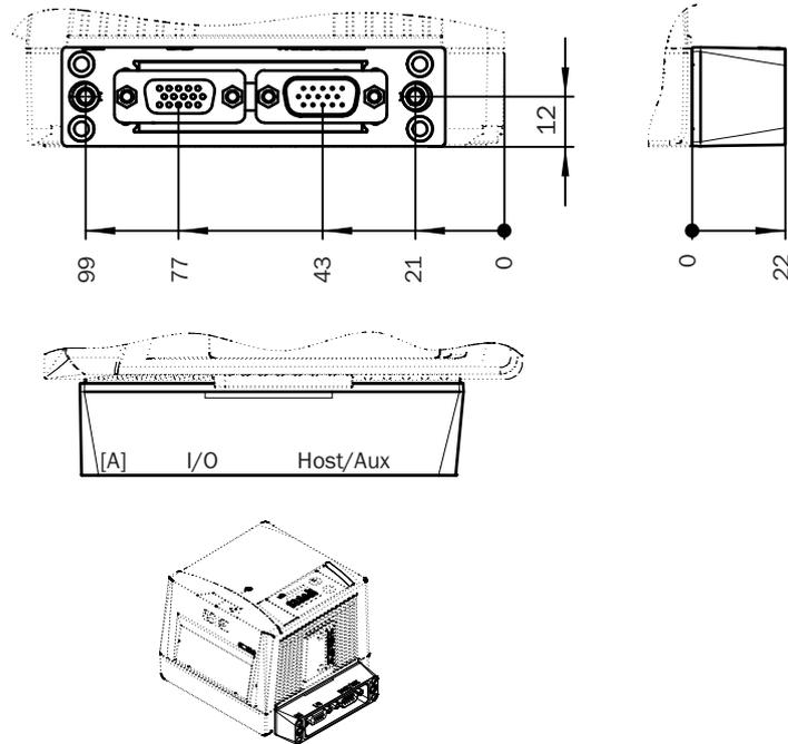
Figure 30: Dimensions of cloning plug A (D-Sub), all dimensions in mm
