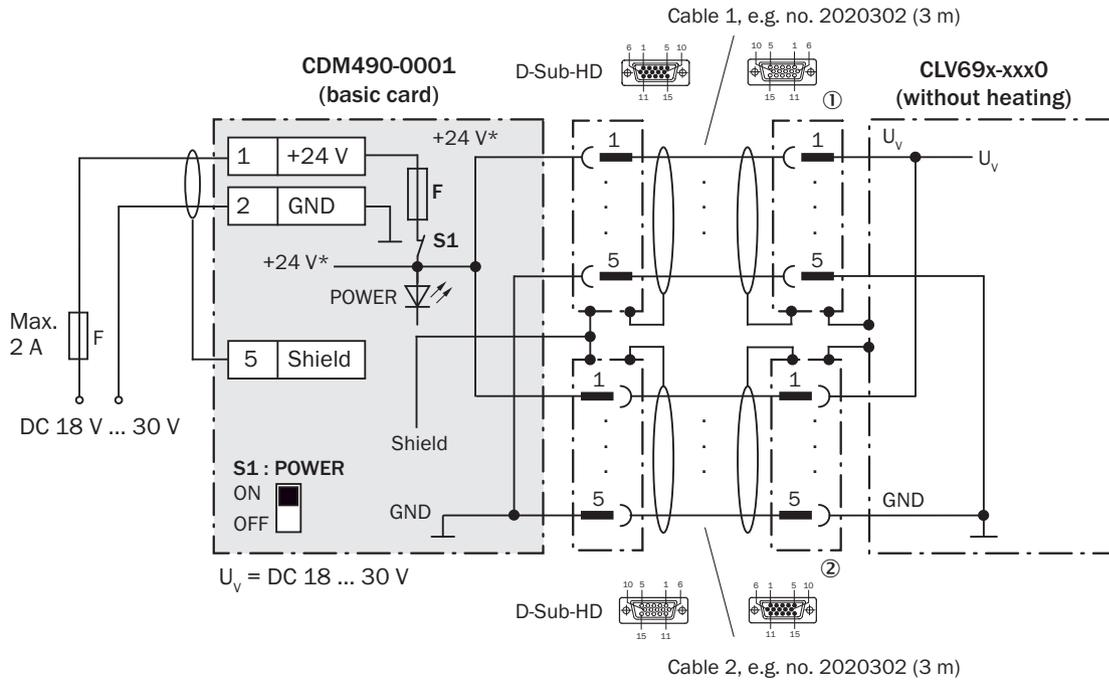
+) If no switching inputs and outputs of the CLV69x are used, cable 2 does not have to be used
