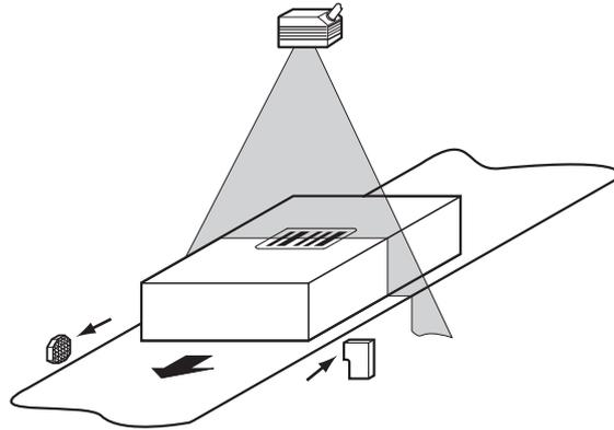
Figure 100: Cleaning the external optical sensors (read pulse encoder)
