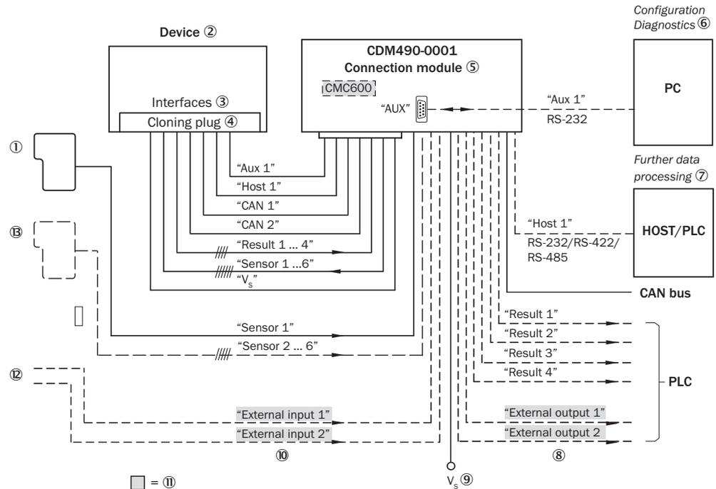
Figure 59: Connection of the device to the CDM490-0001 connection module
