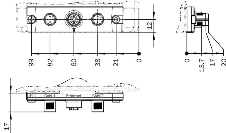
Figure 56: Dimensions of cloning plug F (M12), all dimensions in mm
