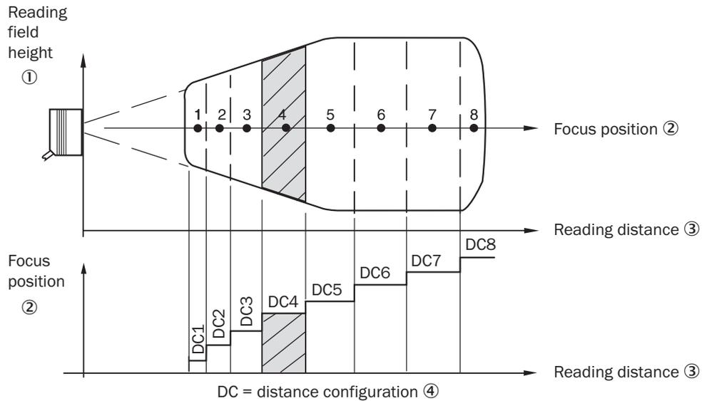
Figure 8: Focus switching - dividing the total read area into distance configurations
