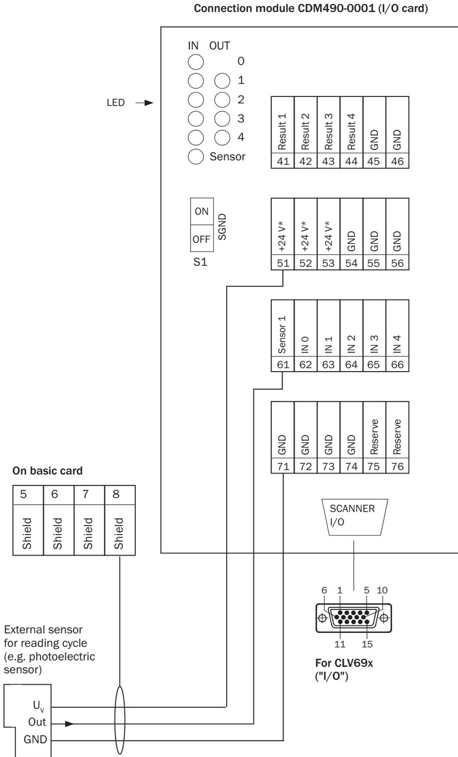
Figure 89: Wiring overview, part 2 (I/O map top right), 1 switching input used
