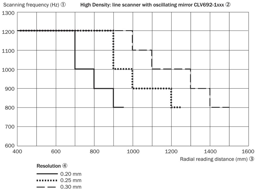
Figure 130: CLV692-1xxx (High Density): characteristic curve field scanning frequency depending on the radial reading distance and resolution
