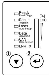
Figure 99: LED status indicator, bar graph and function keys
