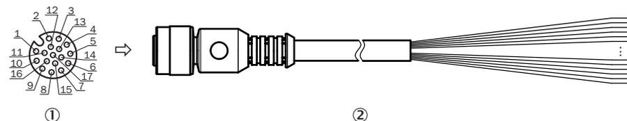
Figure 134: Adapter cable, e.g. part no. 2081094 (2 m)
