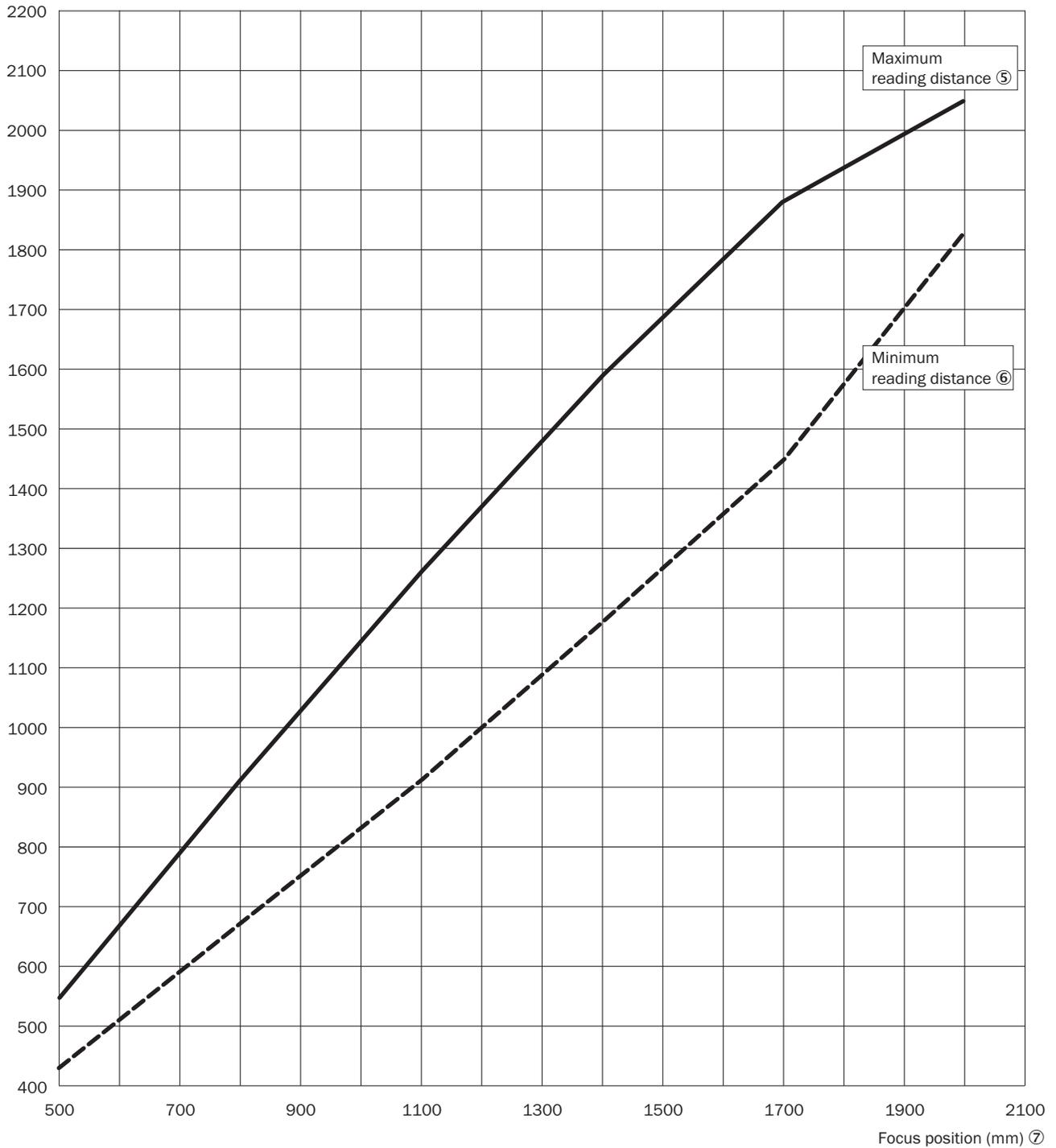
Figure 104: CLV690-0xxx (Standard Density): min. and max. radial reading distance depending on the focus position at a resolution of 0.50 mm and aperture angle of  $\alpha = 40^\circ$
