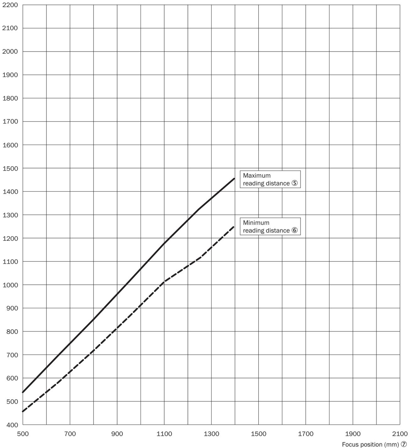
Figure 124: CLV692-0xxx (High Density): min. and max. radial reading distance depending on the focus position at a resolution of 0.35 mm and aperture angle of  $\alpha = 56^\circ$
