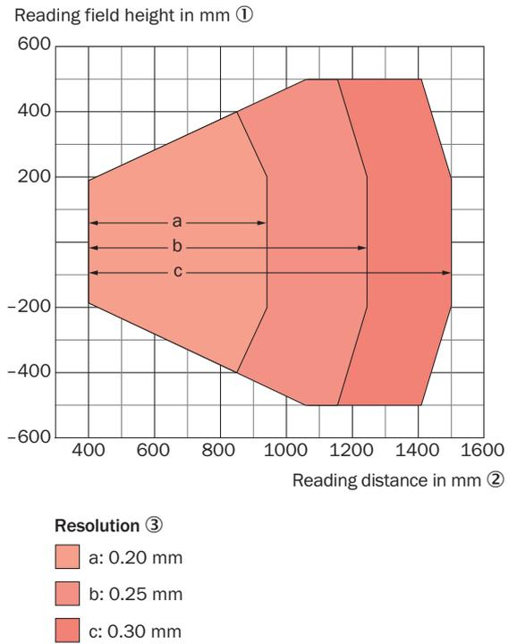
Figure 126: CLV692-1xxx (High Density): reading field height depending on the reading distance and resolution
