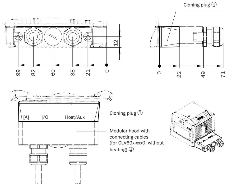
Figure 31: Dimensions of cloning plug A (D-Sub), with the hood of a connecting cable. All dimensions in mm.
