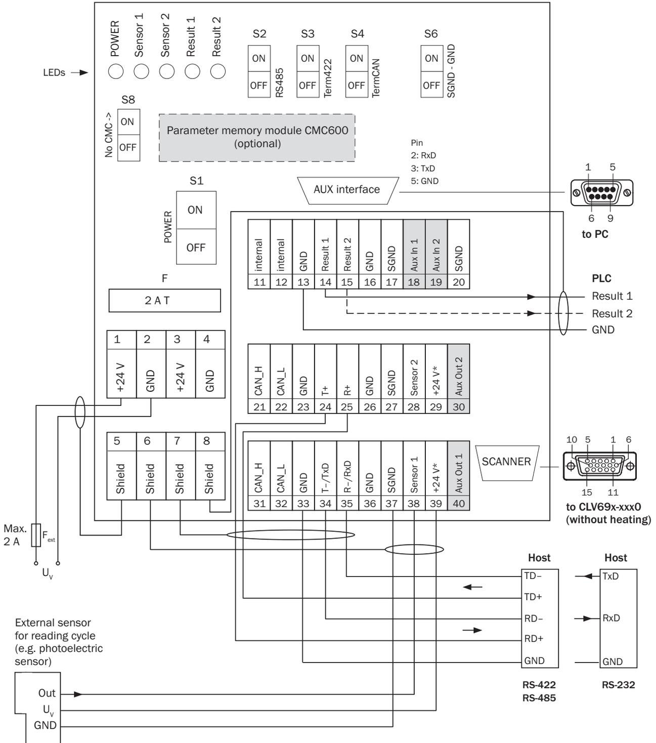
$U_V = DC 18 V \dots 30 V$  for CLV69x-xxx0 (without heating) at terminal +24 V = +24 V\* after switch S1, protected by internal fuse F
