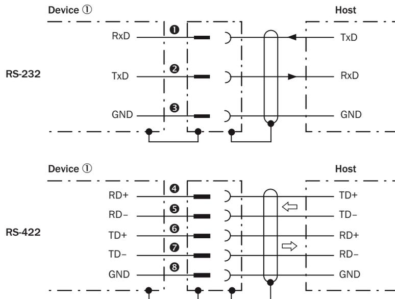
Figure 60: Internal circuitry for RS-232 and RS-485 data interfaces
