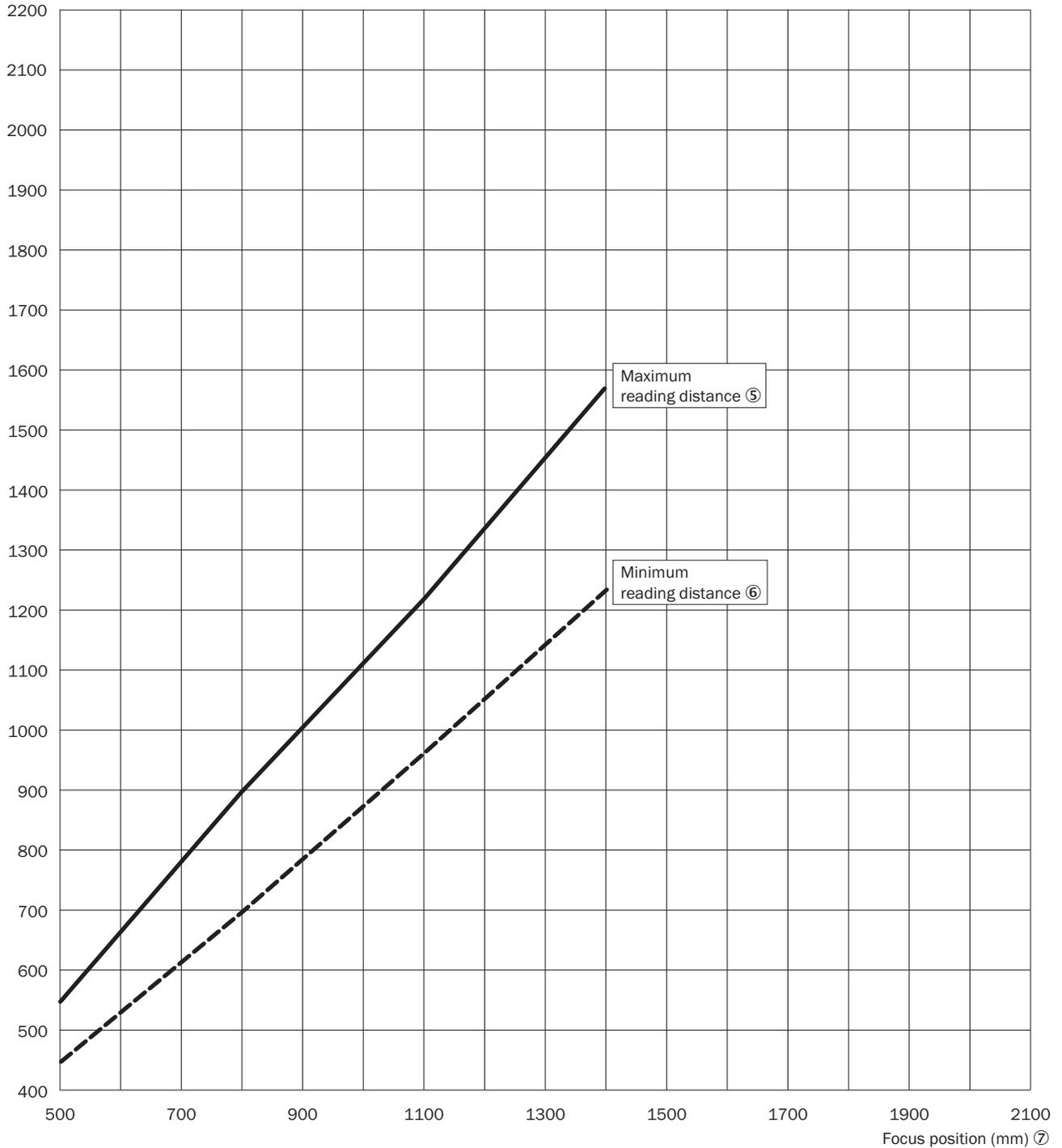
Figure 105: CLV690-0xxx (Standard Density): min. and max. radial reading distance depending on the focus position at a resolution of 0.50 mm and aperture angle of  $\alpha = 56^\circ$
