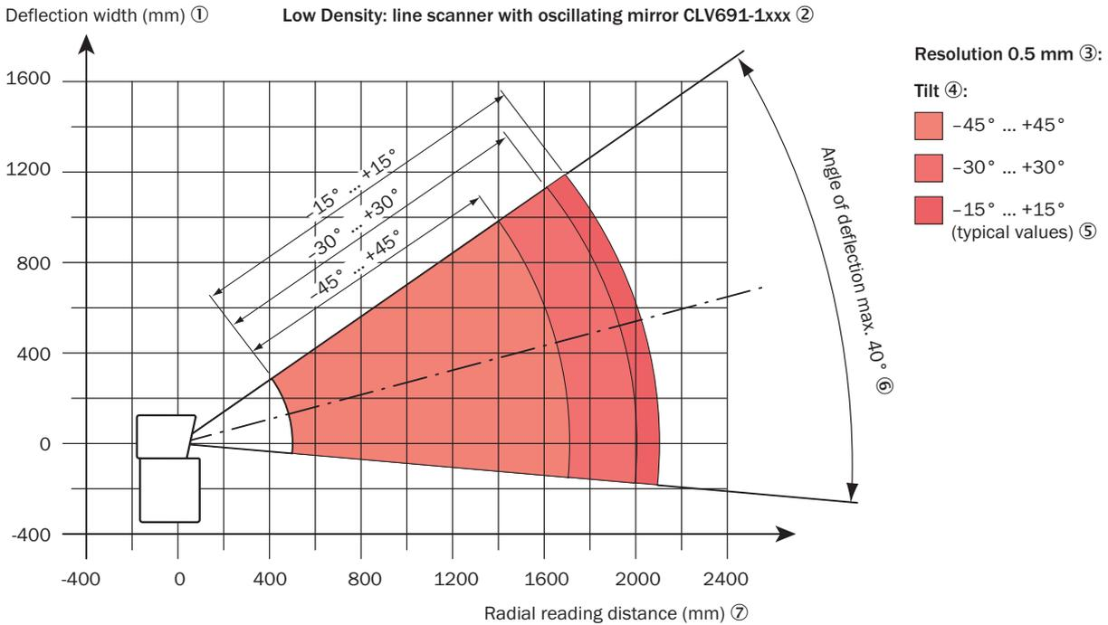
Figure 120: CLV691-1xxx (Low Density): deflection width depending on the reading distance, angle of deflection and tilt at a resolution of 0.5 mm
