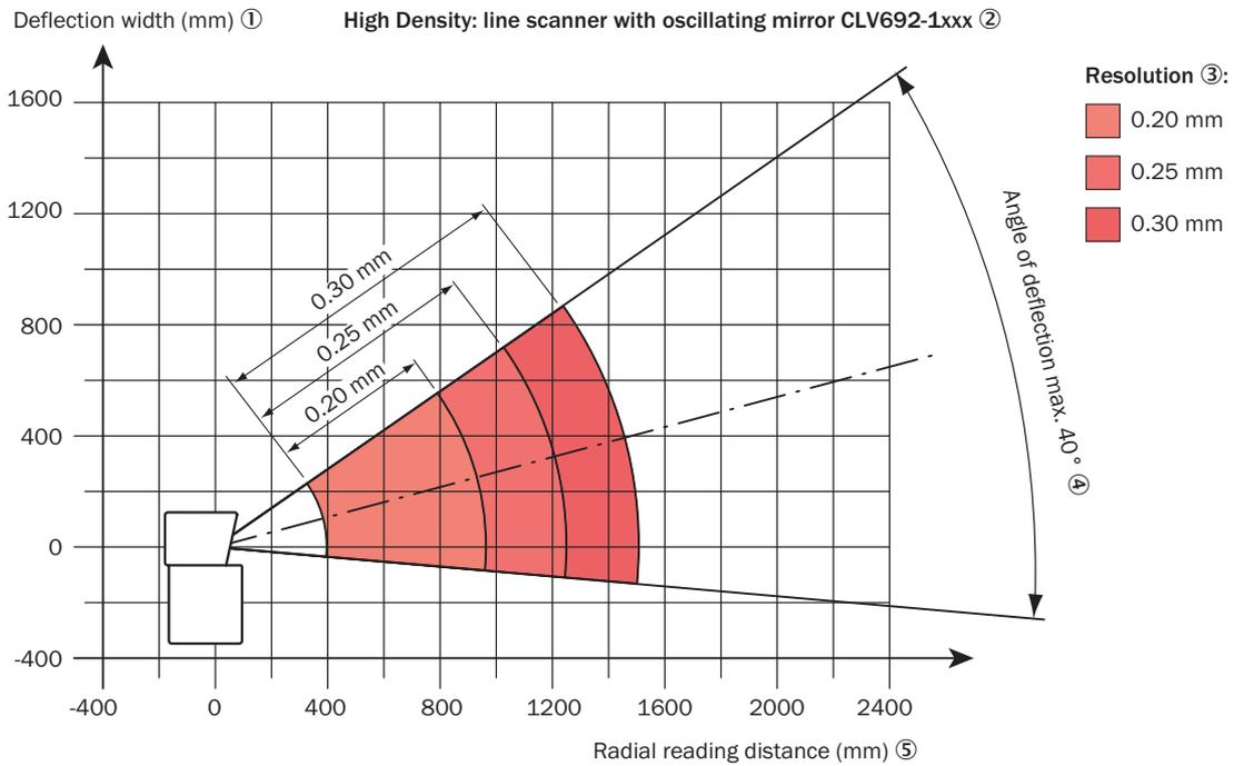
Figure 131: CLV692-1xxx (High Density): deflection width depending on the radial reading distance, angle of deflection and resolution
