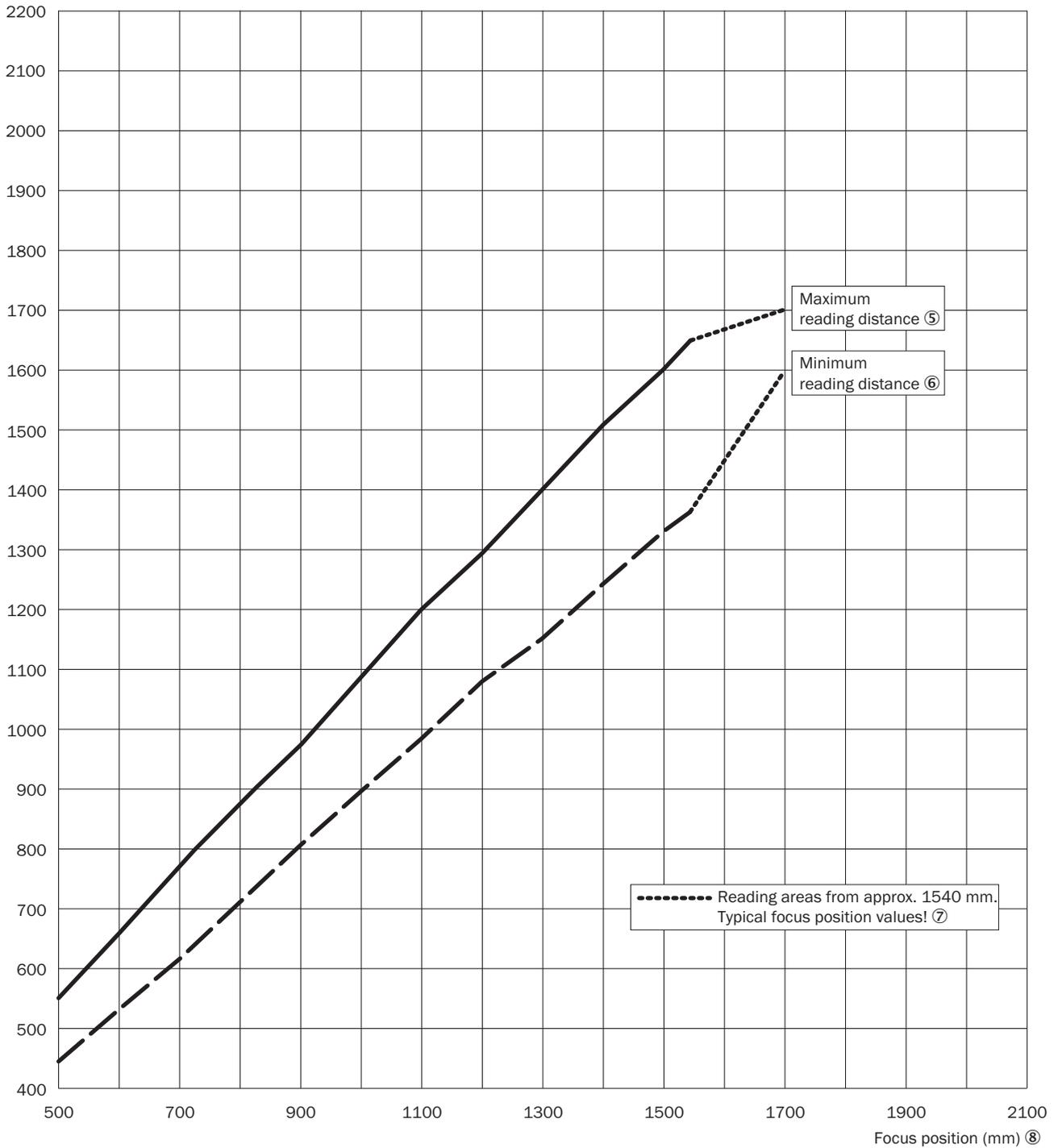
Figure 102: CLV690-0xxx (Standard Density): min. and max. radial reading distance depending on the focus position at a resolution of 0.35 mm and aperture angle of  $\alpha = 40^\circ$
