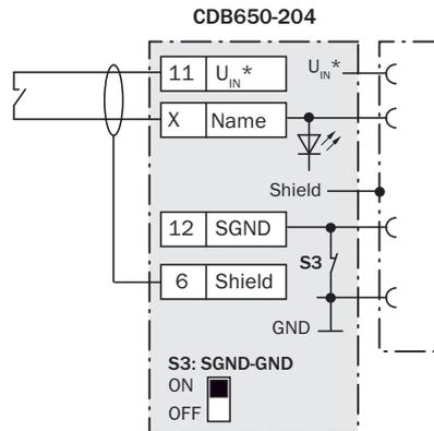
d) Diagram: switch connected volt-free and supplied externally
