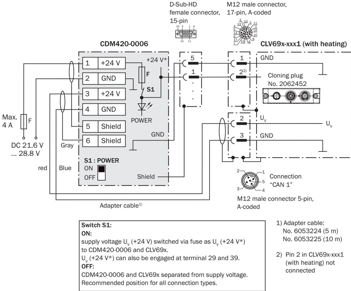
Figure 78: Wire supply voltage for CLV69x-xxx1 (with heating)
