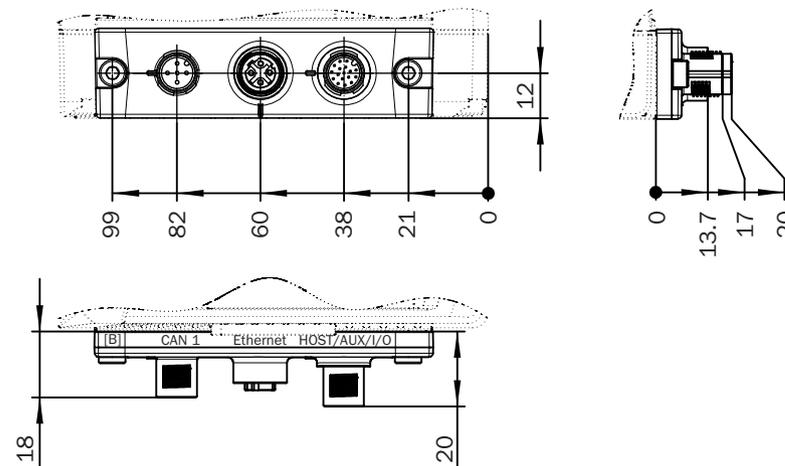
Figure 36: Dimensions of cloning plug B (M12), all dimensions in mm
