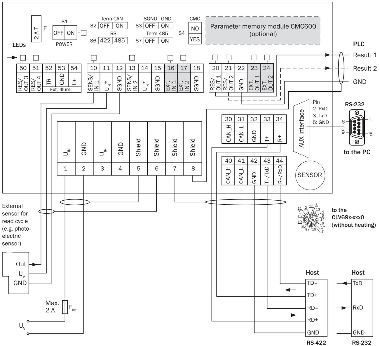
U<sub>V</sub> = DC 18 V ... 30 V for CLV69x-xxx0 (without heating) at terminal U<sub>IN</sub> = U<sub>IN</sub>\* after switch S1, protected with internal fuse F
