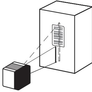
Figure 98: Appearance of the scan line in “Adjusting Mode”
