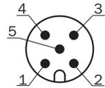
Figure 53: Male connector, M12, 5-pin, A-coded
