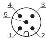
Figure 48: Male connector, M12, 5-pin, A-coded
