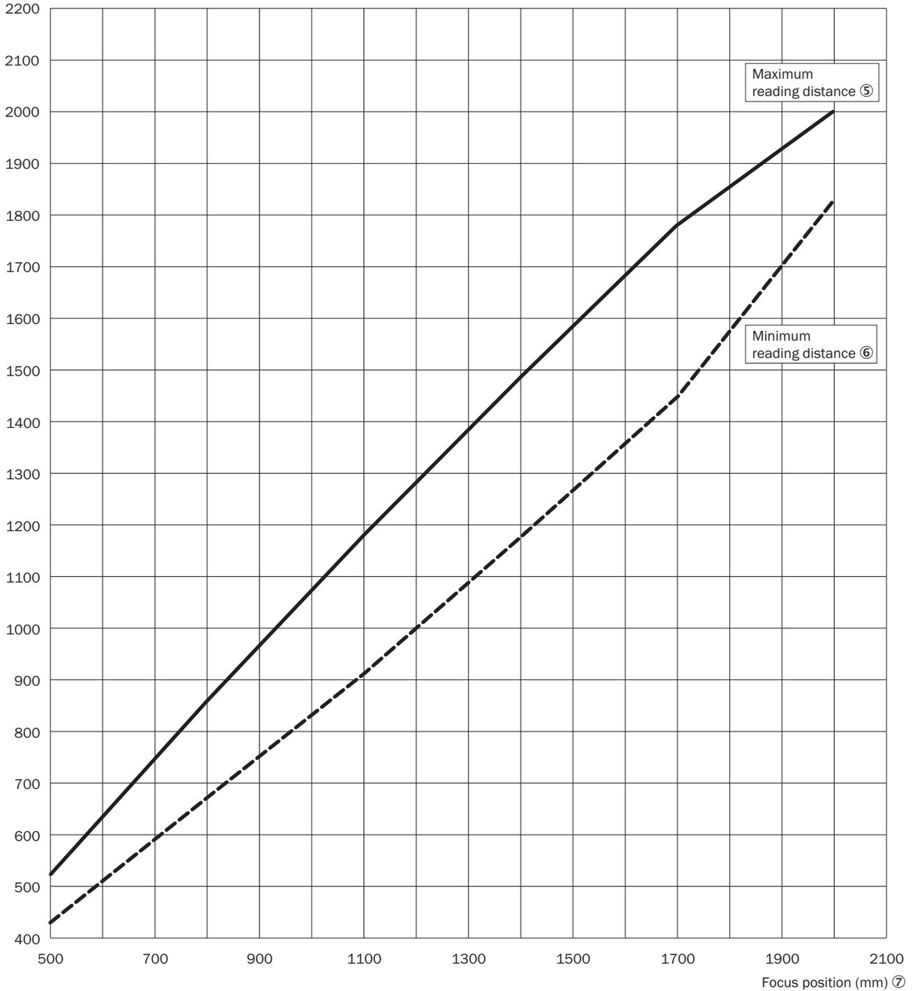
Figure 110: CLV690-1xxx (Standard Density): min. and max. radial reading distance depending on the focus position at a resolution of 0.50 mm and aperture angle of  $\alpha = 40^\circ$
