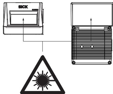
Figure 1: Laser output aperture in the different designs
