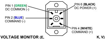
Use the following wiring diagram for QB valves with a voltage monitor output.
