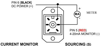
Use the following wiring diagram for QB valves with a current sourcing monitor output.
