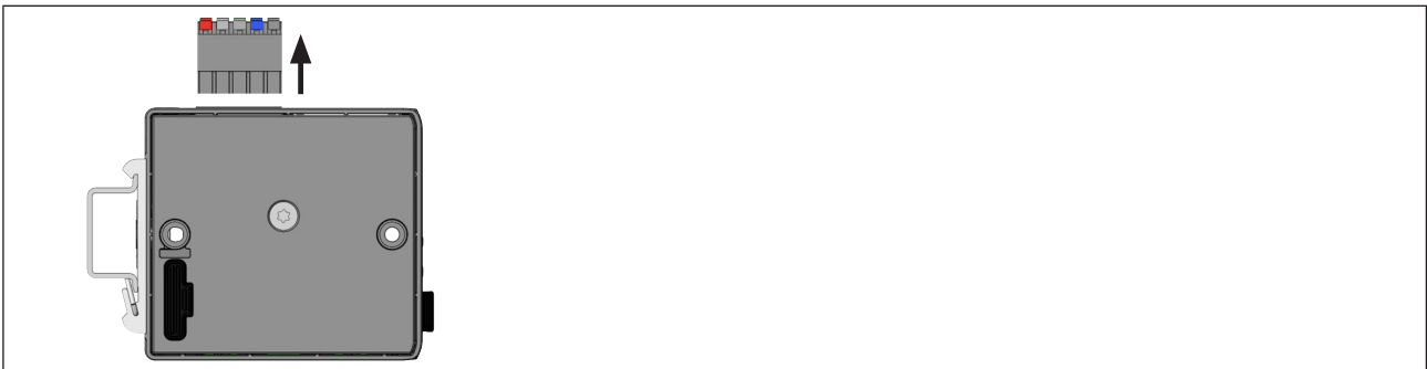
Figure 35: Remove 5-pin spring-loaded terminal
