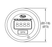
The Series LPI is a loop powered indicator with a 4-digit red LED display. The Series LPI accepts a 4-20 mA input signal and displays the associated process variable. The instrument configuration settings are selectable via a simple to use menu system, which is navigated by the use of three push-button keys located on the rear of the display. The entire assembly is sealed into a cap that fits directly onto the connecting heads.
