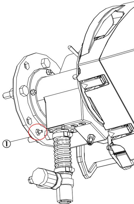
Figure 22: Potential equalization on the GMP measuring probe
