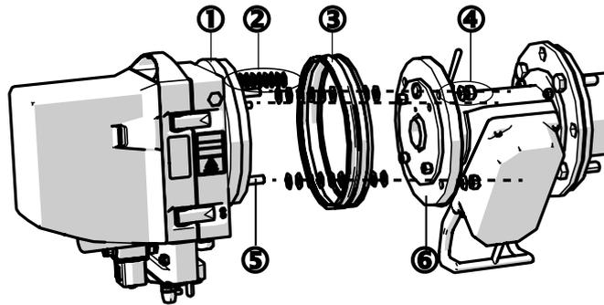
Figure 24: Fastening the GMP measuring probe on the SR-unit
