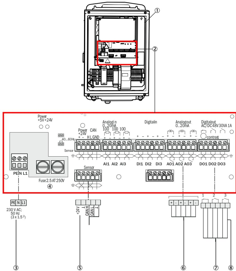
Figure 16: Electrical connection of the evaluation unit
