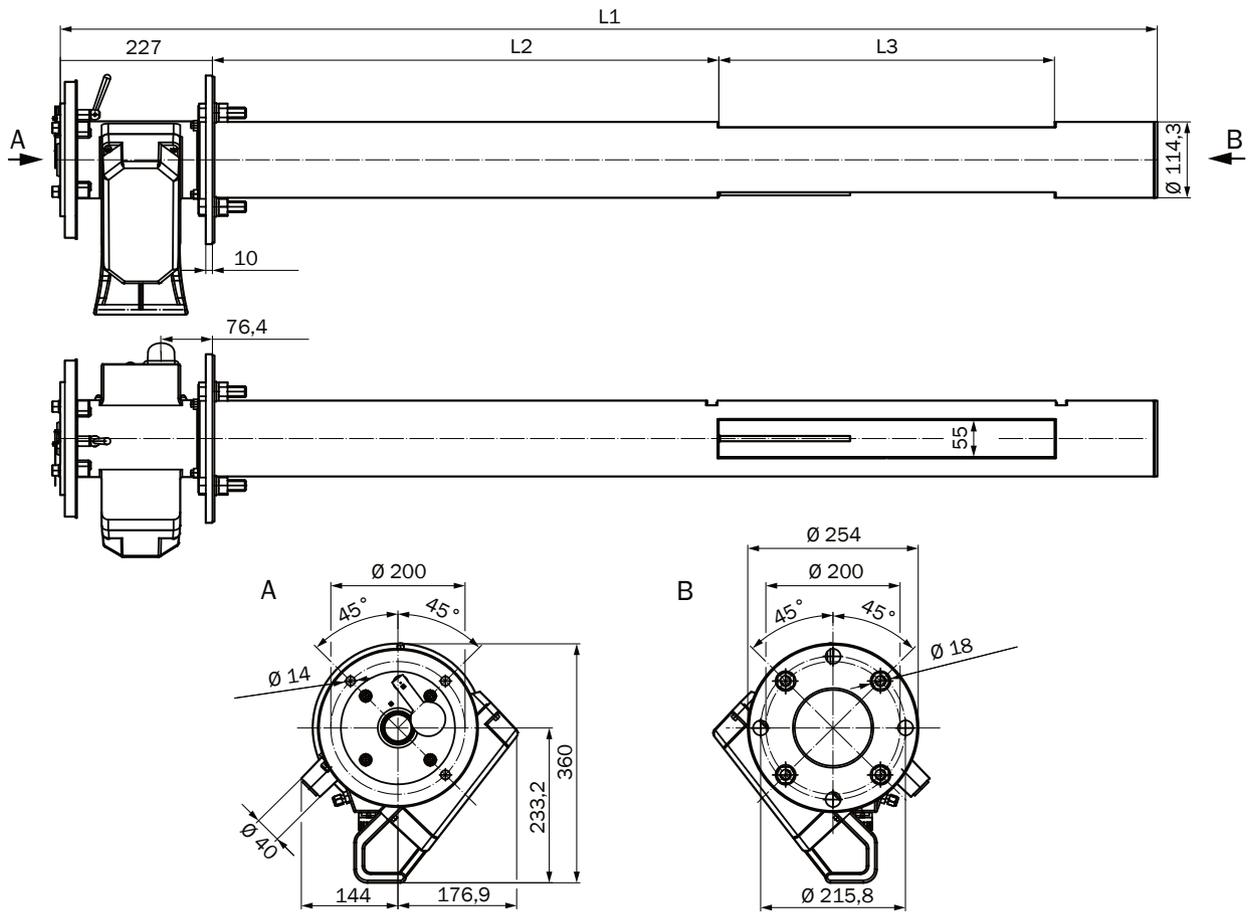
Figure 38: GMP measuring probe (all dimensions in mm)
