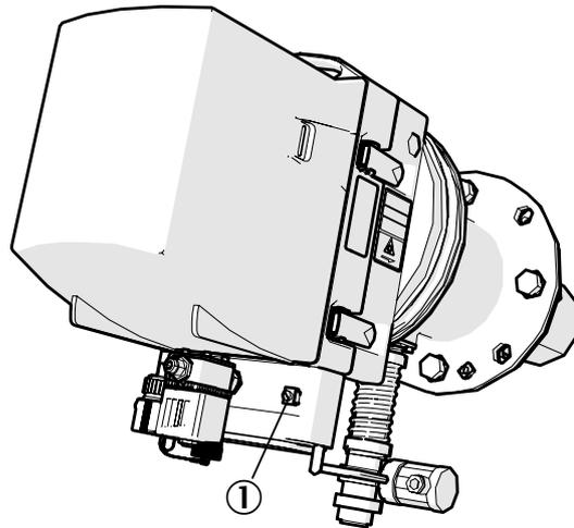
Figure 21: Connecting the potential equalization on the SR-unit
