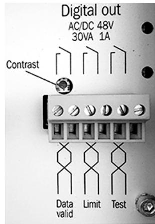
Figure 31: Rotary potentiometer for display contrast
