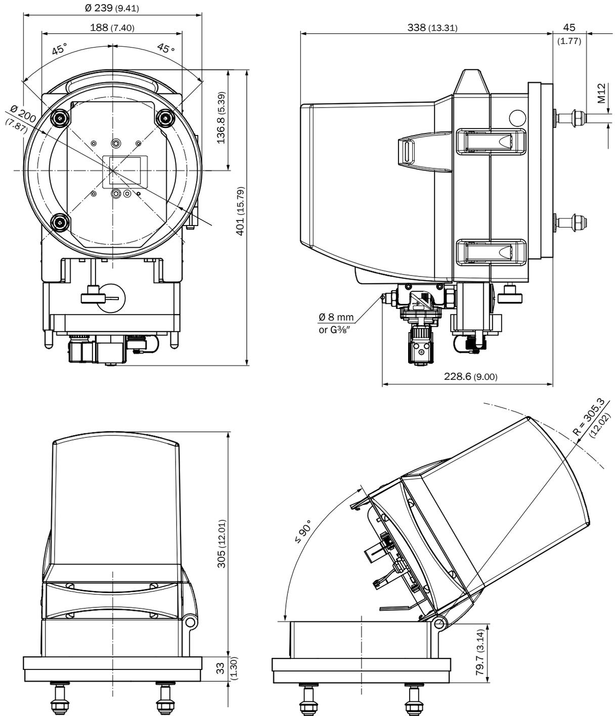
Figure 37: GM700 Ex 3G sender/receiver unit (all dimensions in mm)
