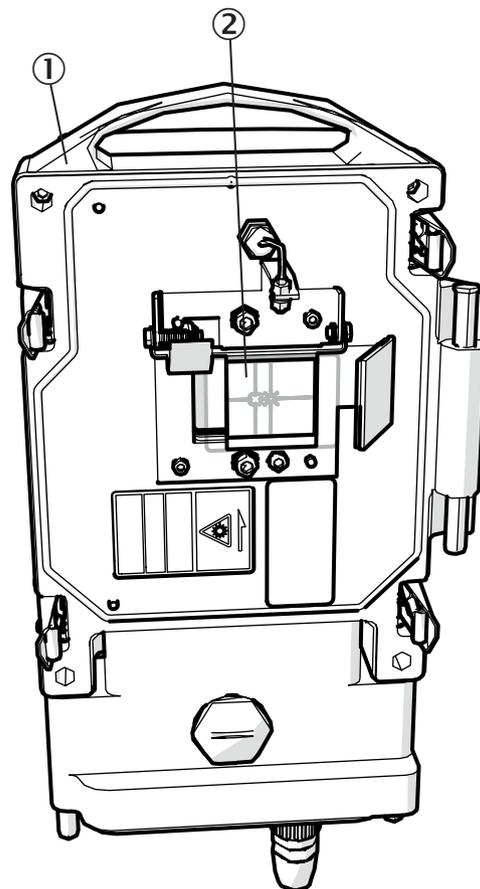
Figure 33: Optical interfaces on the SR-unit
