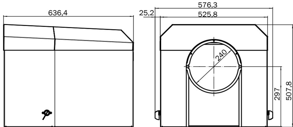
Figure 42: Weatherproof cover for sender/receiver unit (all specifications in mm)
