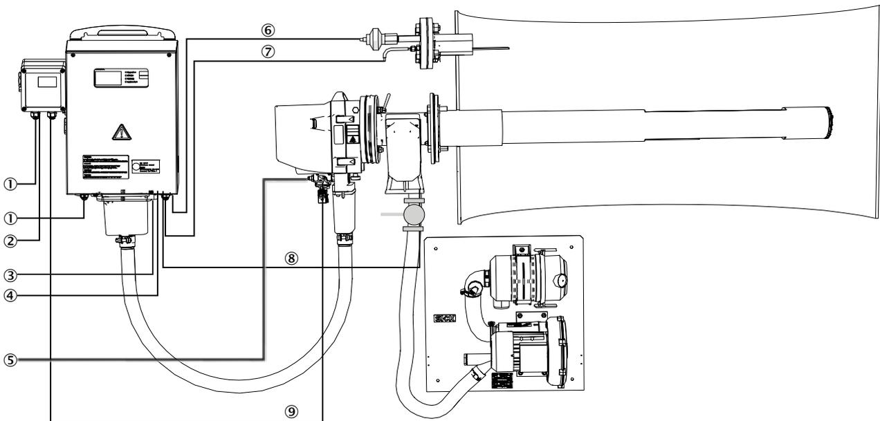
Figure 13: GM700 Ex 3G / zone 2 connection diagram
