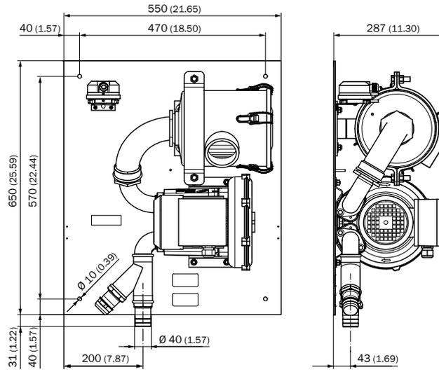
Figure 39: Dimensions, purge air unit (all dimensions in mm (inch))
