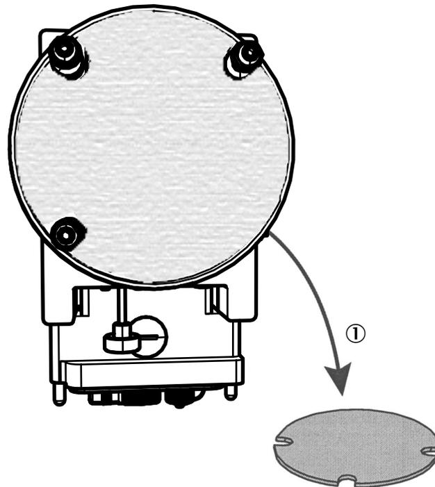
Figure 7: Transport safety device on the SR-unit
