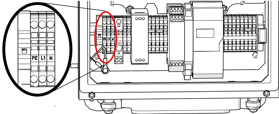
Figure 18: Power connection in the evaluation unit, power supply 230V / 50 Hz
