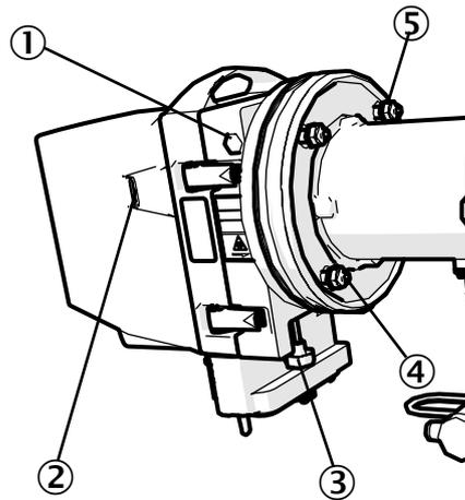
Figure 28: Components of the alignment tool on the SR-unit
