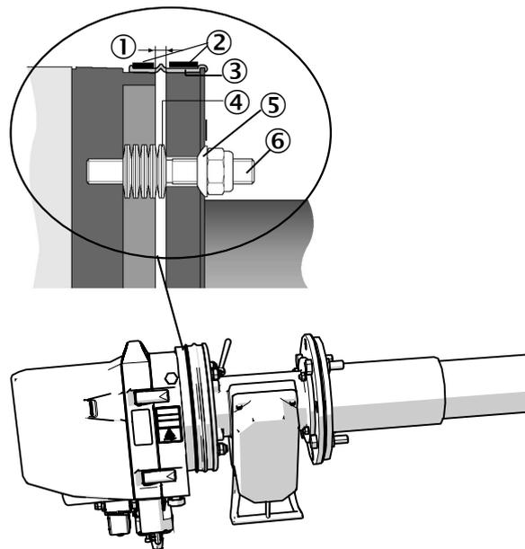
Figure 25: Cross-section of the connection fitted between the SR-unit and measuring probe
