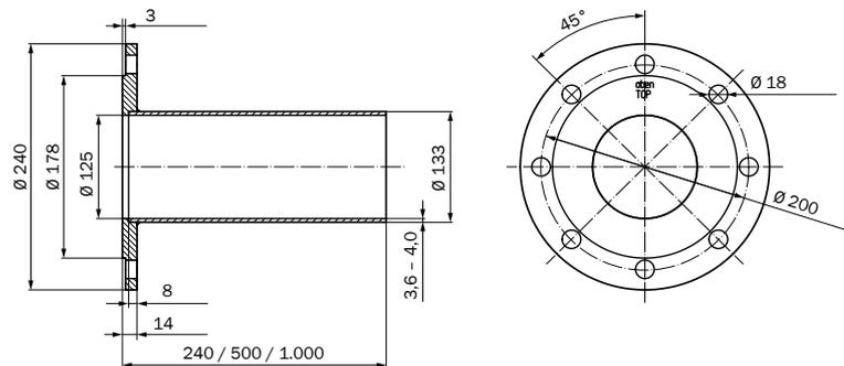
Figure 41: Mounting flange DN125 (all specifications in mm)
