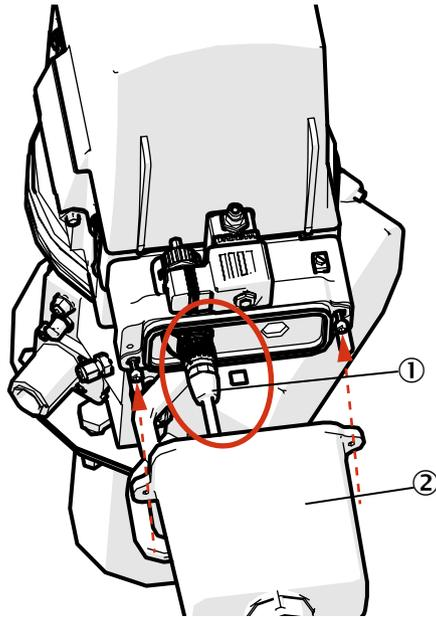
Figure 20: Connection of connecting hose with the SR-unit
