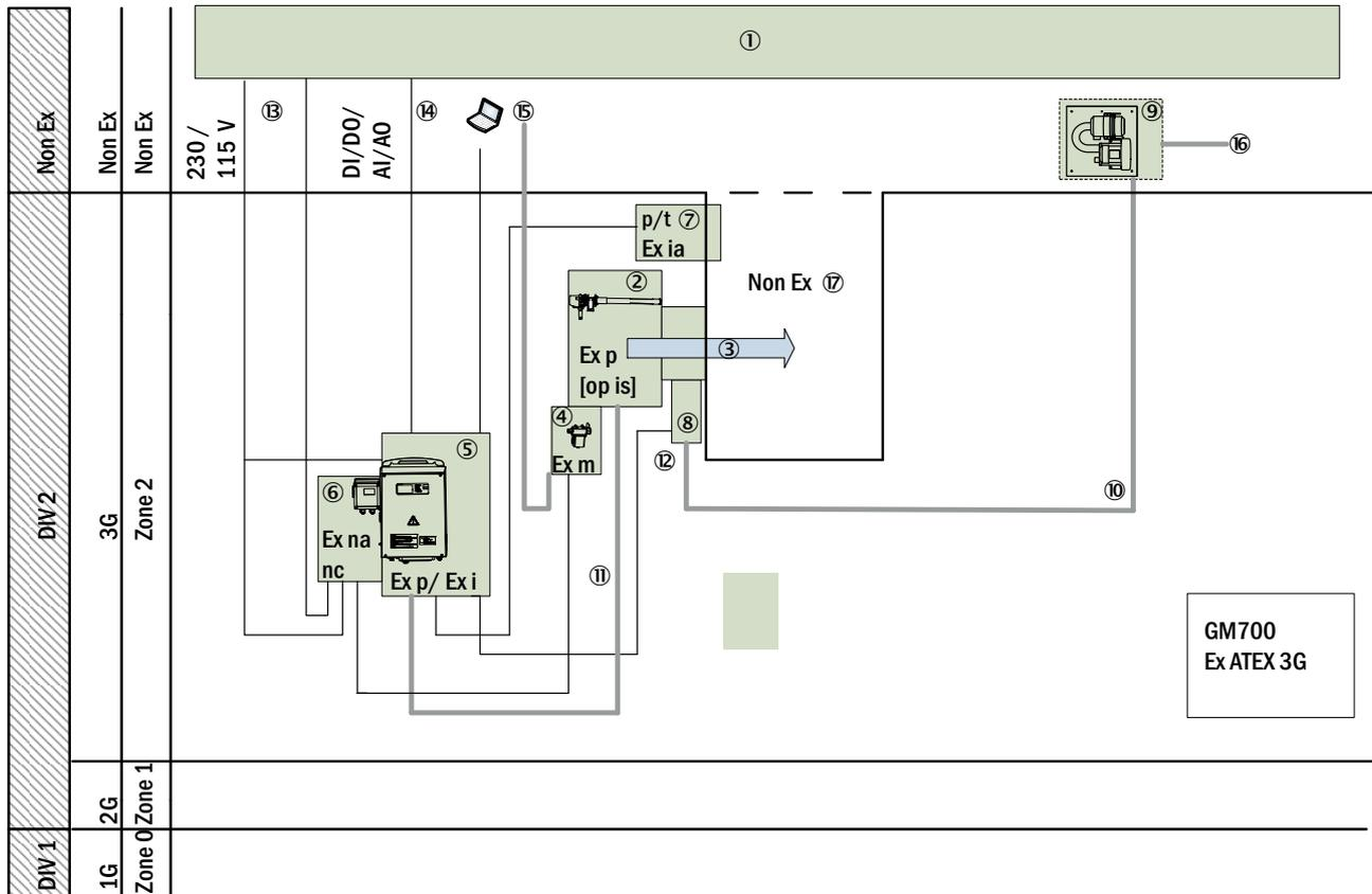
Figure 5: Zone of use GM700 Ex 3G components
