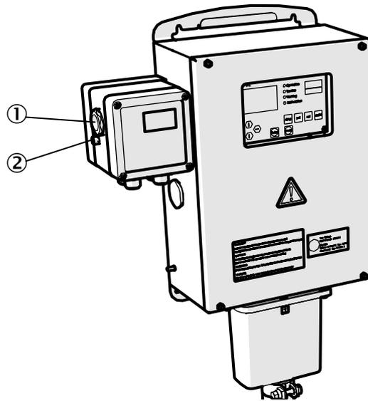
Figure 12: Protective gas outlet
