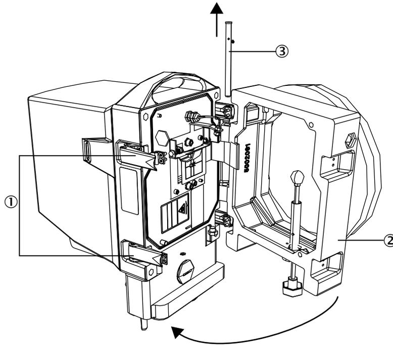
Figure 32: Opening the GM700 Ex sender/receiver unit and removing the intermediate enclosure
