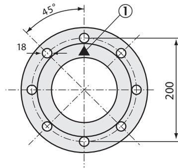
Figure 10: "Top" marking on flange with tube
