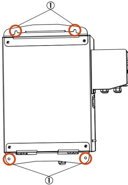
Figure 11: Assembly brackets GMA700 Ex 3G
