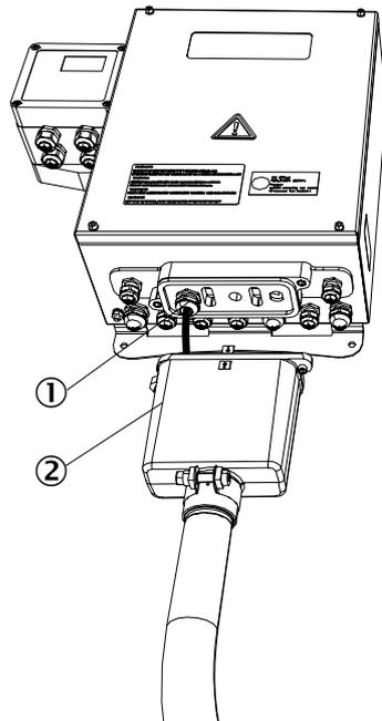
Figure 17: Connecting the connecting hose of the SR-unit on the EvU
