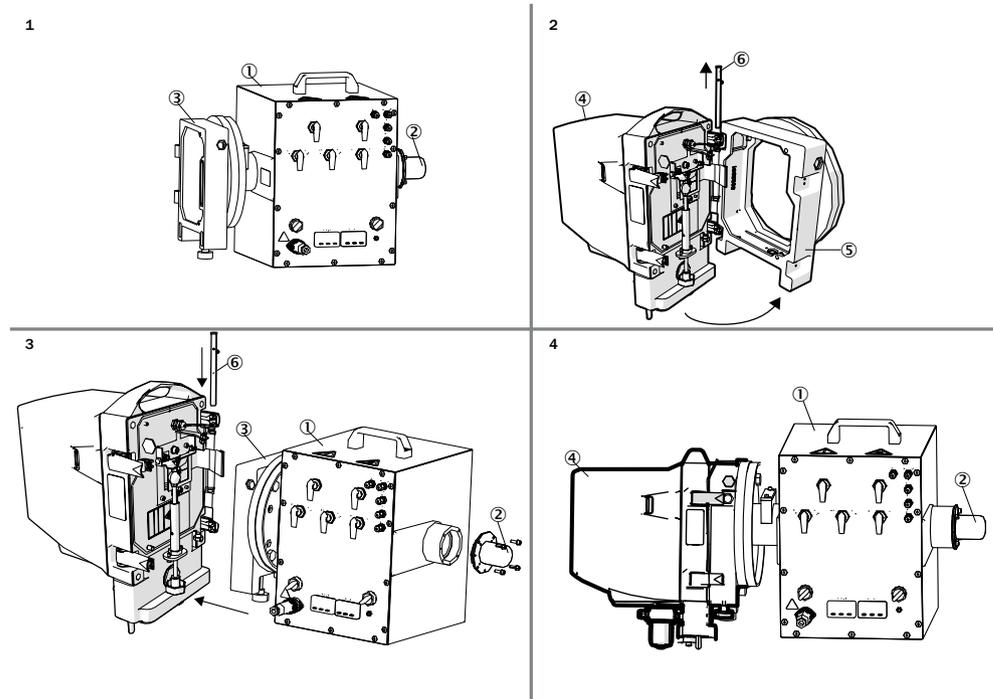
Figure 36: Fit the filter box on the measuring device
