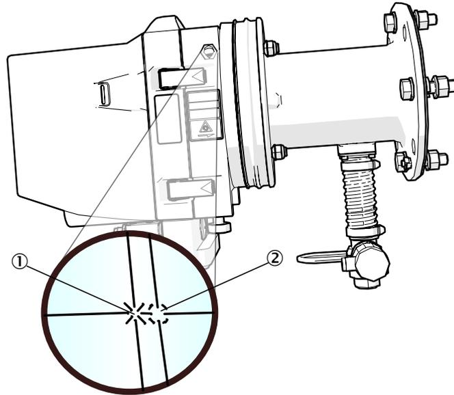
Figure 29: Point for correct fine adjustment
