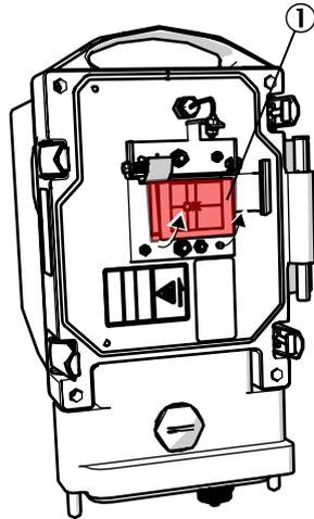
Figure 34: Flap the target holder upwards
