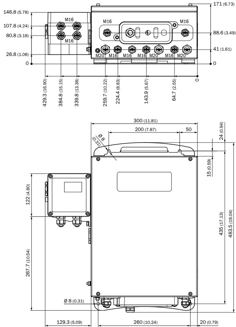
Figure 40: Evaluation unit (all dimensions in mm)
