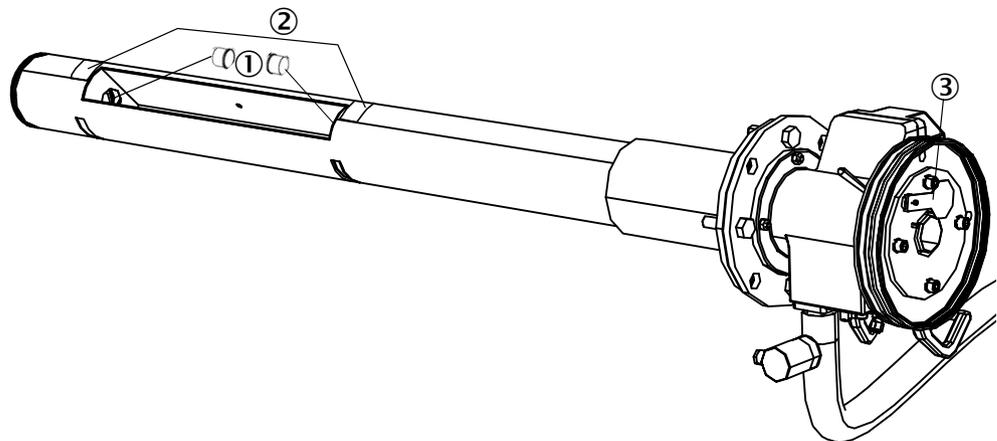
Figure 8: Transport safety device on the GMP measuring probe
