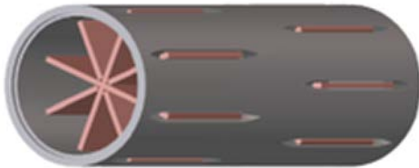
Flow rectifier with star-shaped copper plates (shown in brown)
