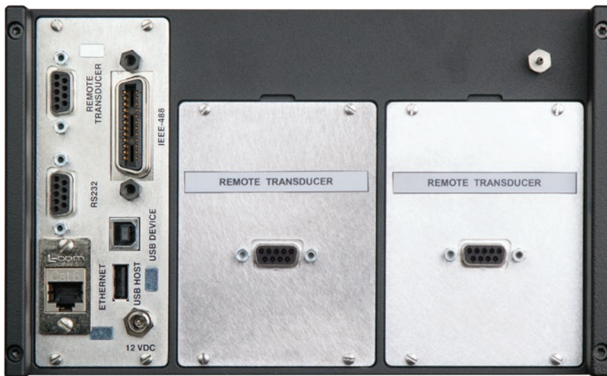
Figure 5.4 B - Two remote transducer interface connections installed
