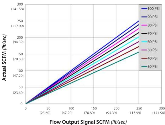
This graph illustrates the effect of varying supply pressures on the flow output signal of an FR Model Flow Transducer. This graph can be used to correct for variations in gas density due to the temperature and/or specific gravity of different gases by purposely altering the supply pressure with a Proportion-Air pressure control valve.
