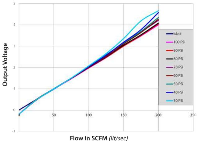
This graph illustrates how effectively the FP Model Flow Transducer automatically corrects the flow output signal when the supply pressure varies over a wide range.
