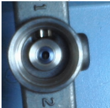
Valve seating / sealing surface in solenoid valve
