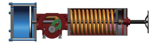
**b)** Close the valve by hand: Turning the hand wheel (counterclockwise) to loosen the spring and the stored energy overriding the actuator to closed position.
