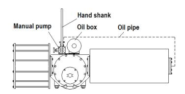
**5.2.2.2.2** Seeing the drawing below, you can find that the hydraulic cylinder is built inside of the spring cartridge. When needed to operate the the actuator / valve by hydraulic override, the two air ports on each side of the pneumatic cylinder muct be connected or open to air to sure no air pressure on the pneumatic piston.
