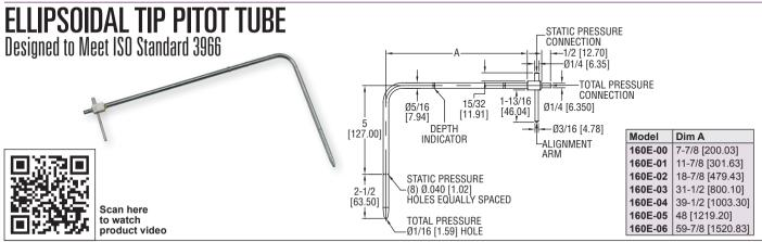
The **SERIES 160E** Ellipsoidal Tip Pitot Tube uses a precision crafted tip configuration, which allows air to pass smoothly with minimum turbulence for consistent, reliable readings. Sliding depth indicators grip firmly to ensure uniform insertion when measuring traverses across ducts. Total and static pressure taps are  $1/4^{\prime\prime}$  (6 mm) and are permanently silver soldered to the connection block, making them leak-proof and durable.
