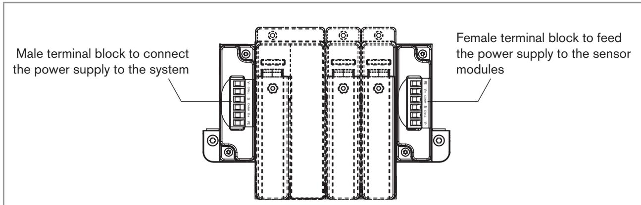
Fig. 14: Position of the terminal blocks
