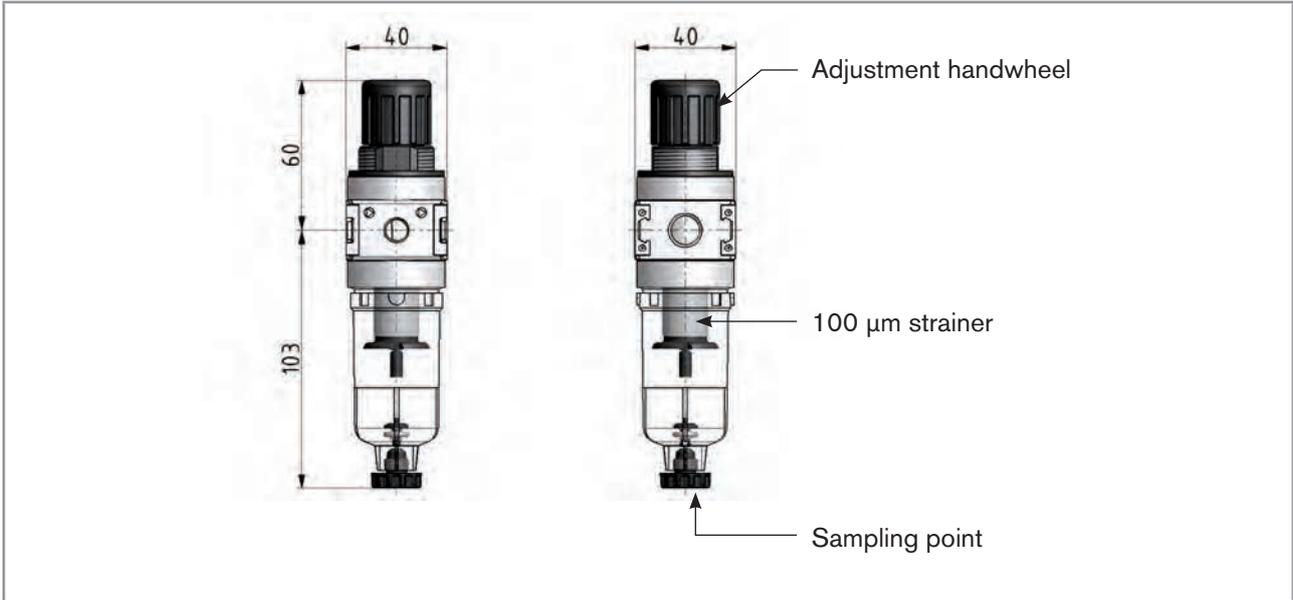
Fig. 12: Pressure reducer available as an accessory
