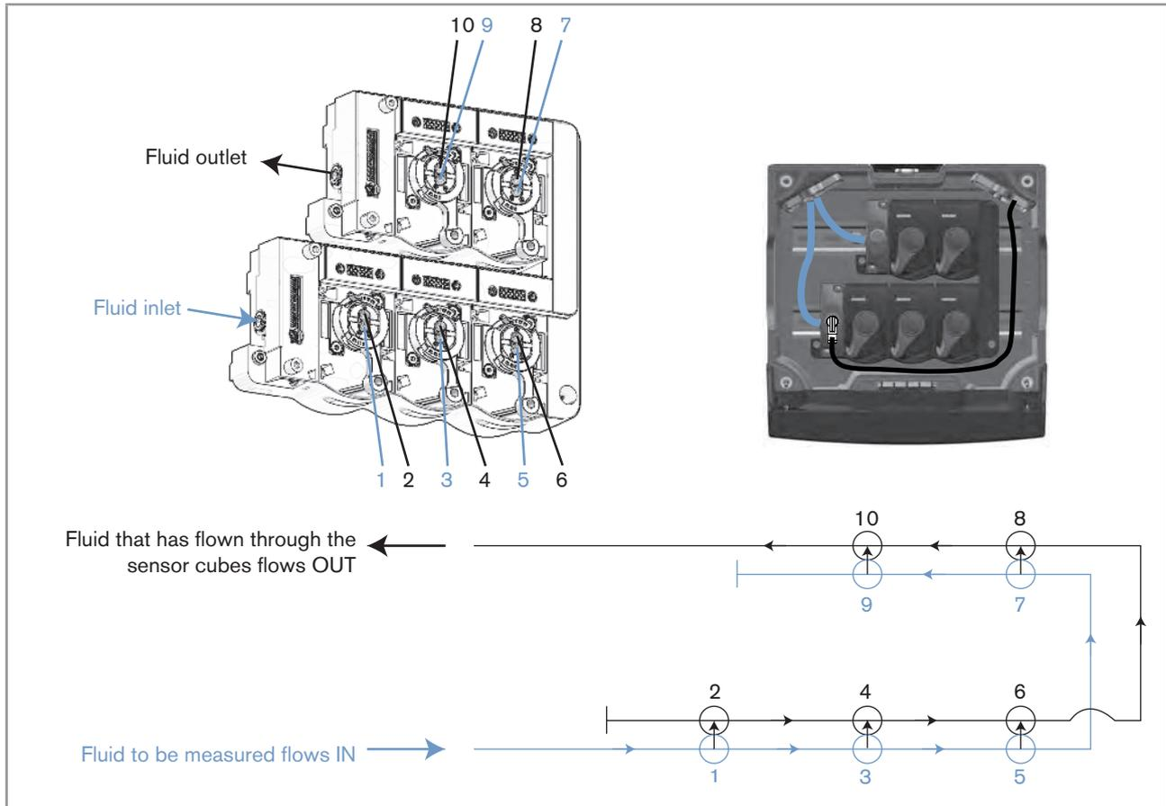
Fig. 11: Principle of the fluid circulation in the fluidic backplanes and the sensor cubes
