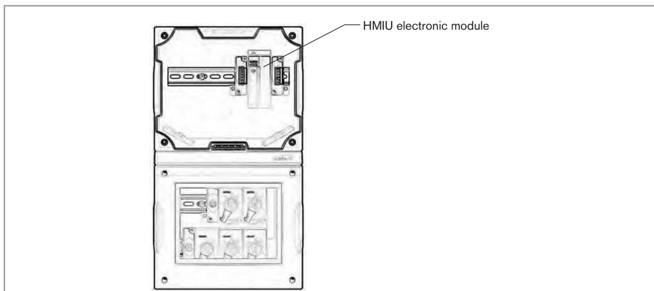
Fig. 4: Housing with the electronic modules (example of a system with 1 electronic module and no switched-mode power supply)
