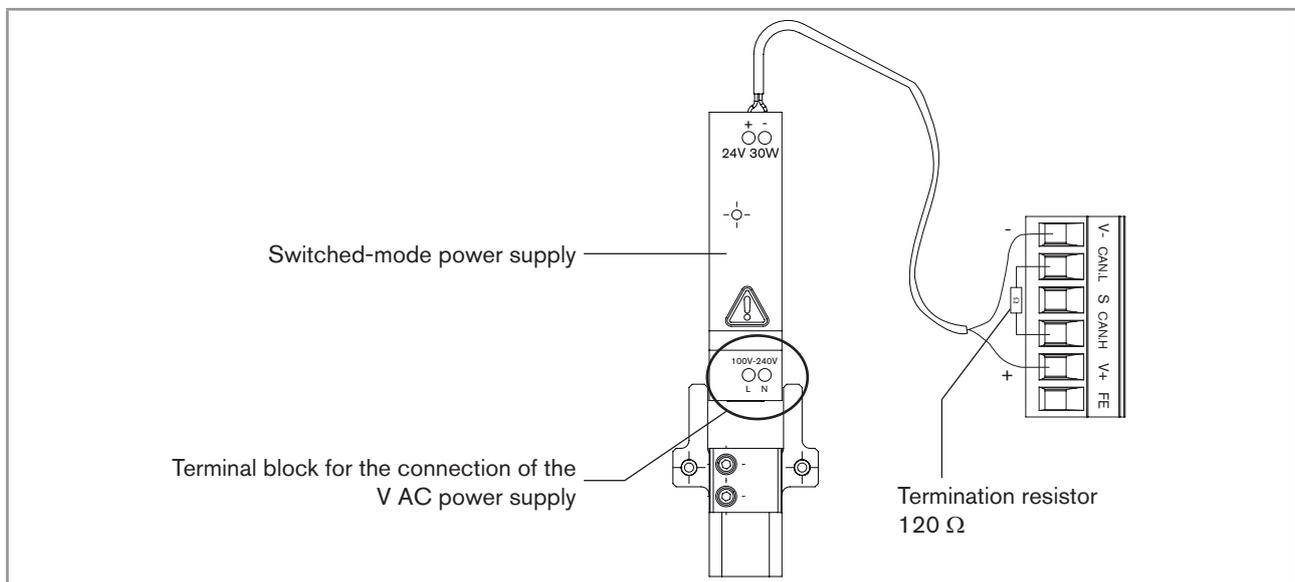
Fig. 16: Factory-made wiring of the terminal block
