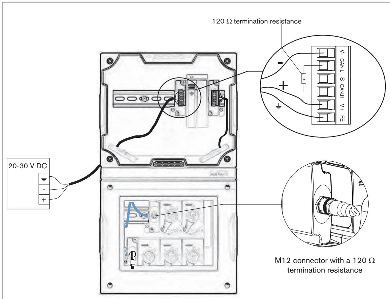
Fig. 18: Connecting the system to the VDC power supply
