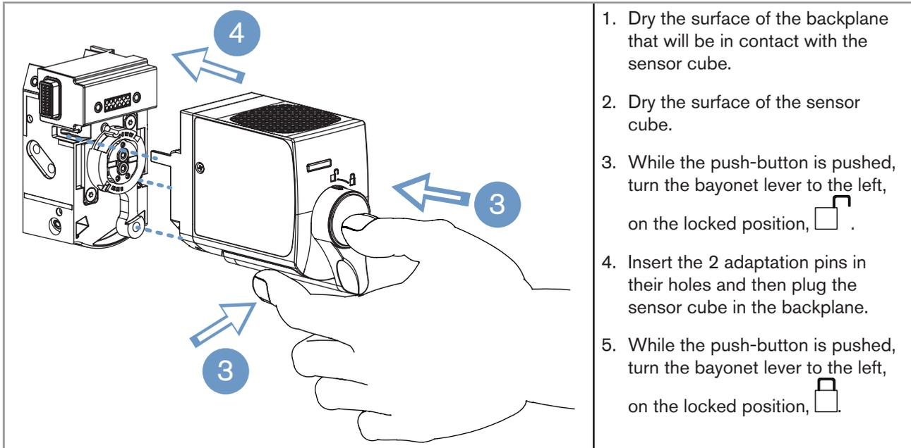
Fig. 10: Mounting a sensor cube on the backplane of the system
