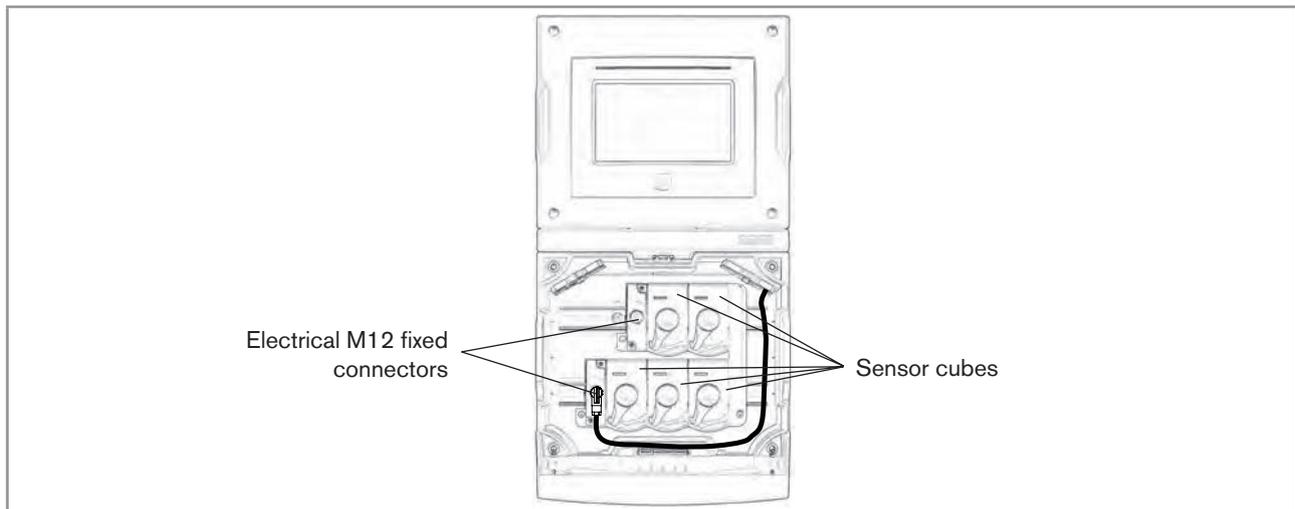
Fig. 5: Housing with the sensor cubes (example with five sensor cubes)
