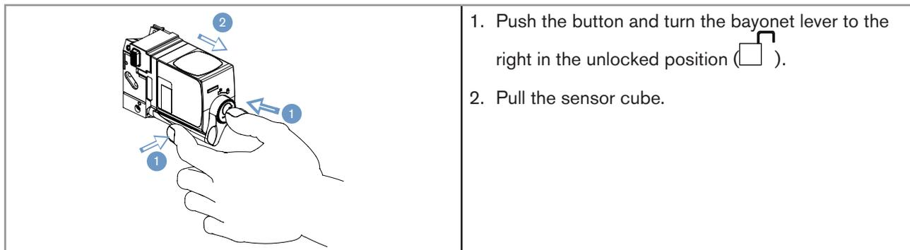
Fig. 19: Removing the sensor cube from the backplane
