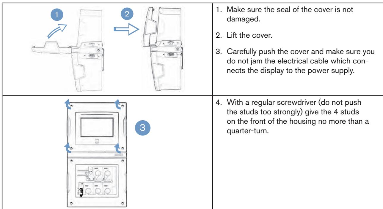
Fig. 20: Closing a housing
