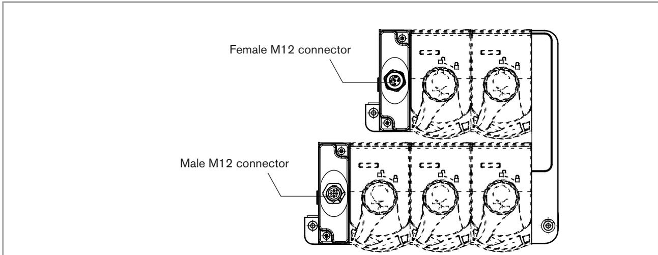
Fig. 15: Position of the M12 connectors
