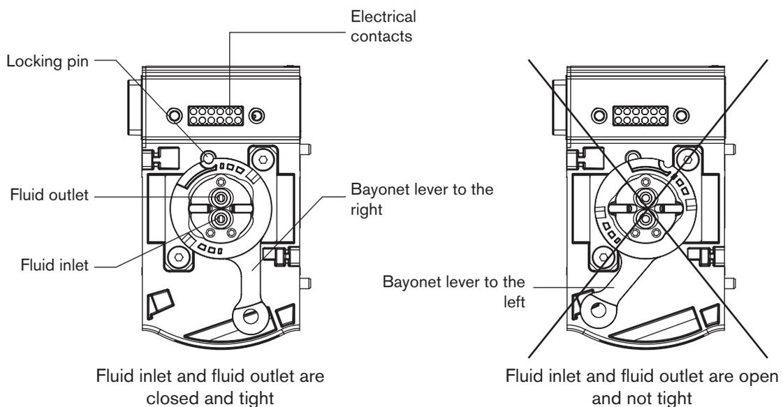
Fig. 6: Description of a sensor cube backplane
