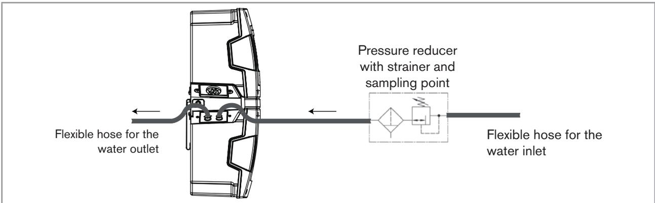
Fig. 13: Connection of the flexible tubing, outside the housing
