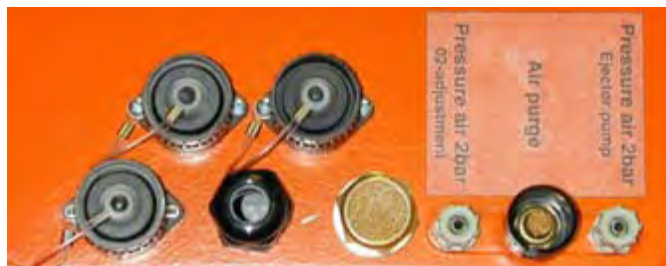
Fig. 4-6: Connections at the cast-aluminum housing
