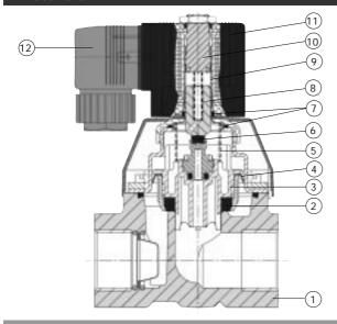
1 Valve body: **Brass** 2 Seat-seal: **NBR** 3 Piston: **PPS** 4 Gasket: **PTFE** 5 Spring: 1.4310 6 Plunger-seal: **NBR** 7 O-rings: **NBR** 8 Plunger: 1.4105 9 Armature guide tube: 1.4301 1.4105 10 Stopper: Coil Polyamide 11 12 Cable plug: Polyamide
