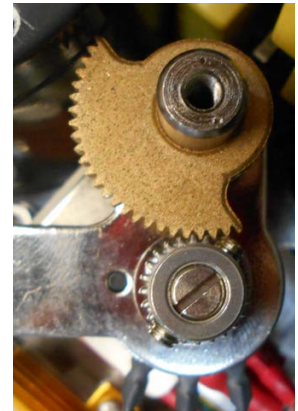
Alignment of the sector and potentiometer gear sets at actuator full CW position. (ref step 9).
