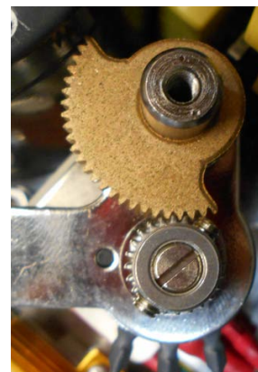
Alignment of the sector and potentiometer gear sets at actuator full CW position. (ref step 9).
