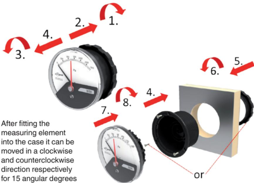
After fitting the measuring element into the case it can be moved in a clockwise and counterclockwise direction respectively for 15 angular degrees in order to ensure precise horizontal positioning of the instrument.
