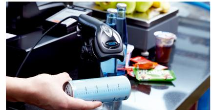
Time-saving use in presentation mode: Tedious actuation of the trigger switch is no longer necessary.
