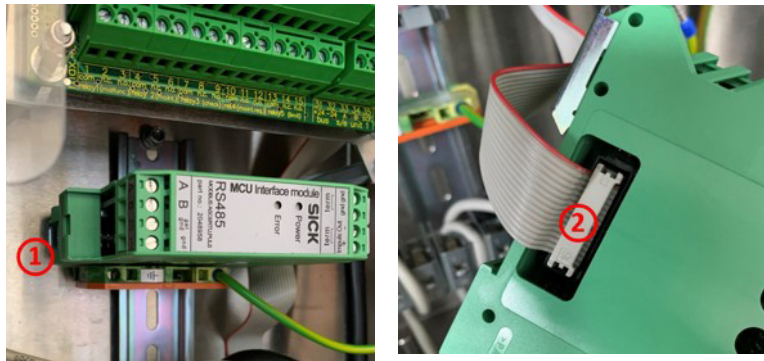
Fig. 51: Illustrations, exchanging the Interface module
