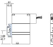
DIN Rail Kit suitable for EN-50035, EN-50045 and EN-50022 Rails
