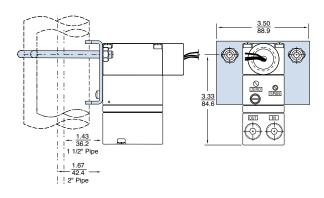
1.50 Panel Mounting 38.1 <u>.312</u> 7.92 <u>.281</u> 7.14 <u>4.86</u> <u>4.50</u> 114.3 123.4 OUT IN <u>2.43</u> 61.7  $\overline{\odot}\overline{\odot}$ Mount using (2) #1/4-20 screws not included in kit
