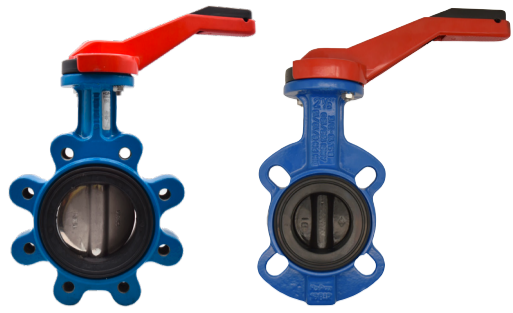
Butterfly Valve Type 038 Lug style Butterfly Valve Type 039 Wafer style
