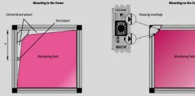
On mounting in the frame there will be unmonitored areas due to the mounting principle. This situation can result in the failure to detect objects. You can identify the unmonitored areas with the aid of a test object.
