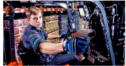
Thanks to the 75 cm reading distance, codes on piece goods and pallets can be conveniently identified from manned forklift trucks.
