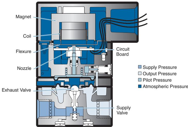
The Type 550X I/P, E/P Transducer is a force balance device in which a coil is suspended in a magnetic field by a flexure. Current flowing through the coil generates movement of the flexure. As this assembly moves towards the nozzle, it creates backpressure, which acts as a pilot to an integral booster relay. Input signal increases (or decreases for reverse acting) cause an accurate proportional change in output.
