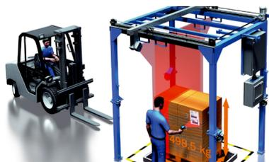
Stationary volume measurement systems often require mobile code reading for identifying goods: AUX connectivity provides a cost-effective solution.
