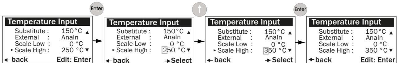
Figure 44: Setting the upper limit value for the temperature range (example)
