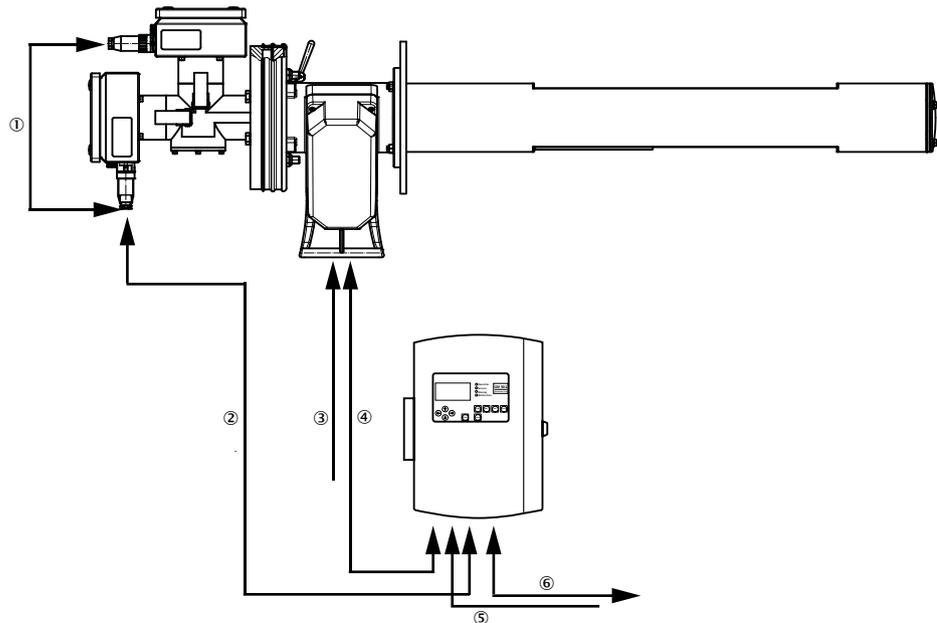
Figure 13: Connection diagram for standard version
