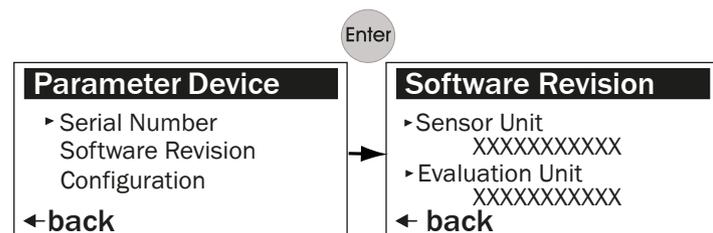
Figure 54: Calling up the current software version
