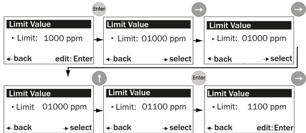
Figure 39: Setting the limit value (example)
