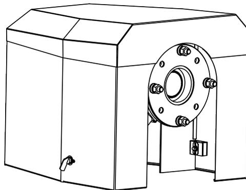
Figure 27: Placing the weatherproof cover on the installation plate
