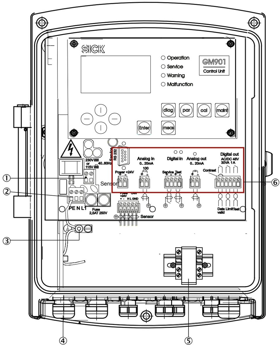
Figure 14: Electrical wiring of the evaluation unit
