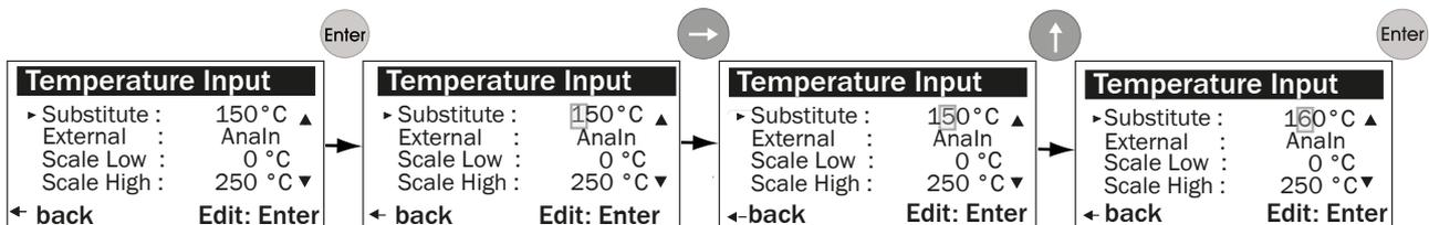
Figure 41: Setting the default temperature setting (example)
