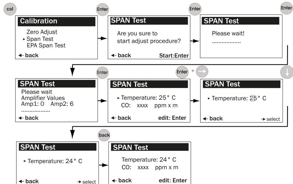
Figure 59: Performing a manual SPAN test
