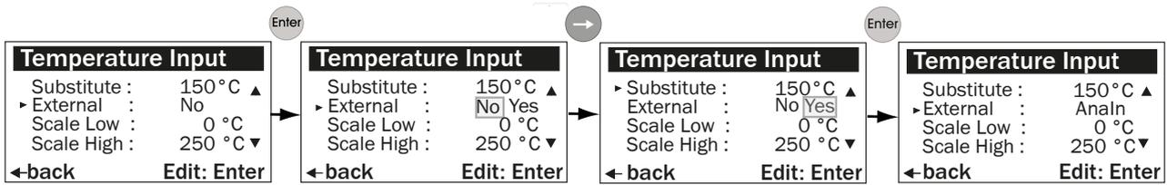
Figure 42: Activating the use of an external temperature sensor
