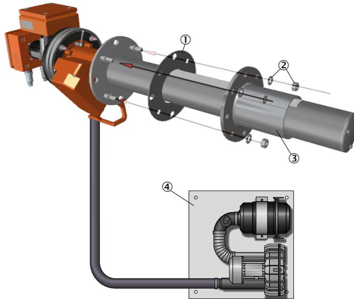
Figure 23: Installing the device on the duct flange
