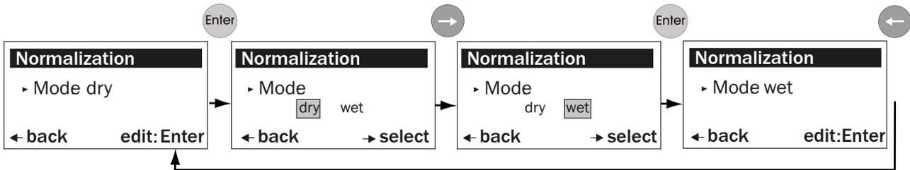
Figure 36: Selecting the humidity correction
