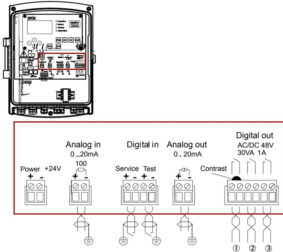
Figure 15: EvU connections for customer wiring
