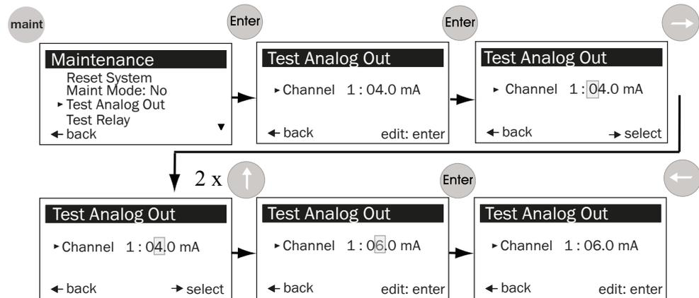
Figure 64: Setting the analog value
