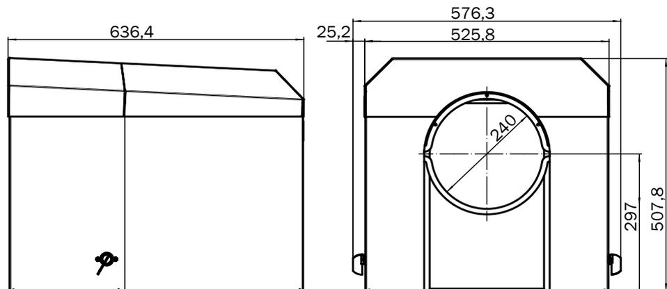
Figure 75: Weatherproof cover for sender/receiver unit
