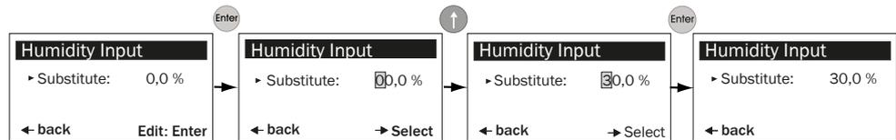
Figure 47: Entering the default value for humidity content in sample gas (example)
