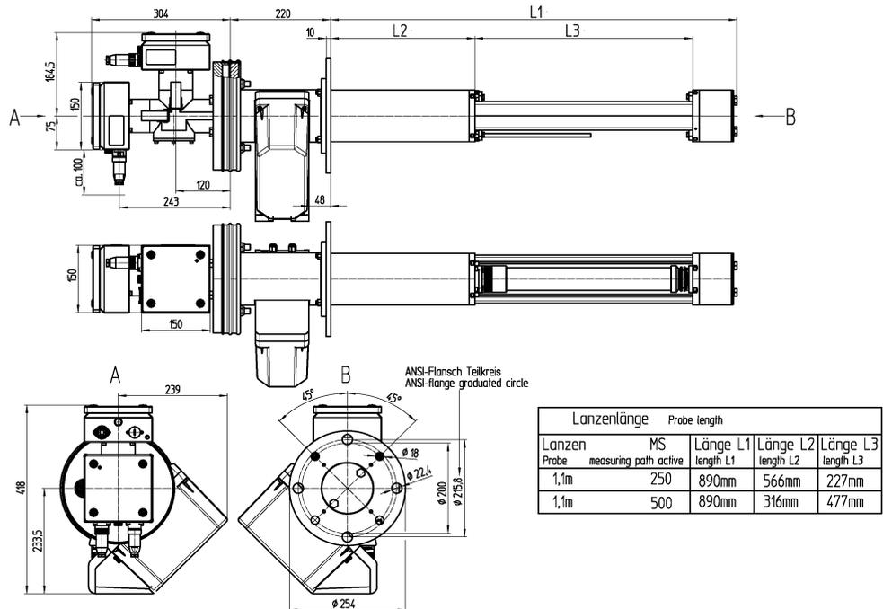
Figure 71: Dimensions, GM901-02 sender/receiver unit with GPP probe (all specifications in mm)
