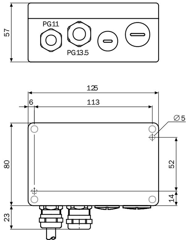
Figure 74: Dimensions, terminal box (all specifications in mm)
