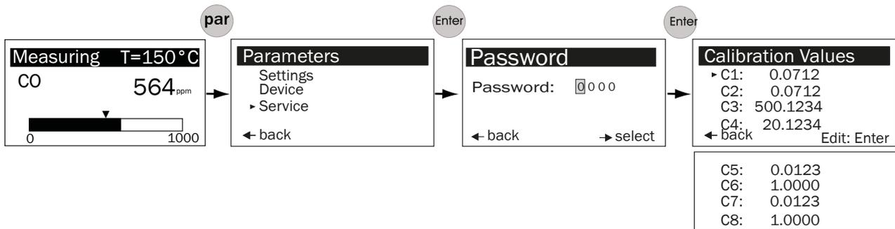
Figure 56: Calling up the device calibration data
