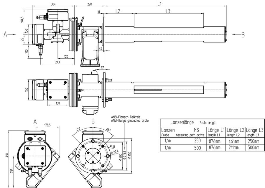
Figure 70: Dimensions, GM901-02 sender/receiver unit with GMP probe (all specifications in mm)
