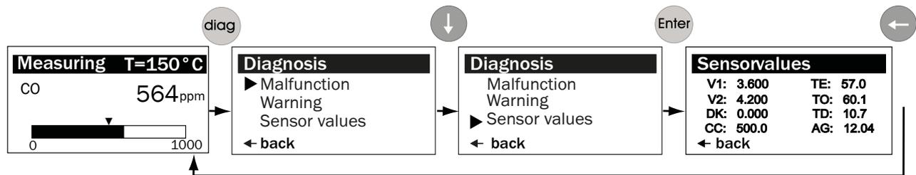
Figure 33: Viewing sensor values (example)
