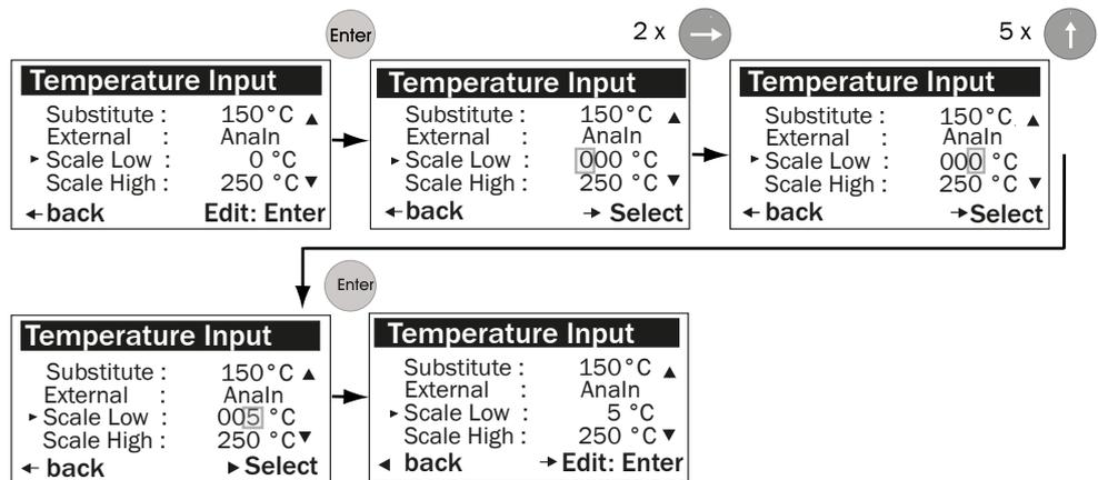
Figure 43: Setting the lower limit value for the temperature range (example) (corresponds to Live Zero)
