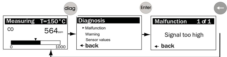
Figure 31: Viewing error messages (example)
