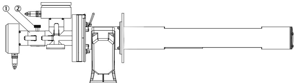
Figure 18: GM901-02 with holder for test cell
