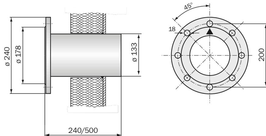
Figure 11: Mounting flange
