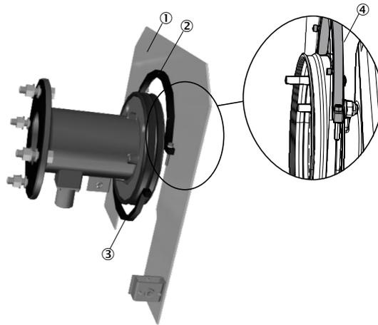
Figure 26: Detail view: Positioning the top mounting ring on the side of the purge air fixture
