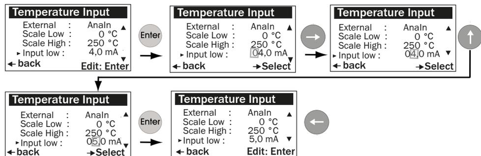
Figure 45: Setting the lower measuring range value (Live Zero) (example)
