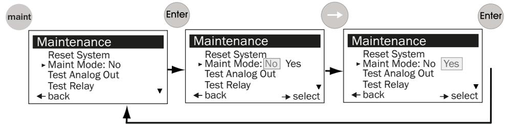
Figure 63: Activating/deactivating maintenance mode
