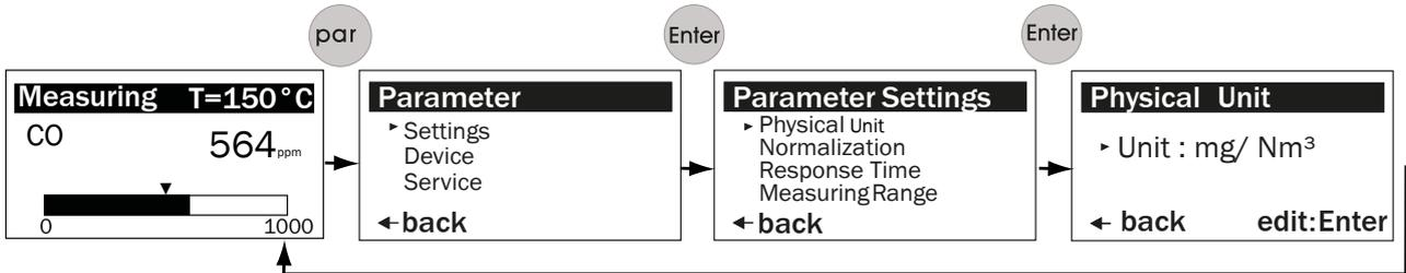
Figure 34: Path from Measuring Screen to change parameters (example)
