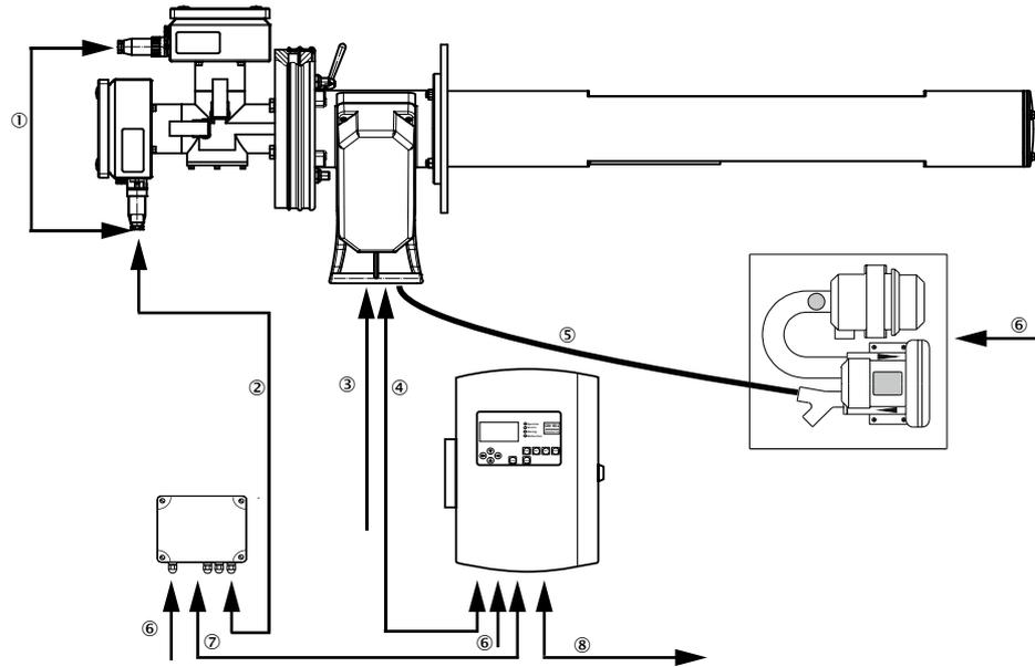
Figure 16: Wiring with terminal box and detached evaluation unit
