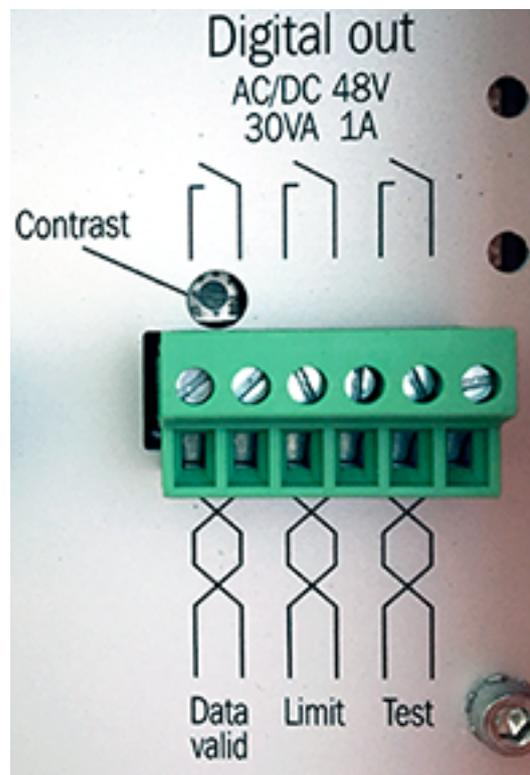
Figure 29: Rotary potentiometer to adjust the display contrast
