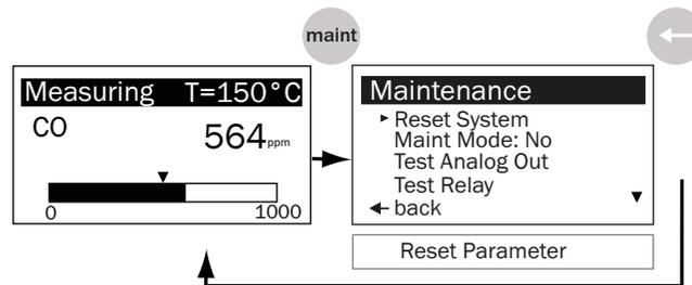
Figure 61: Path from Measuring Screen to change parameters (example)
