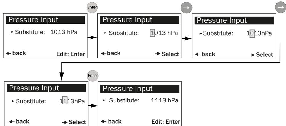
Figure 48: Entering the default value for the sample gas pressure (example)
