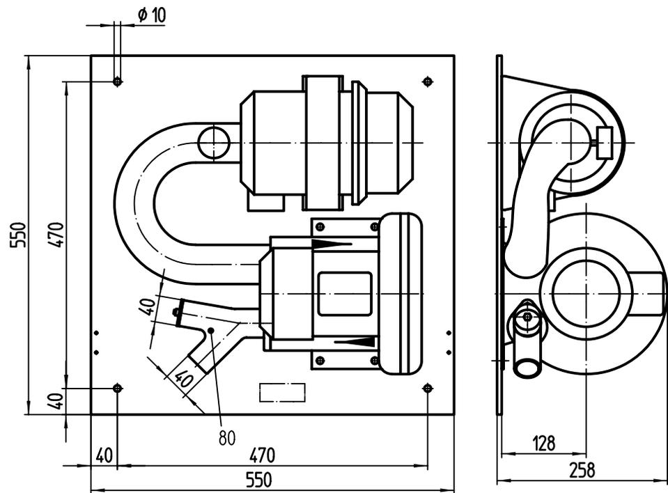
Figure 73: Dimensions, evaluation unit (all specifications in mm)
