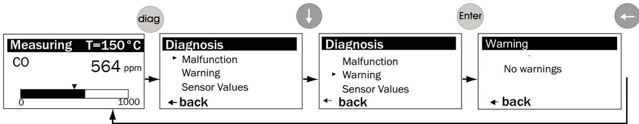
Figure 32: Viewing warning messages (example)
