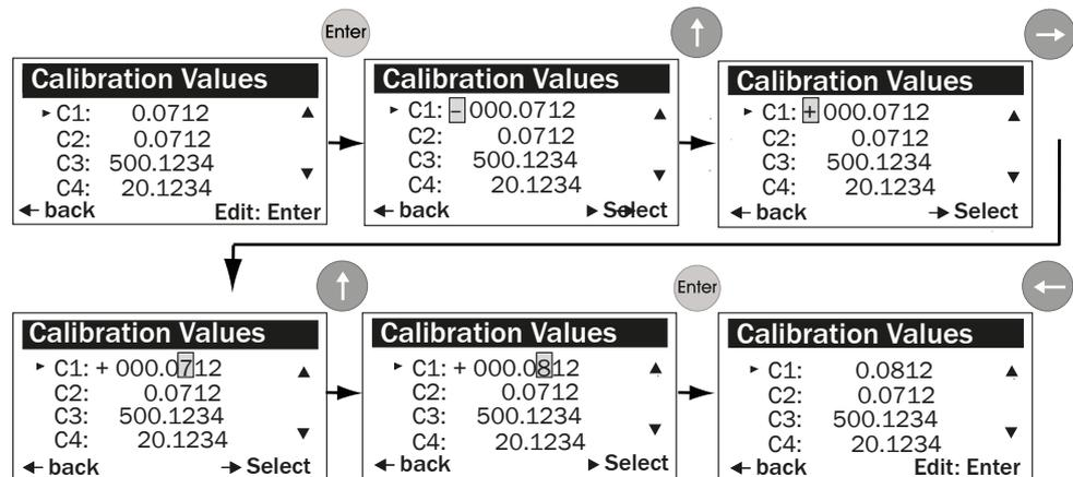
Figure 57: Changing device calibration data
