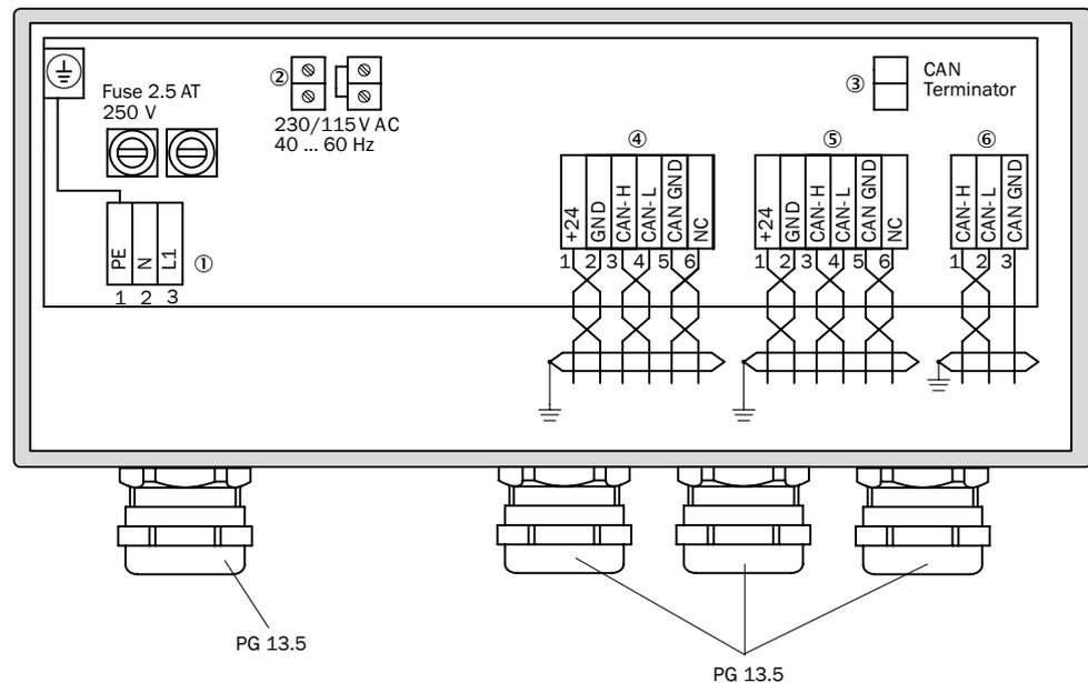
Figure 17: Terminal box customer wiring
