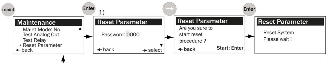
Figure 66: Resetting parameters to the factory settings
