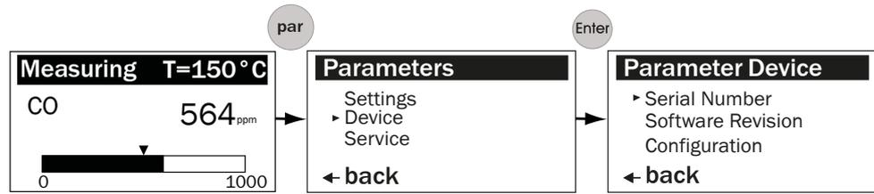
Figure 52: Path from Measuring Screen to Device Characteristic Data
