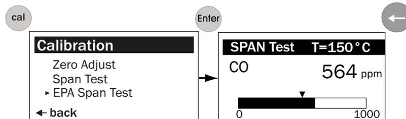
Figure 60: Performing a manual SPAN test
