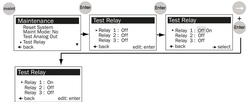
Figure 65: Testing relays 1, 2 and 3
