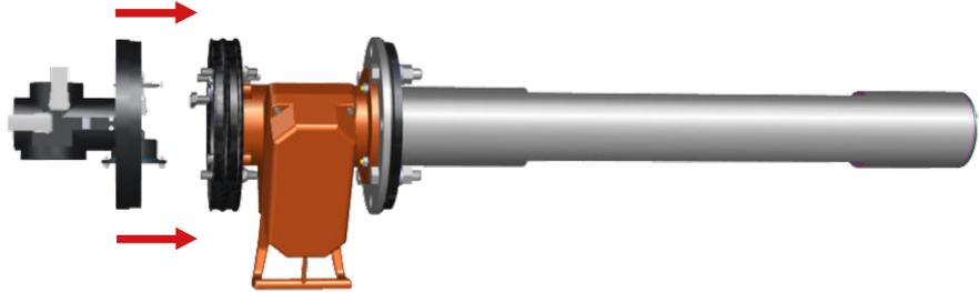
Figure 20: Fitting the T-piece on the measuring probe
