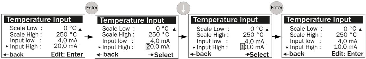
Figure 46: Changing the value for the upper output value (example)
