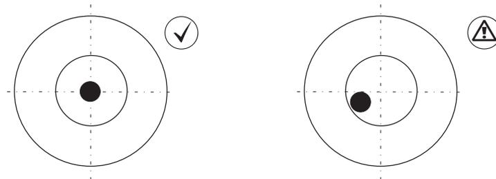
Figure 21: Light point on the focusing screen
