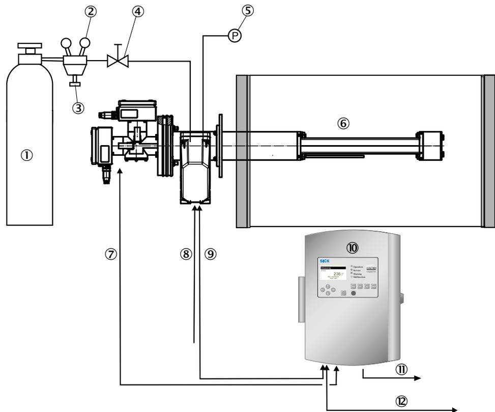
Figure 19: Equipment for the manual SPAN test
