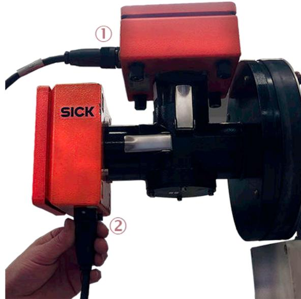
Figure 24: Connecting the CAN line between sender and receiver
