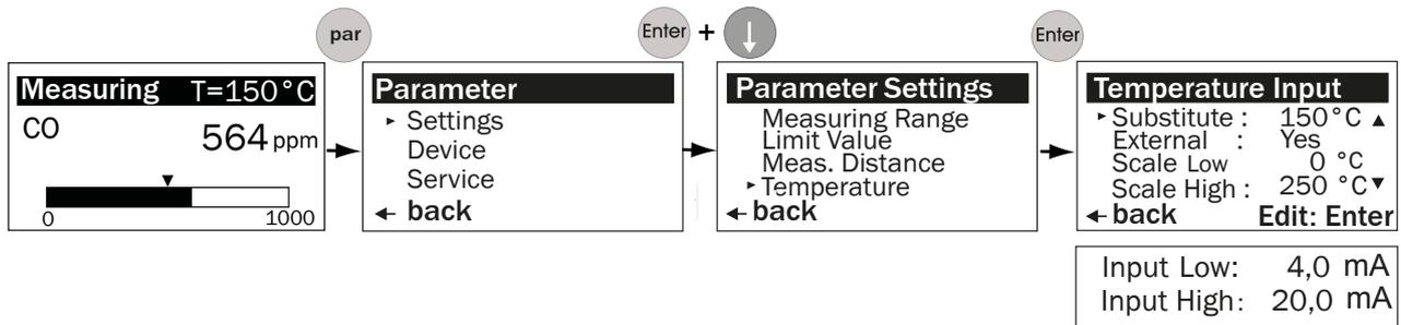
Figure 40: Setting the parameters for the temperature sensor PT1000
