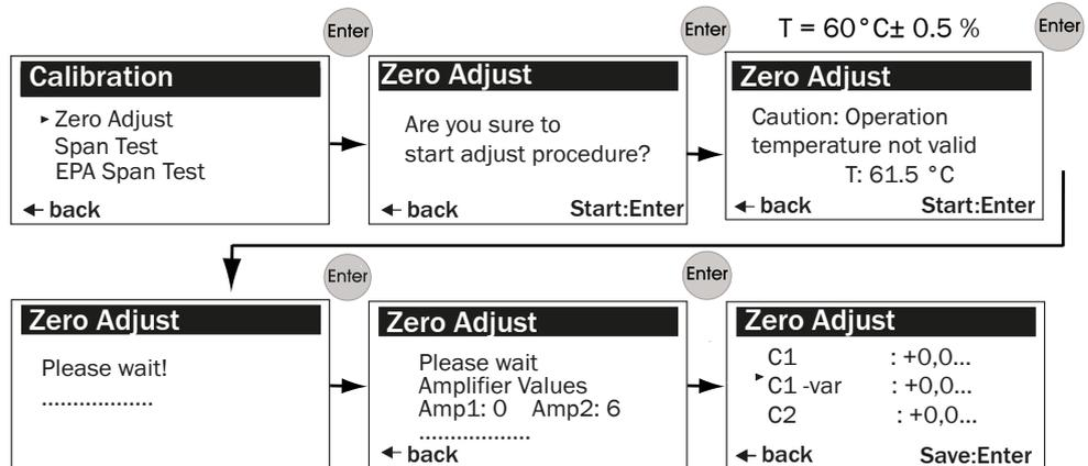
Figure 58: Performing zero adjust
