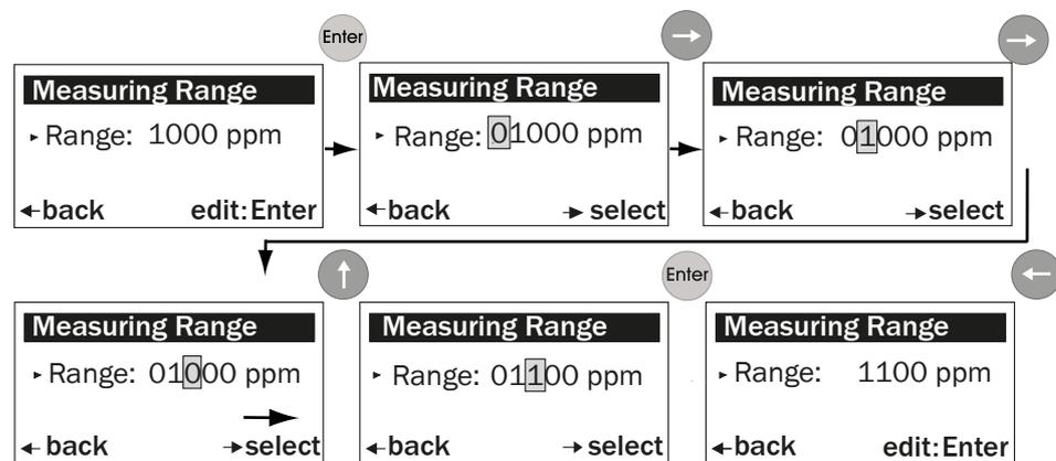
Figure 38: Changing the measuring range (example)
