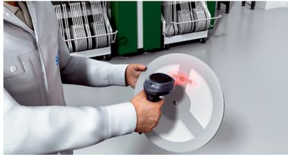
Mobile identification of placement material. Fast code identification in any orientation thanks to integrated matrix camera.
