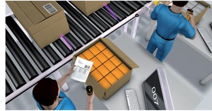
The hand-held scanner is suitable for reading 1D, 2D, and stacked codes during the collection of consignments.
