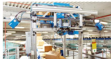
Easy PROFIBUS integration into large track-and-trace systems with the CDF600 fieldbus module.
