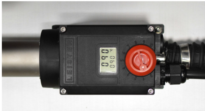
Fig. 2: Purge air heater
