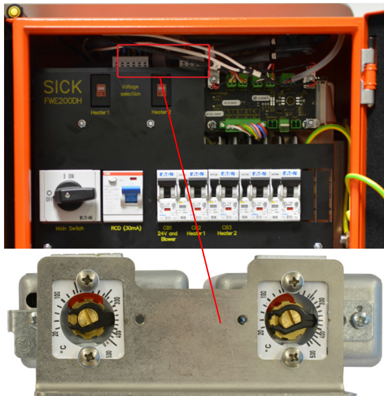
Fig. 8: Heating band settings on control unit
