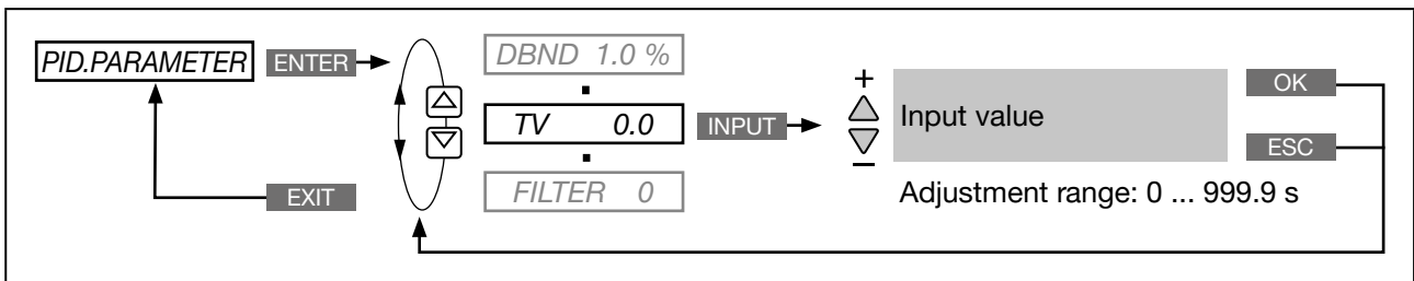
Fig. 56: Operating structure TV; hold-back time
