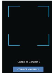
**NOTE:** If the connection between Fluke Connect and the gateway fails, a hint to retry the process appears. Try to rescan the QR code. If gateway details were entered manually, retry scanning the QR code.
