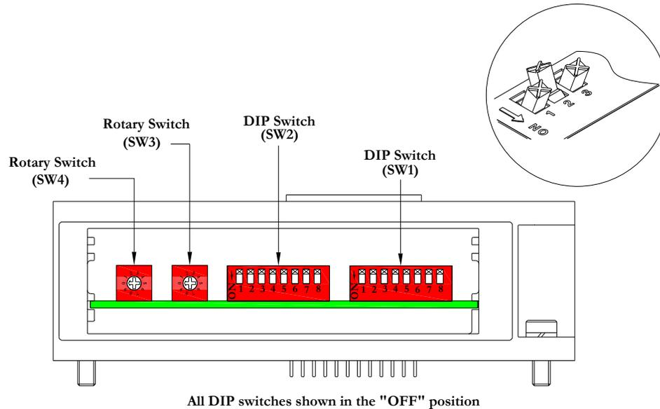
The MCM is the module that allows the user to manually test the Numatics manifold using Self-Test mode. The MCM consists of two DIP switch sets (SW1 and SW2) and two rotary switches (SW3 and SW4).
