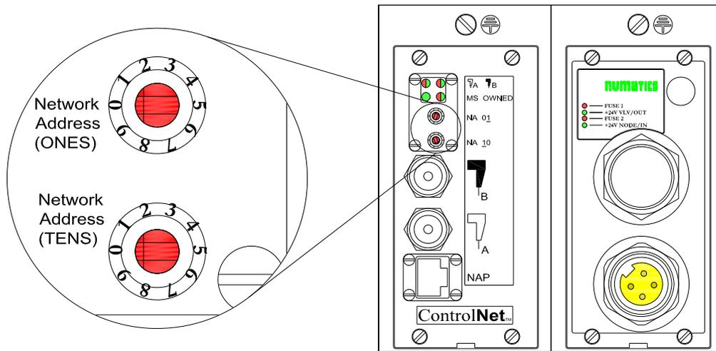
The Rotary switches allow the user to set the node address.
