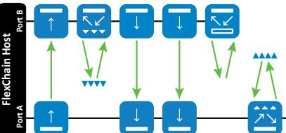
Optimum measurement certainty: Sequential cycling prevents the signals from overlapping
