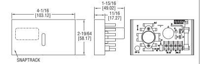
The MODEL BPS-015 Building Automation Power Supply is used to convert 24 VAC to a regulated DC power source for transmitters with 4 to 20 mA outputs. The output voltage can be field adjusted from 1.5 V to 27 V using a potentiometer. The 3 A fuse protects the power supply from over-current conditions. The snap-on bracket can be quickly surface mounted to any flat surface.
