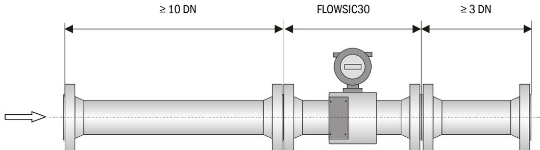
In order to achieve the specified meter accuracy, ensure 10D of straight inlet and 3D of straight outlet pipe length as a minimum.
