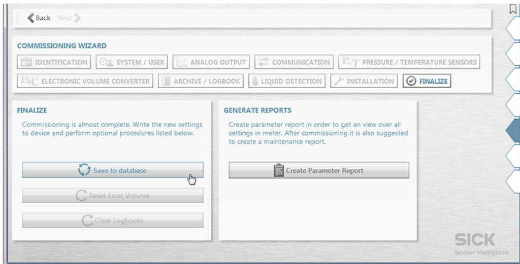
Individual parameters can also be checked and changed at a later time after commissioning via the menu “Parameter Modification”, → Fig. 29.
