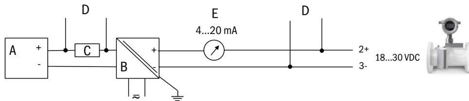
Fig. 12 Intrinsically safe installation, HART® + Modbus RS485 output
