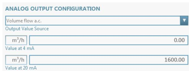
Further parameters such as damping, error value, gain and current offset can be set.
