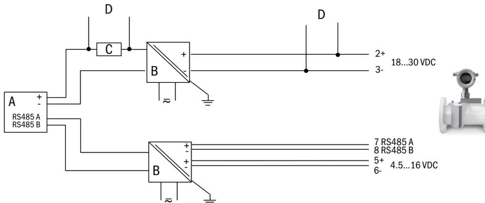
Fig. 13 Intrinsically safe installation, HART® + Modbus RS485 output + external pressure sensor
