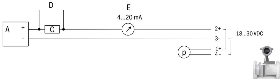
Fig. 16 Non-intrinsically safe installation, HART® + Modbus RS485 output
