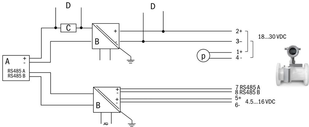
Fig. 14 Non-intrinsically safe installation, HART® output
