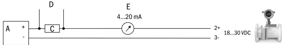
Fig. 15 Non-intrinsically safe installation, HART® output + external pressure sensor
