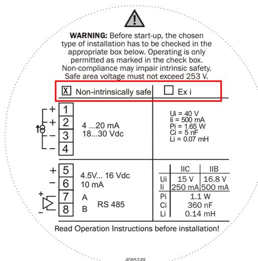
**WARNING:** Before start-up, the chosen type of installation has to be checked in the appropriate box below. Operating is only permitted as marked in the check box. Non-compliance may impair intrinsic safety. Safe area voltage must not exceed 253 V.
