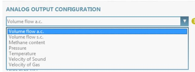
To adapt the FLOWSIC30 to the different application conditions, the analog output has to be configured. The adjustment of the analog output requires the change of various parameters.
