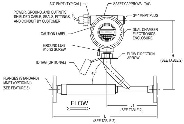
DIRECTLY ATTACHED ELECTRONICS ENCLOSURE (TA)
