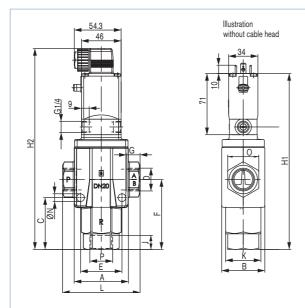
This dimensional drawing shows a valve in circuit function C with the port specifications P, R and A/B (manual override via port P). In circuit function D the manual override is located above the port A/B (pilot rotated 180° with respect to circuit function C). (Vacuum pump connected at port R, atmospheric pressure connected at port P.)
