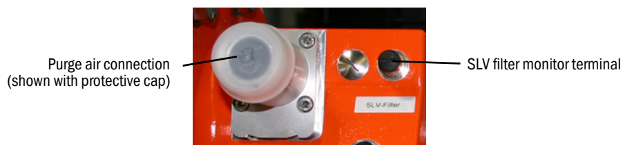
Fig. 16: Connection of the purge air supply
