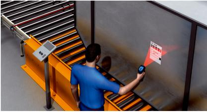
Container identification in factory automation: A wide range of code types can be reliably identified with only one device.
