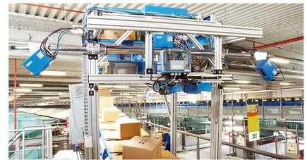
Easy PROFIBUS integration into large track-and-trace systems with the CDF600 fieldbus module.
