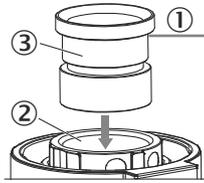
Figure 6: Screw in the S-mount lens
