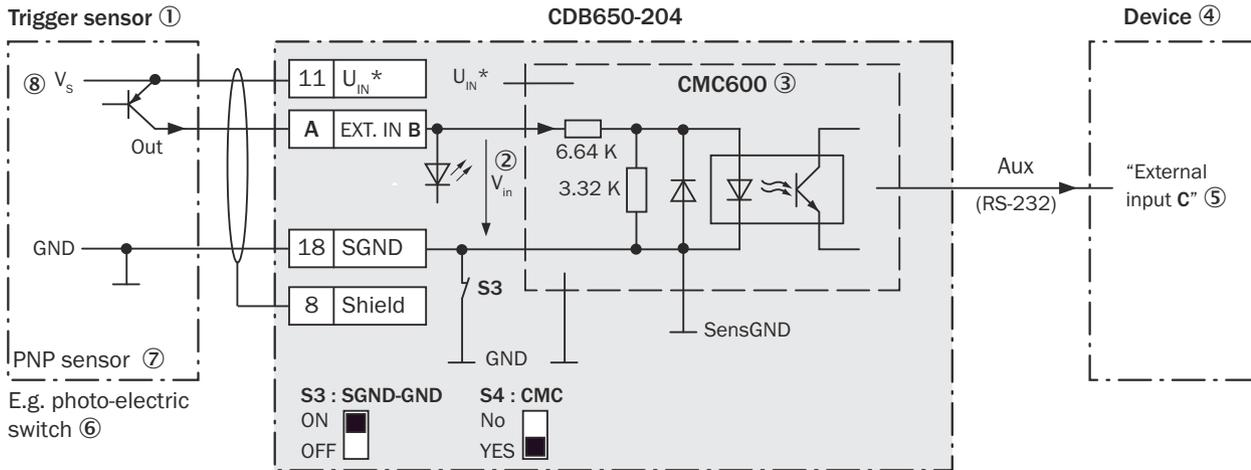
Figure 26: Trigger sensor supplied with power by connection module CDB650-204
