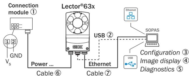
Figure 12: Connection block diagram
