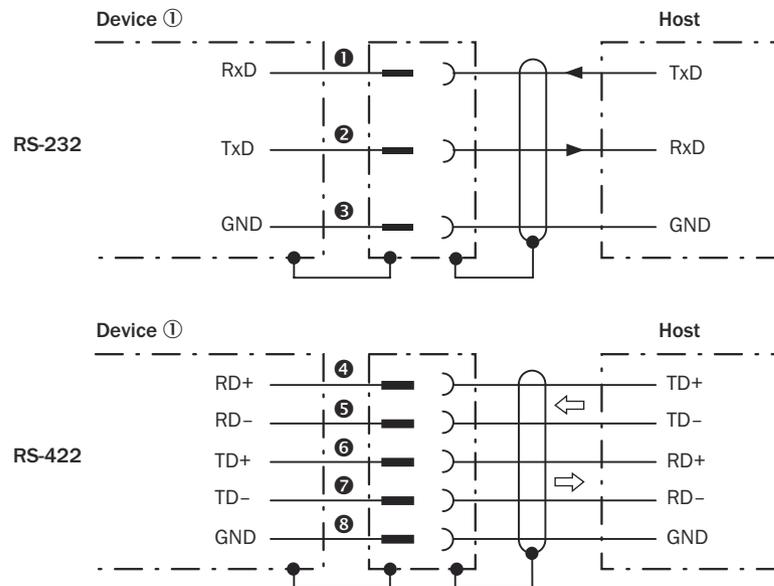
Figure 14: Wiring of the serial data interfaces RS-232 and RS-422
