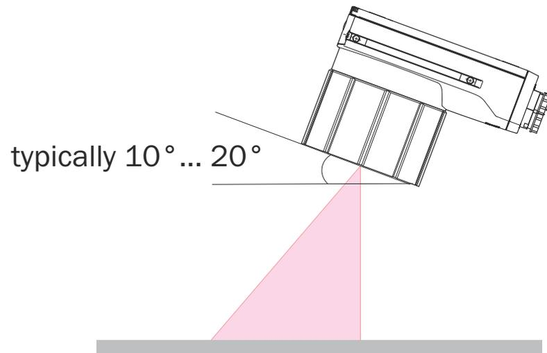
*Figure 7: Mounting angle to use, depending on the application*
