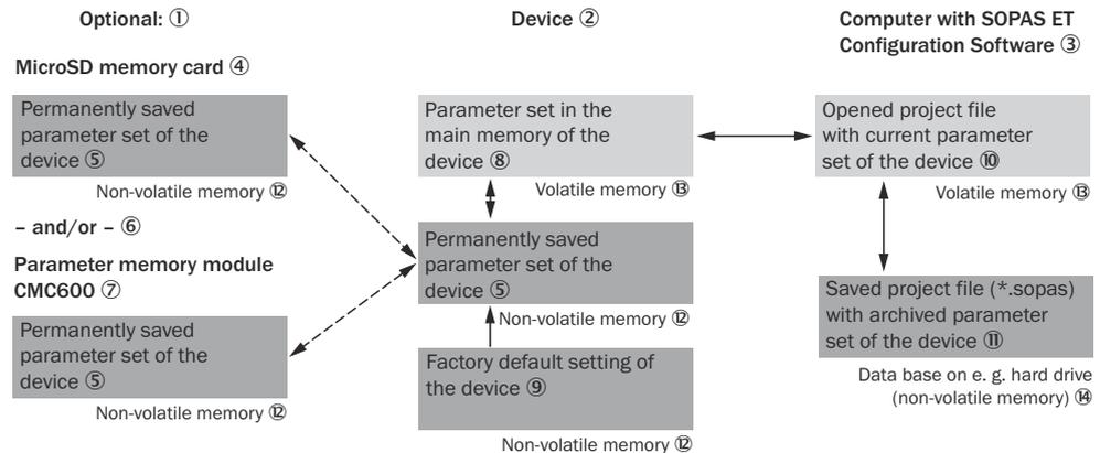
Figure 17: Configuration with SOPAS ET and saving the parameter set
