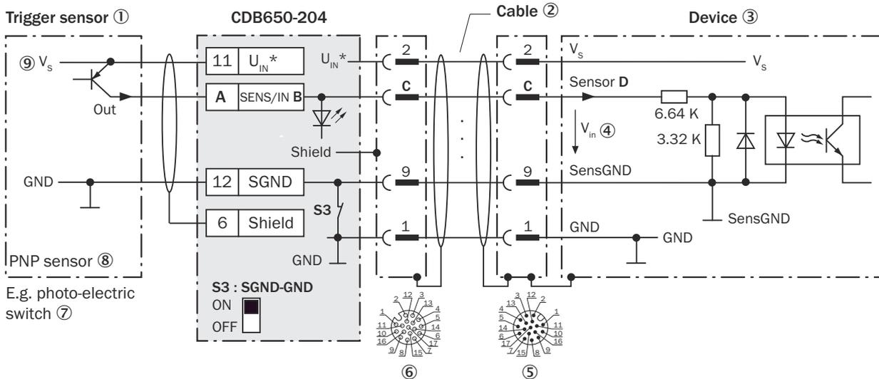
Figure 24: Trigger sensor supplied with power by connection module CDB650-204
