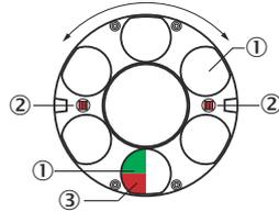
Figure 4: VI55I ring illumination unit (integrable illumination unit)
