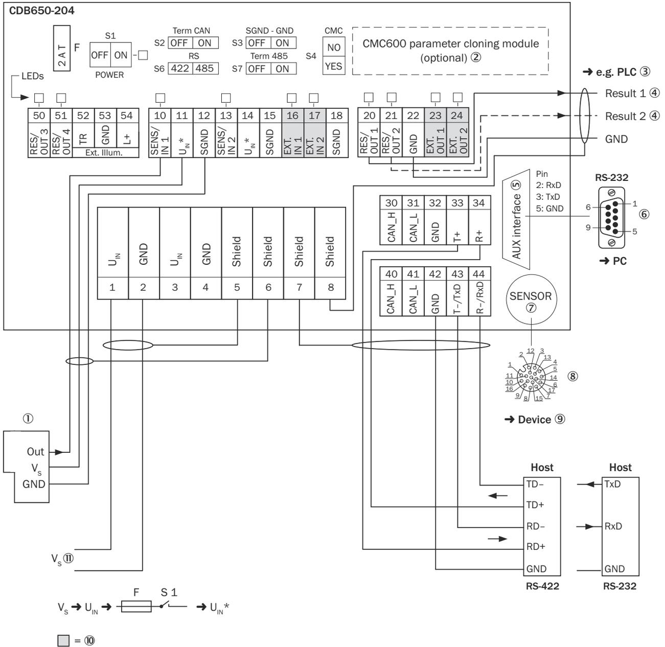
Figure 19: Connection of device and peripherals to the CDB650-204 connection module (overview)
