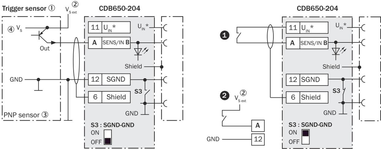
Figure 25: Left: Trigger sensor connected potential-free and supplied with power externally. Right: Alternatively switch, ❶ supplied with power by connection module CDB650-204 or ❷ connected potential-free and supplied with power externally. Switch setting S3 then as in left figure.
