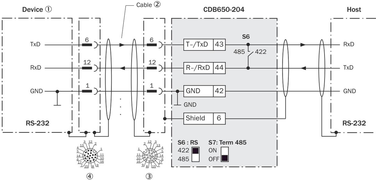
Figure 21: Wiring data interface RS-232 of the device in the connection module CDB650-204
