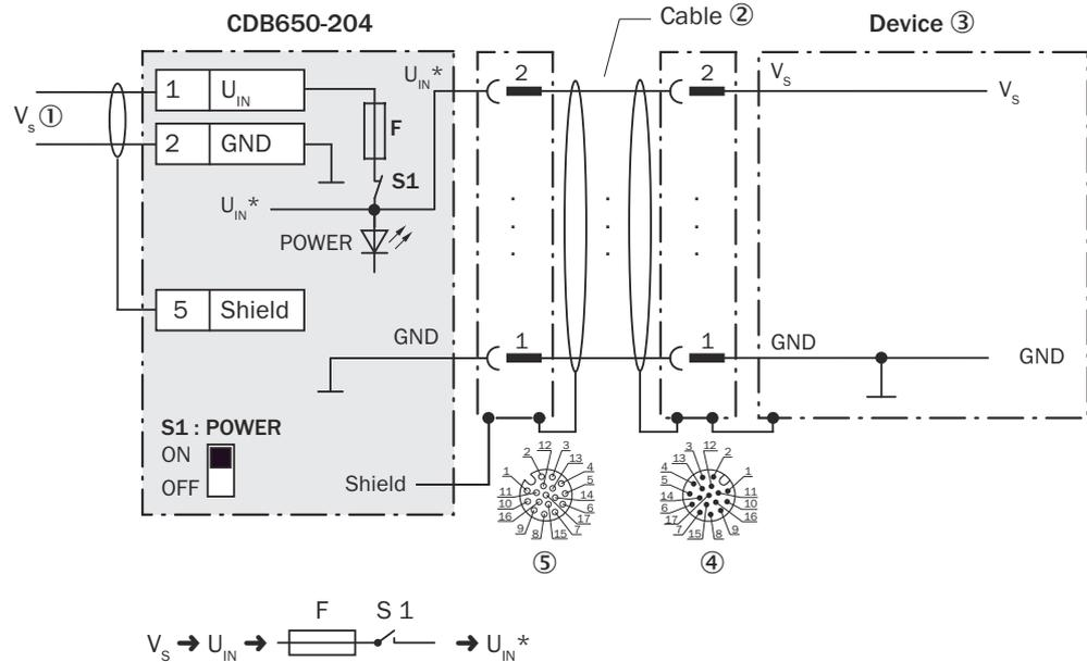
Figure 20: Connecting supply voltage for the device in CDB650-204 connection module
