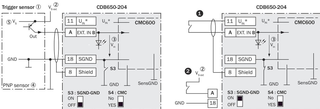
Figure 27: Left: Trigger sensor connected potential-free and supplied with power externally. Right: Alternatively switch, ① supplied with power by connection module CDB650-204 or ② connected potential-free and supplied with power externally. Switch setting S3 then as in left figure.
