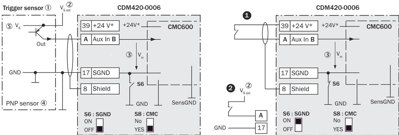
Figure 39: Left: Trigger sensor connected potential-free and supplied with power externally. Right: Alternatively switch, ① supplied with power by connection module CDM420-0006 or ② connected potential-free and supplied with power externally. Switch setting S3 then as in left figure.
