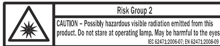
*Figure 1: Risk Group 2: CAUTION - Possibly hazardous optical radiation emitted from this product. Do not look into the lamp during operation. This could damage your eyes. IEC 62471:2006-07; EN62471:2008-09*
