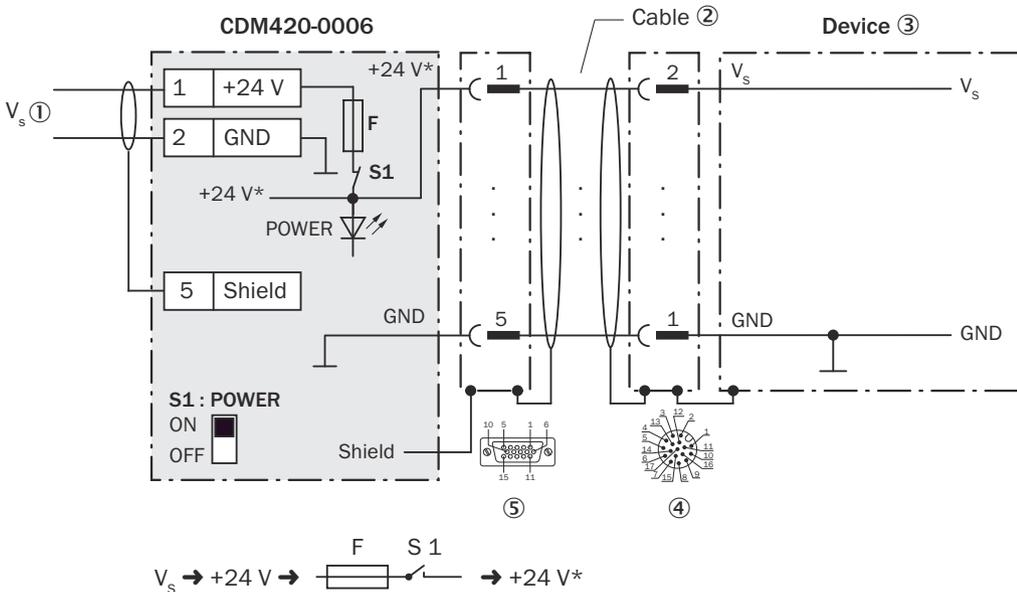
Figure 32: Connecting supply voltage for the device in CDM420-0006 connection module
