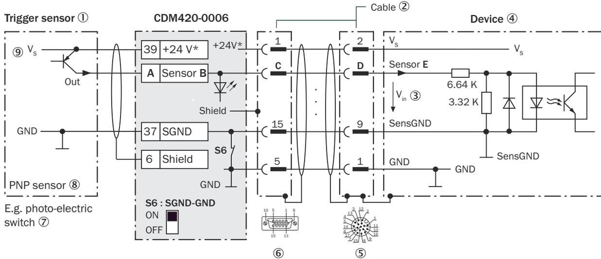
Figure 36: Trigger sensor supplied with power by connection module CDM420-0006
