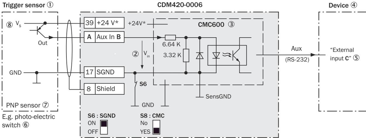
Figure 38: Trigger sensor supplied with power by connection module CDM420-0006
