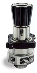
TESCOM 26-1600 Series highly accurate, diaphragm sensed pressure reducing regulator offers adjustable venting standard. Panel mounting, integrated 40 micron filter and low handknob torque ensure a robust and adaptable design with many modifications available.
