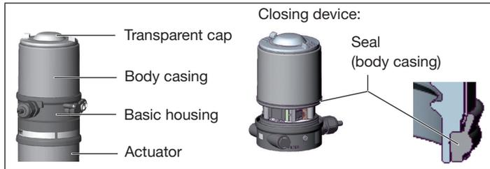
Fig. 33: Opening or closing the device
