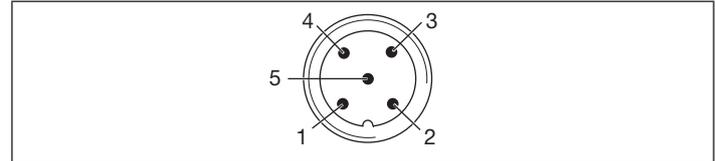
Fig. 22: Pin assignment
