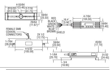
The MODEL UFM Compact Ultrasonic Flowmeters is an economical, clamp-on, ultrasonic flowmeter. The Model UFM implements the transit-time difference to measure flow rates in pipes and can measure velocity and flow in pipes with outside diameters ranging from 0.98 to 4.62" (24.89 to 117.35 mm). This model comes with a volume pulse and 4 to 20 mA flow rate output.
