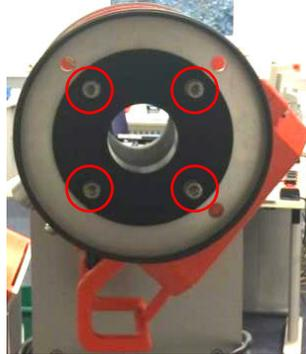
2. Remove the black insert and set aside (store in the shipping box of the protection window for further use)..
