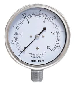
Low Pressure Gauges from Marsh Instruments incorporate a diaphragm element allowing for accurate low-pressure readings in support of a variety of applications, with ASME Grade A 2/1/2% accuracy for ranges above 30" of water. Available ranges include vacuum and pressure in inches of water, ounces per square inch, kilopascals, and millimeters of mercury.
