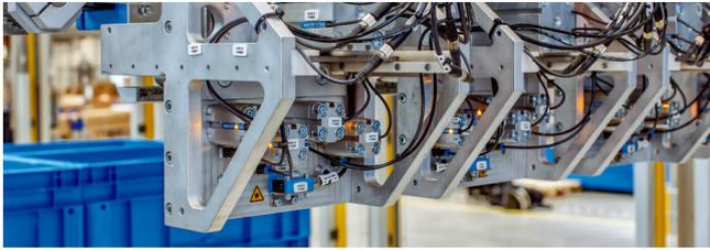
The MPS-G delivers data on possible wear or if the cylinders are not optimally adjusted
