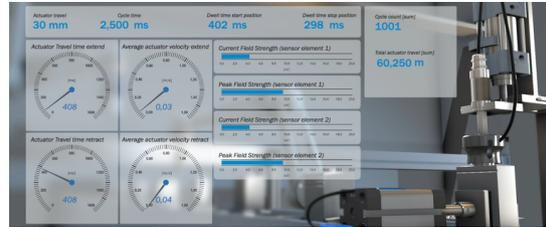
Traversing speed, cylinder travel, dwell time in the end positions and magnetic field strength are only some examples of diagnostic data the MPS-G generates
