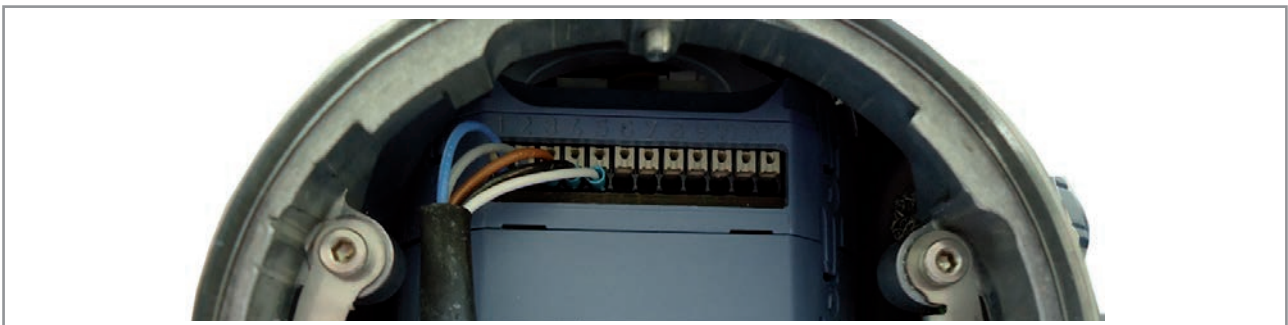
Figure 25: Wiring ex works of the 12 push-in terminal strip
