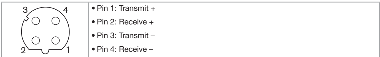
Figure 37: Pin assignment of the 4-pin M12 female connector
