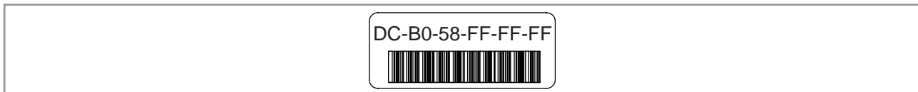
Figure 9: Marking with the MAC address of the device (example)
