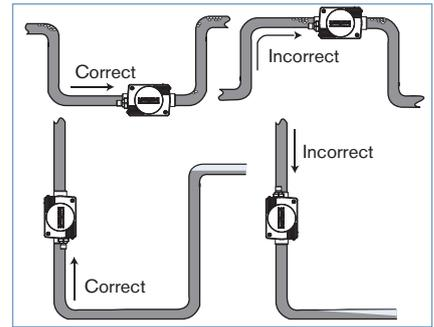
Minimum upstream and downstream distances are not necessary.
