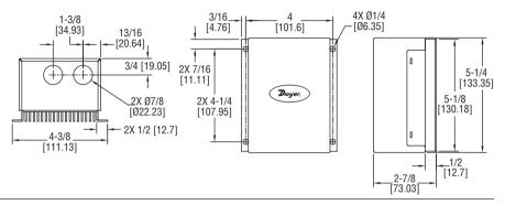
The MODEL FC-1000 Electronic Fan Speed Control provides precise speed modulation of small AC motors. Popular 0-10 VDC input works with most process controllers, eliminating the need for more expensive dampers, damper actuators, and linkages while improving overall energy efficiency of the system. This inexpensive unit enables variable control ventilation fans, condenser fans, and interfacing with VAV box controllers.
